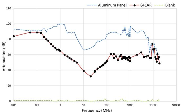
Test performed with a 2 coat thickness.
