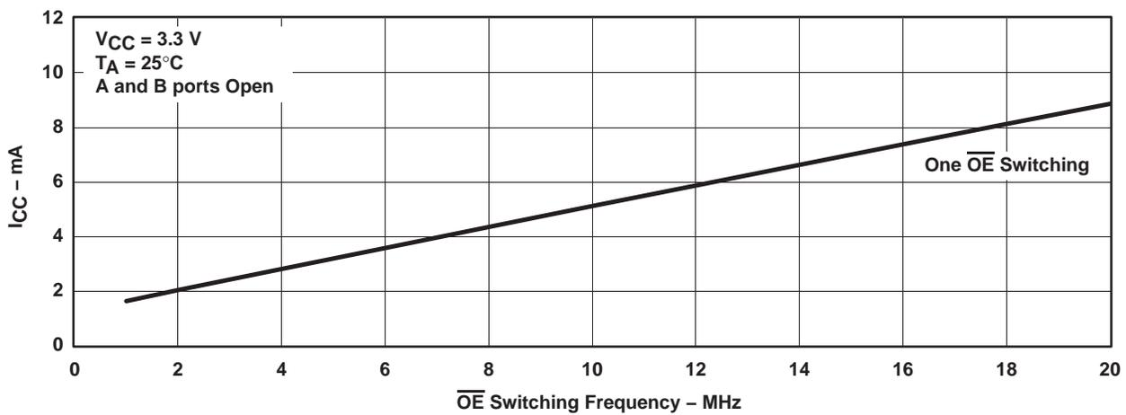
Figure 2. Typical  $I_{CC}$  vs  $\overline{OE}$  Switching Frequency
