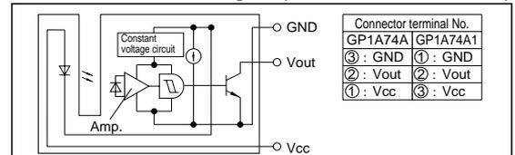
\* GP1A74A and GP1A74A1 are different in the terminal marking number of connectors from each other due to use of connectors of different manufacturers.
