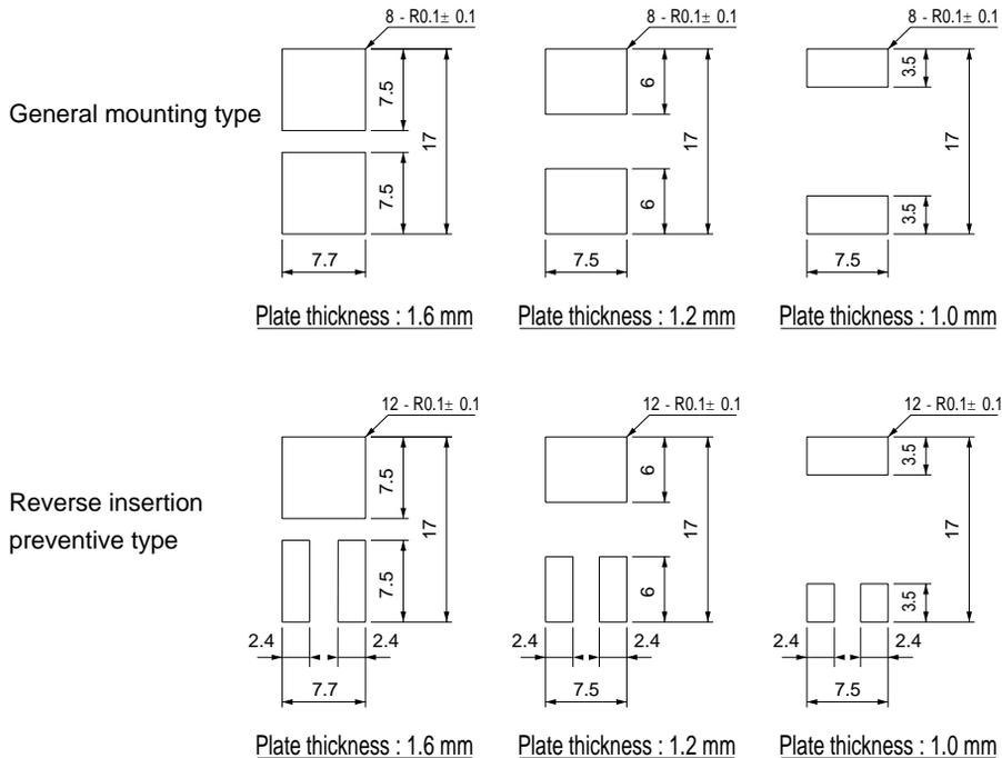
1. It is recommended to mark the shear droop surface (punch side) of the mounting plate (metal plate) with "GP1A74A" or "GP1A74A1".
