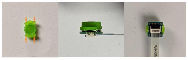
Figure 4. UV Cured Glue Applied to Horn
