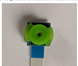
Figure 1. MOD\_CH101-03-01 module with AH-10133-045045MR horn
