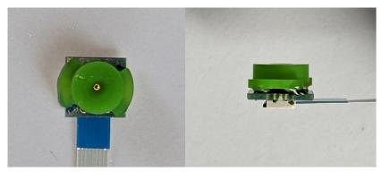
Figure 5. Physical Alignment of Horn
