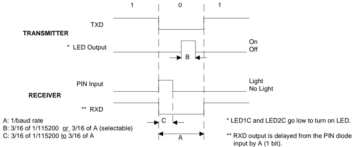
**Figure 2. Infra Red Data Format Mode 1 (IRDA/HPSIR)**
