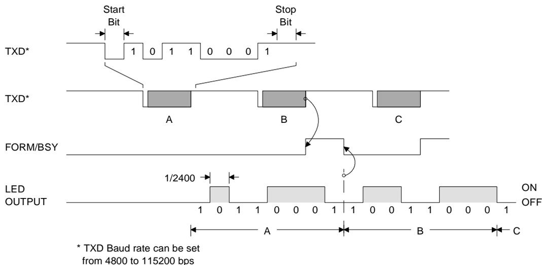
**Figure 5. Mode 3 (TV Remote) Transmit Data Format**
