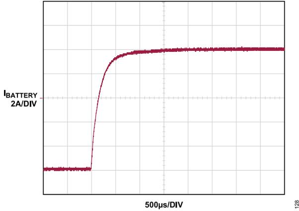
Figure 28. 10 A Step Charge Example in Synchronous Mode, 10 A System Demonstration with 10 AH LiFePO<sub>4</sub> (*I<sub>BATTERY</sub>* Is the Battery Current)
