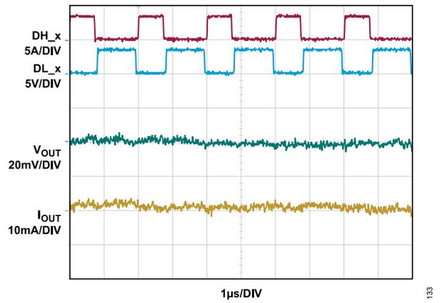
Figure 33. Typical 10 A CC Ripple at 500 kHz, 10 A System Demonstration with 10 AH LiFePO<sub>4</sub>
