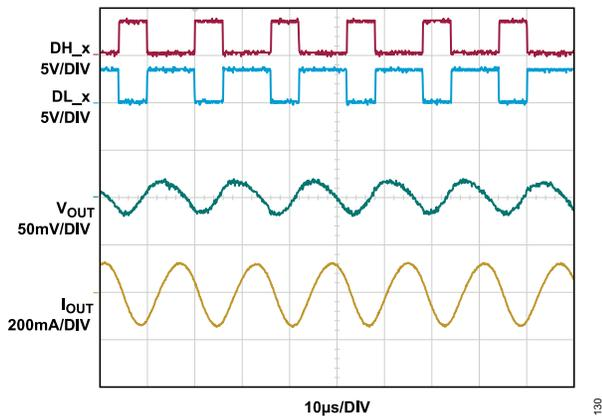
Figure 30. Typical 10 A CC Ripple at 62.5 kHz, 10 A System Demonstration with 10 AH LiFePO<sub>4</sub> (*I<sub>OUT</sub>* Is the Output Current)
