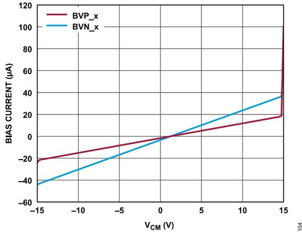
Figure 4. BVx\_x Bias Current vs. Common-Mode Voltage ( $V_{CM}$ )
