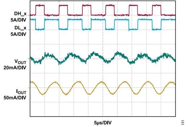
Figure 31. Typical 10 A CC Ripple at 125 kHz, 10 A System Demonstration with 10 AH LiFePO<sub>4</sub>
