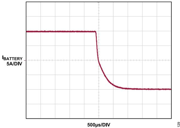
Figure 29. Charge to Discharge Transition Example in Synchronous Mode, 10 A System Demonstration with 10 AH LiFePO<sub>4</sub>
