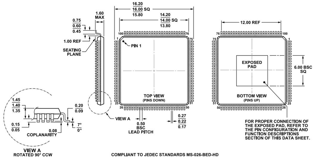
Figure 44. 100-Lead Low Profile Quad Flat Package, Exposed Pad [LQFP]
