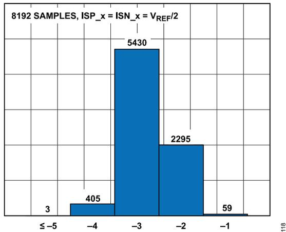
Figure 18. ISx\_x Channel Histogram Codes at Code Center
