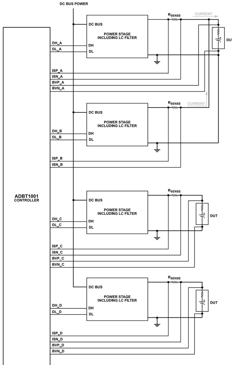
Figure 41. Two Parallel—Two Independent Channels Use Case
