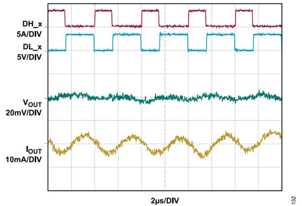
Figure 32. Typical 10 A CC Ripple at 250 kHz, 10 A System Demonstration with 10 AH LiFePO<sub>4</sub>
