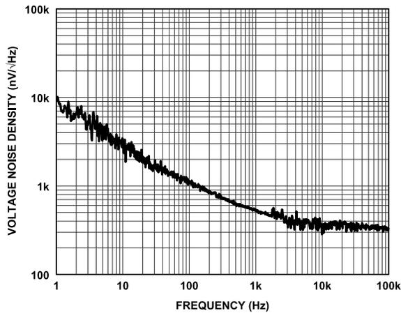
Figure 24. CVS\_x Voltage Noise Density vs. Frequency, G = 0.5
