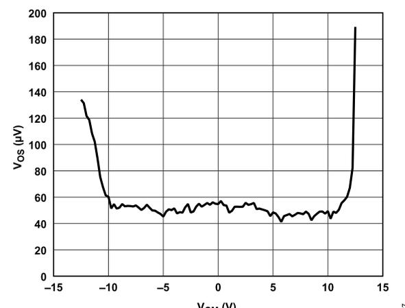
Figure 27. ISx\_x Amplifier Offset Voltage ( $V_{OS}$ ) vs.  $V_{CM}$
