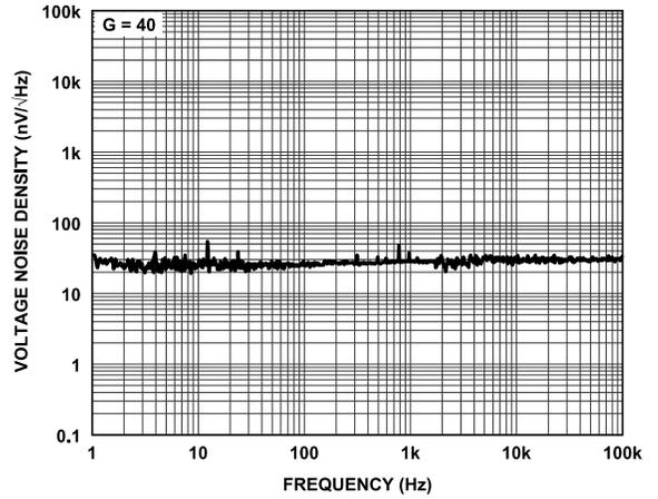
Figure 25. ISx\_x Voltage Noise Density vs. Frequency, G = 40
