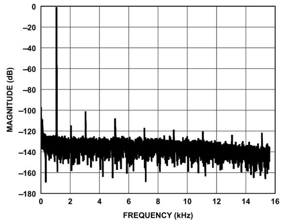
Figure 15. BVx\_x Amplifier Fast Fourier Transform (FFT)
