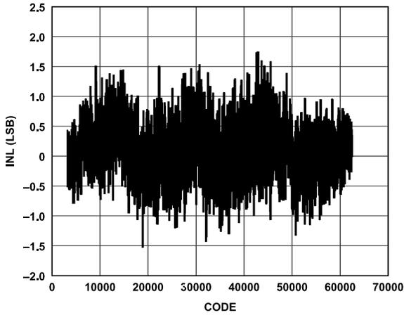
Figure 22. ISx\_x Amplifier Full System INL
