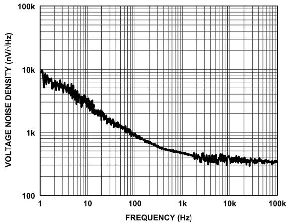
Figure 23. BVx\_x Voltage Noise Density vs. Frequency, G = 0.5
