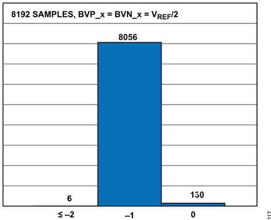
Figure 17. BVx\_x Channel Histogram Codes at Code Center
