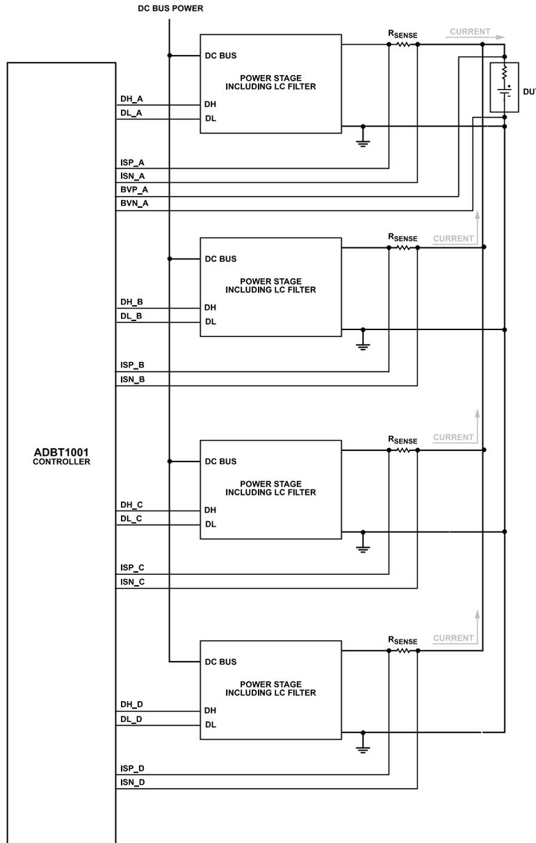
Figure 42. Four Channels in Parallel Use Case
