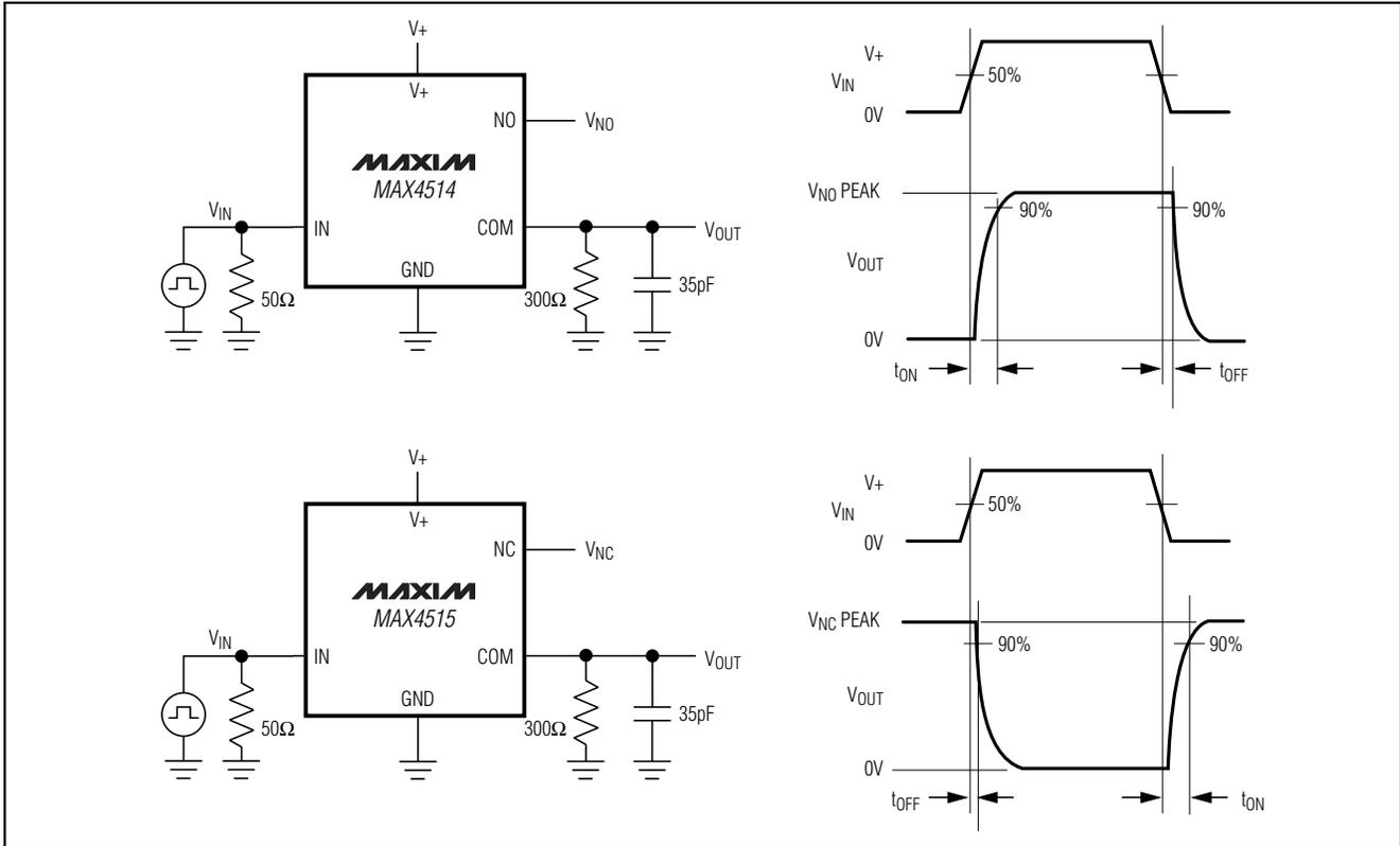
Figure 2. Switching Times
