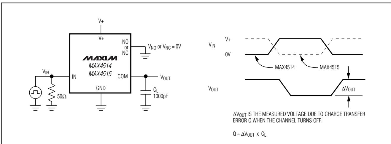
Figure 1. Charge Injection
