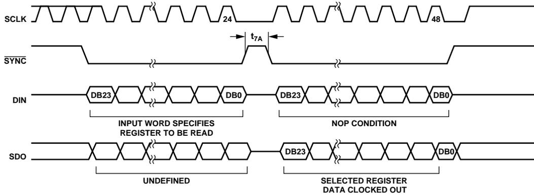
Figure 4. Serial Interface Timing Diagram (Data Readback Mode)
