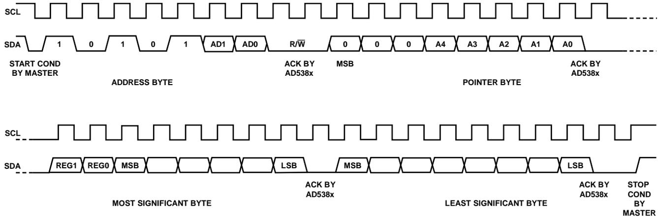
Figure 30. 4-Byte AD5382, I<sup>2</sup>C Write Operation
