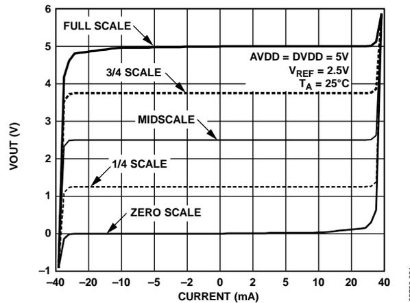
Figure 20. AD5382-5 Output Amplifier Source and Sink Capability
