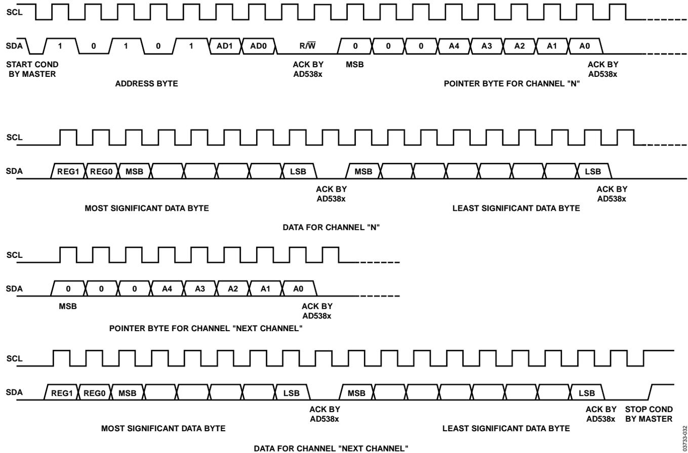
Figure 31. 3-Byte AD5382, I<sup>2</sup>C Write Operation
