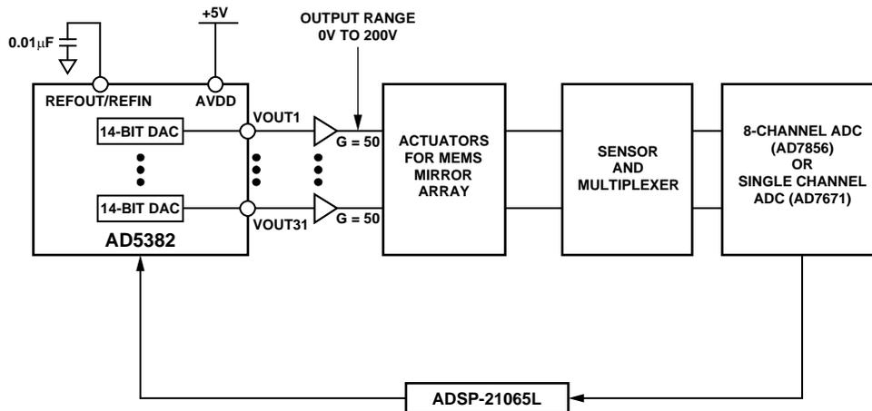
Figure 46. AD5382 in a MEMS Based Optical Switch
