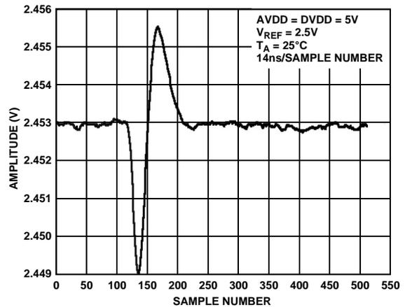
Figure 24. Adjacent Channel DAC-to-DAC Crosstalk
