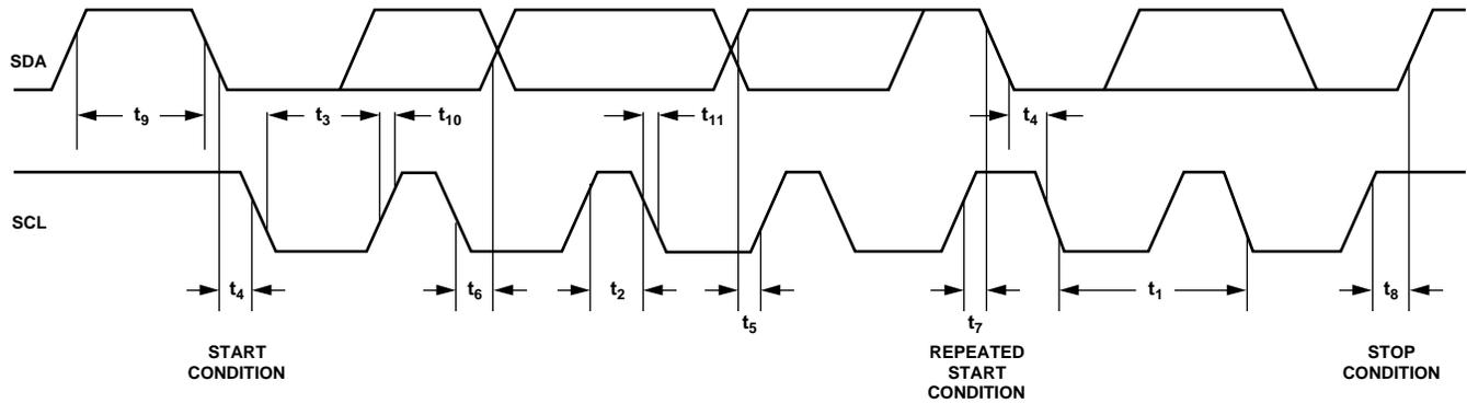
Figure 6. I<sup>2</sup>C-Compatible Serial Interface Timing Diagram
