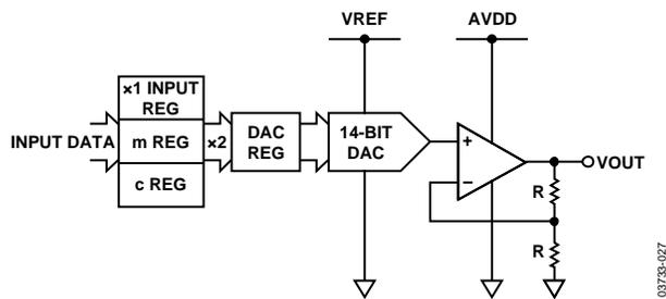
Figure 26. Single-Channel Architecture
