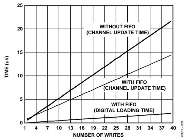
Figure 28. Channel Update Rate (FIFO vs. Non-FIFO)
