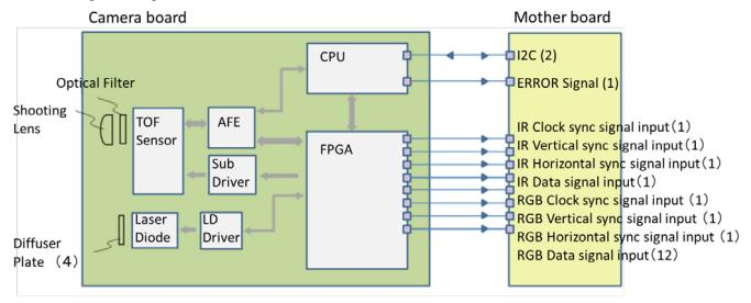
The FPGA outputs the RGB Data and the IR Data.
