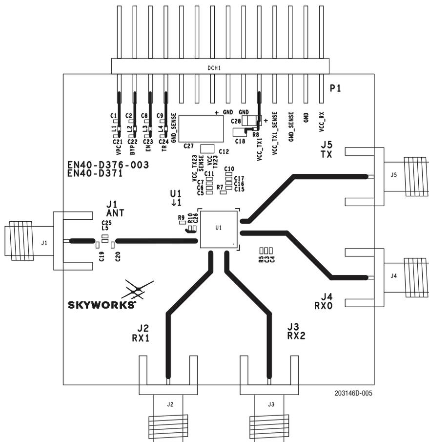
Figure 6. SKY65366-21 Evaluation Board Assembly Diagram
