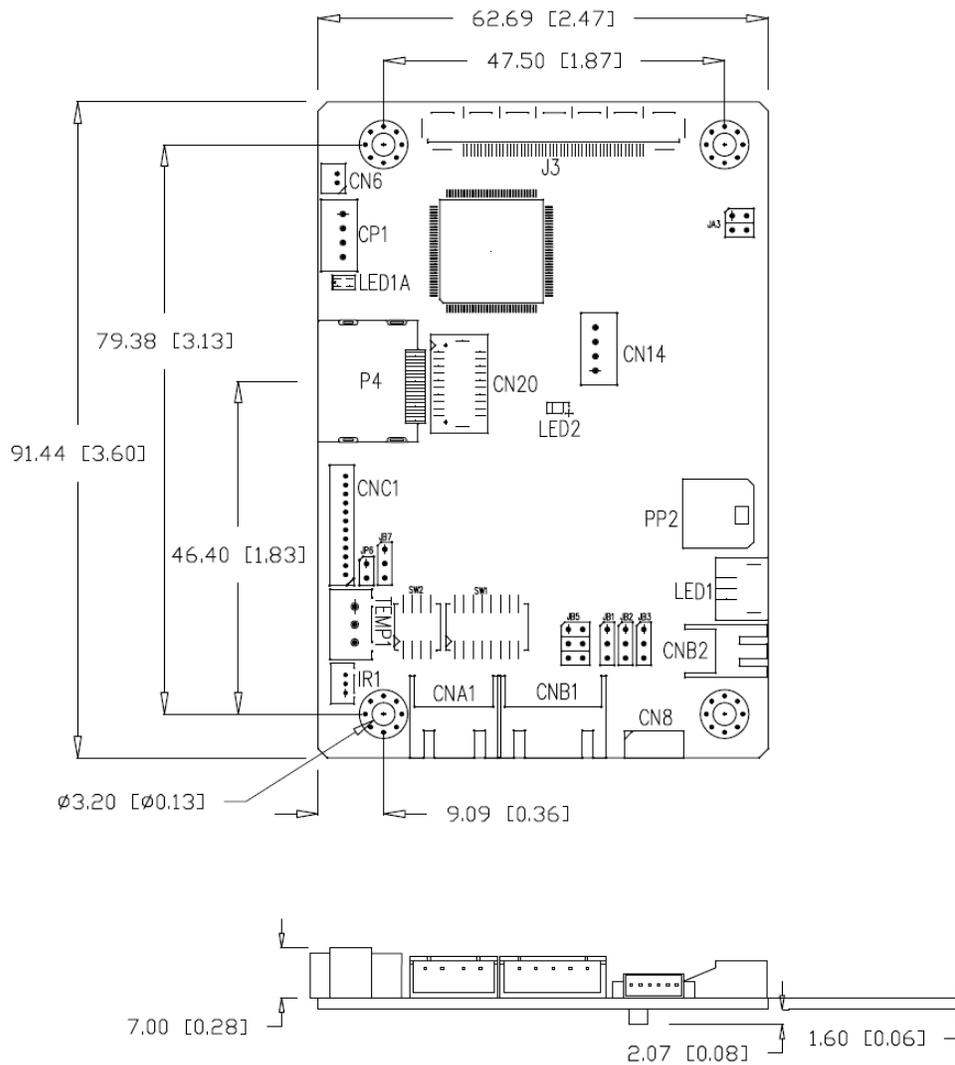
The maximum thickness of the controller is 10.67mm (measured from bottom of PCB to top of components, including any underside components & leads). We recommend clearances of:
