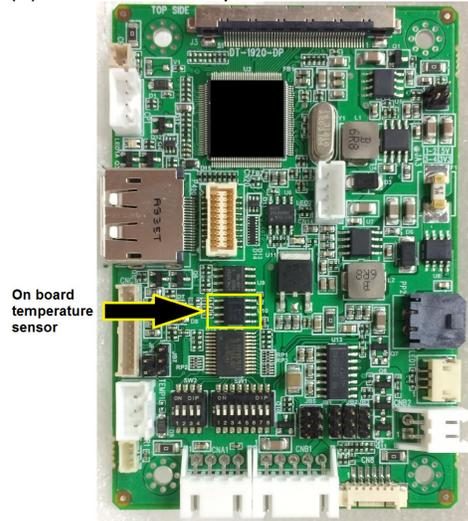
It provides three ways to read the on-board temperature value :
