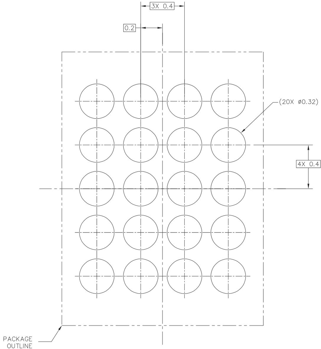
PCB DESIGN GUIDELINES – SOLDER MASK OPENING PATTERN
