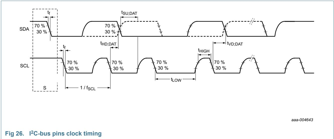
Fig 26. I<sup>2</sup>C-bus pins clock timing
