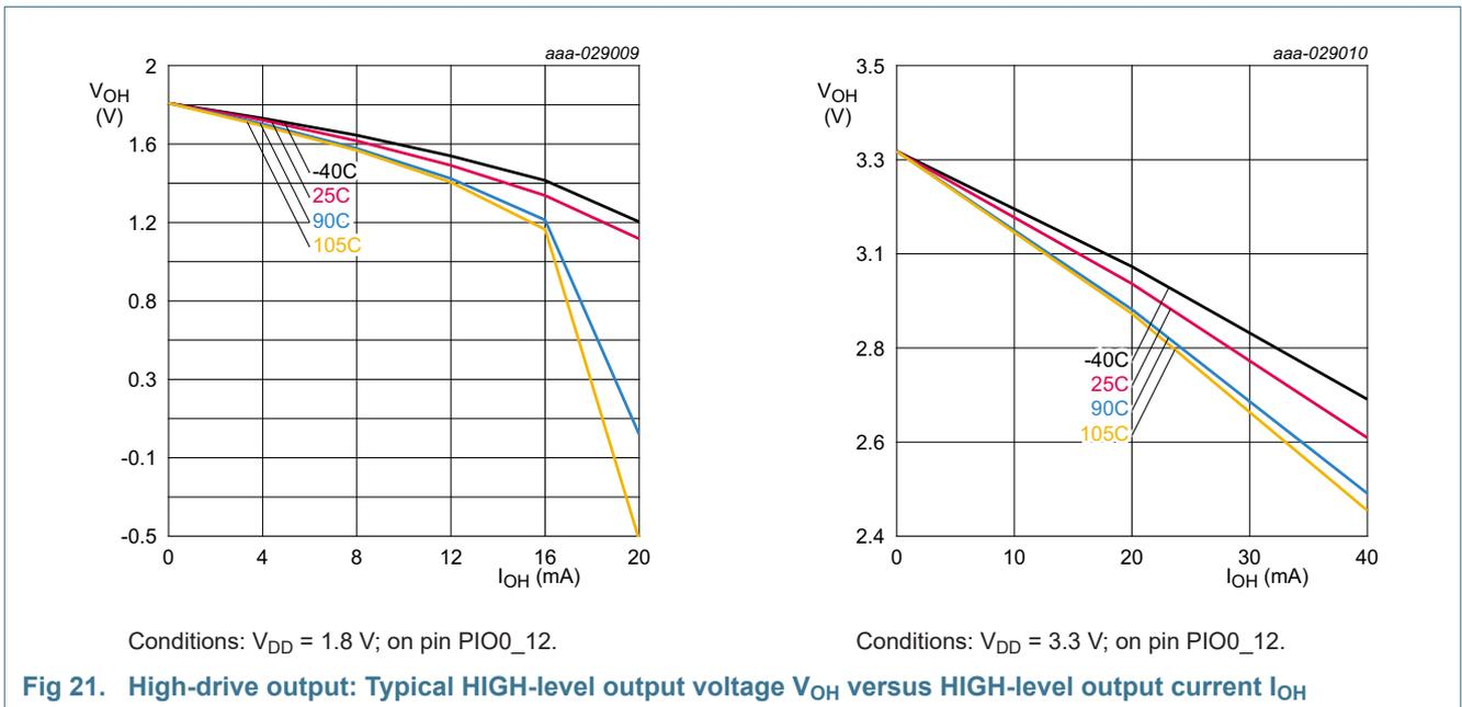
Fig 21. High-drive output: Typical HIGH-level output voltage  $V_{OH}$  versus HIGH-level output current  $I_{OH}$
