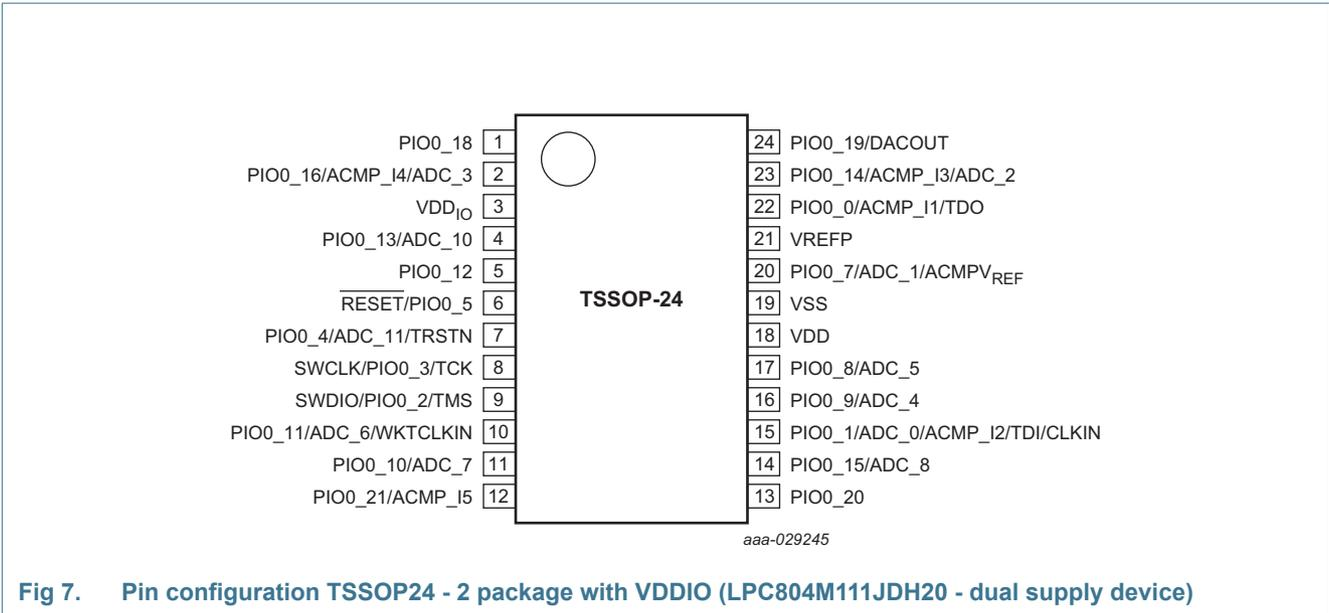
Fig 7. Pin configuration TSSOP24 - 2 package with VDDIO (LPC804M111JDH20 - dual supply device)
