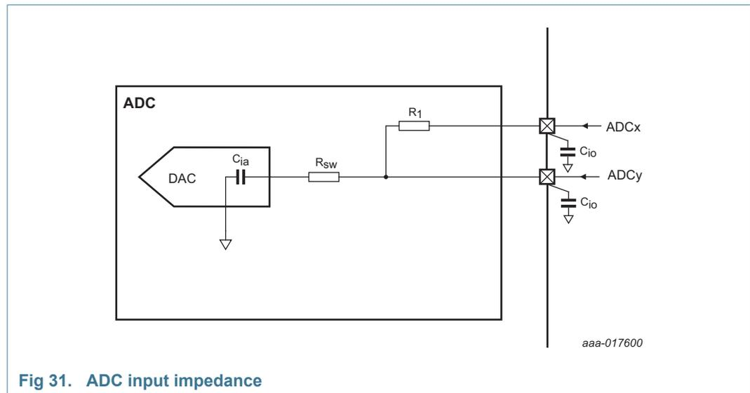
Fig 31. ADC input impedance
