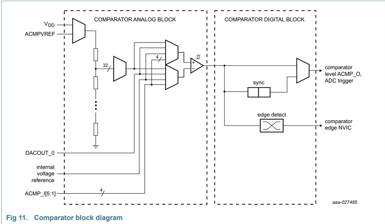
Fig 11. Comparator block diagram
