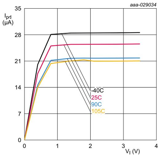
Conditions:  $V_{DD} = 1.8$  V; standard port pins.
