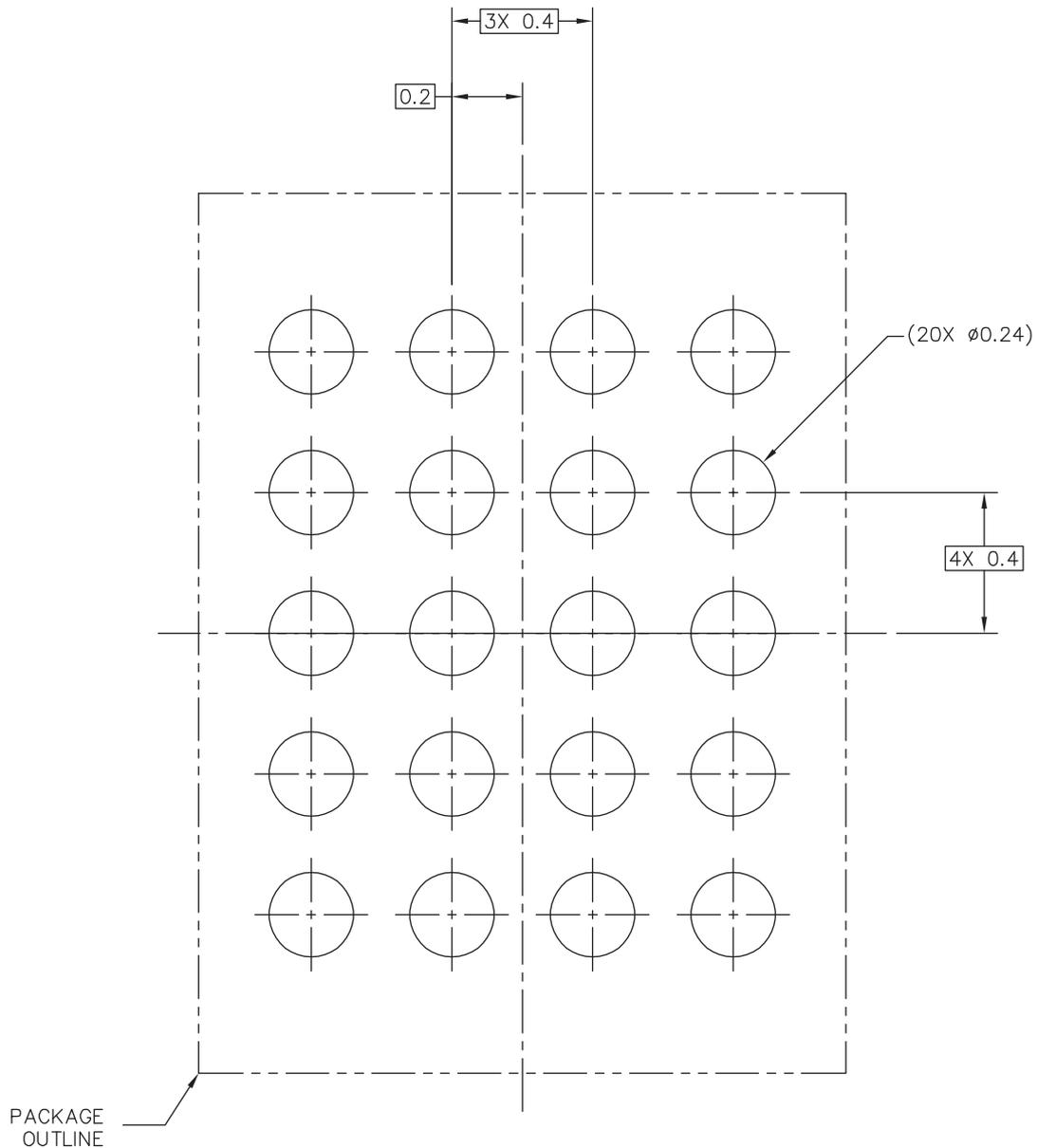
PCB DESIGN GUIDELINES – I/O PADS AND SOLDERABLE AREA
