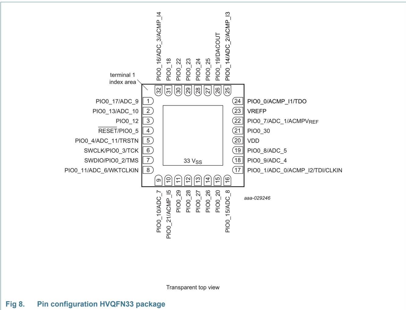
Fig 8. Pin configuration HVQFN33 package
