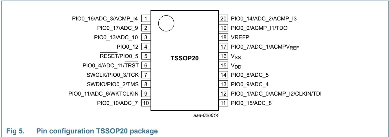
Fig 5. Pin configuration TSSOP20 package
