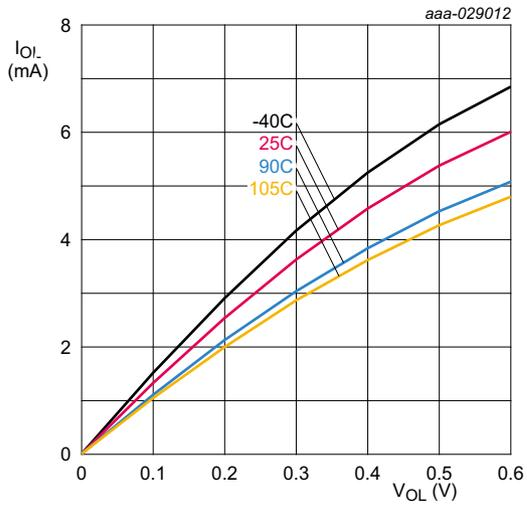
Conditions:  $V_{DD} = 1.8$  V; standard port pins and high-drive pin PIO0\_12.
