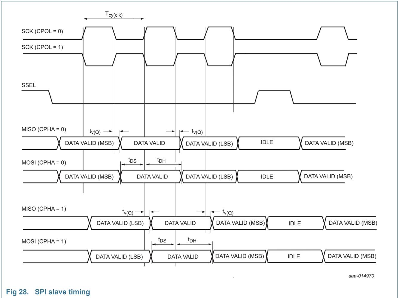
Fig 28. SPI slave timing
