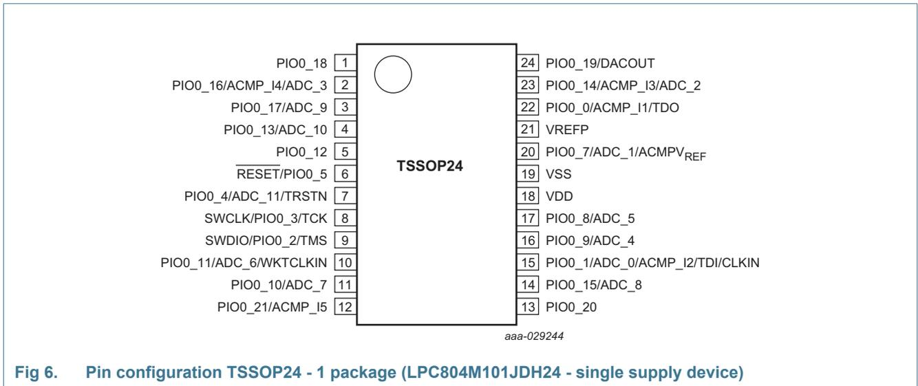
Fig 6. Pin configuration TSSOP24 - 1 package (LPC804M101JDH24 - single supply device)
