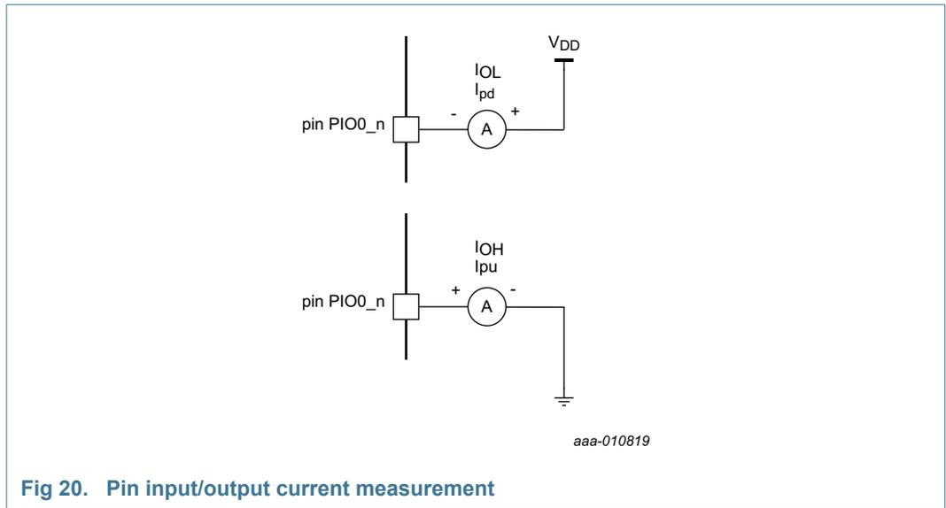
Fig 20. Pin input/output current measurement
