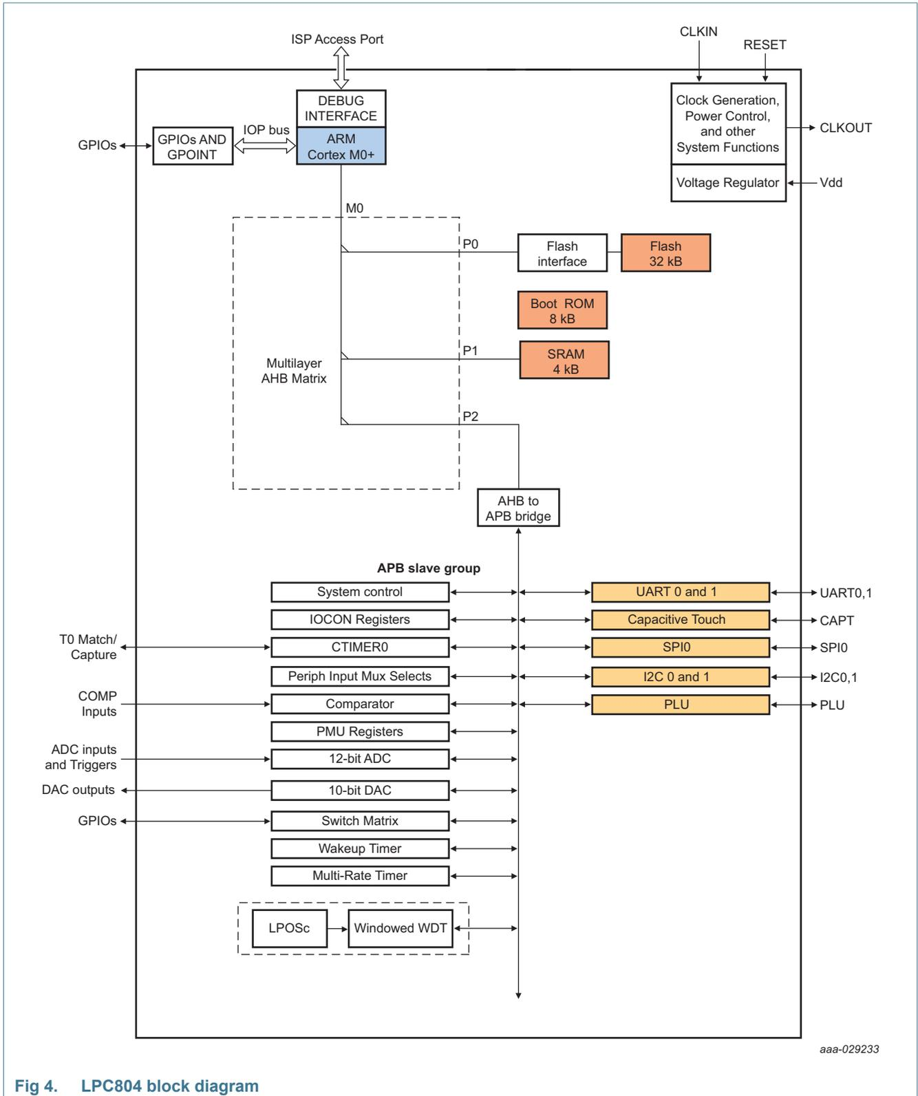
Fig 4. LPC804 block diagram
