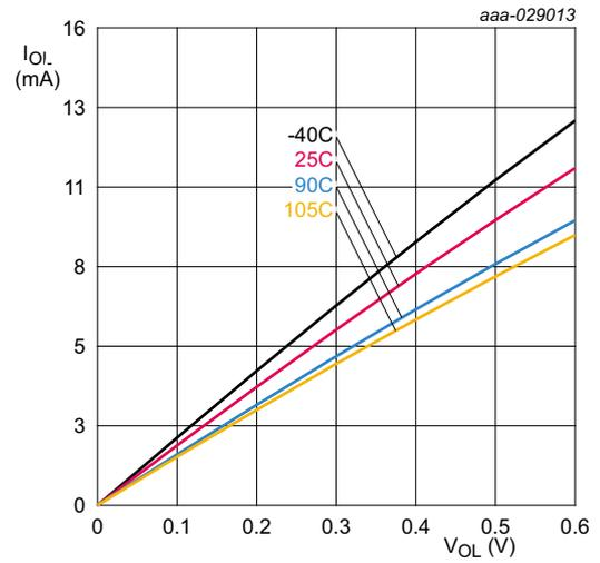
Conditions:  $V_{DD} = 3.3$  V; standard port pins and high-drive pin PIO0\_12.
