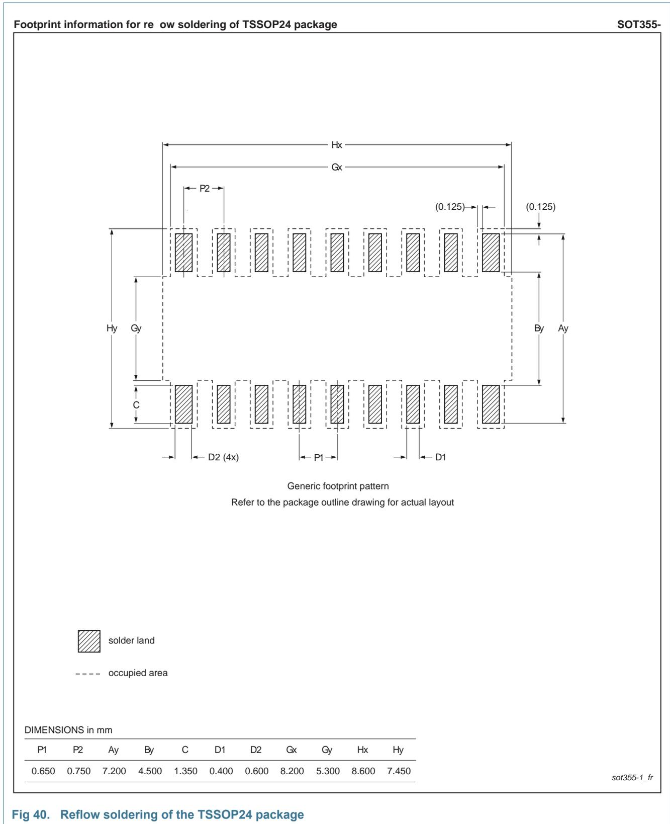
**Fig 40. Reflow soldering of the TSSOP24 package**
