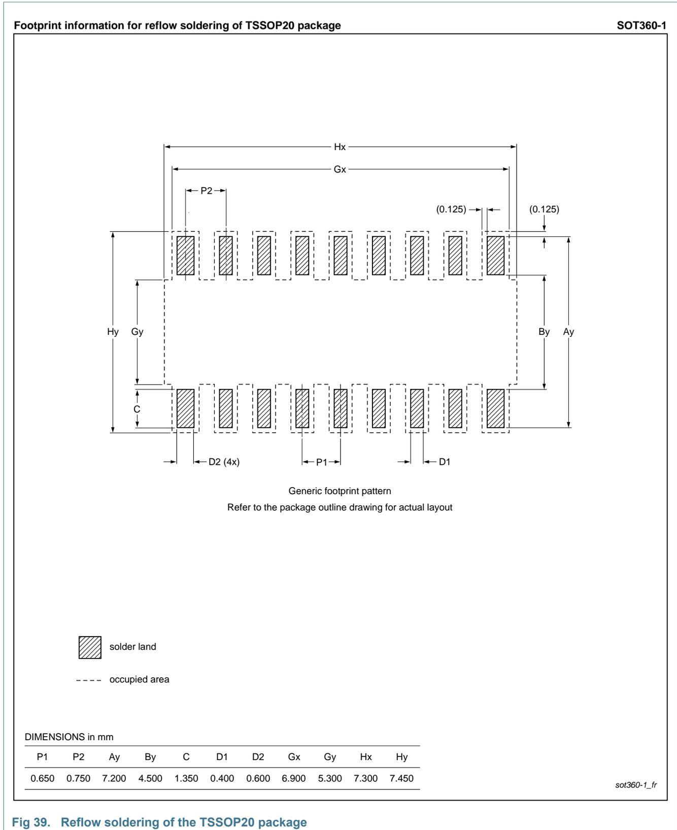
**Fig 39. Reflow soldering of the TSSOP20 package**
