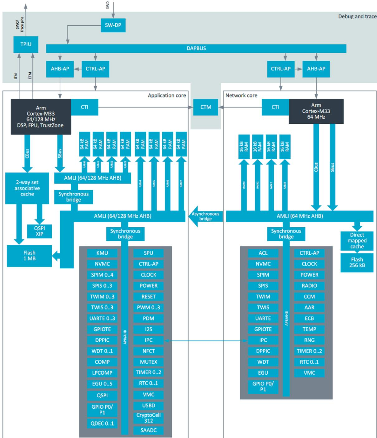
nRF5340 is a wireless ultra-low power multiple core System on Chip (SoC) integrating two fully programmable Arm Cortex M33 processors, advanced security features, a range of peripherals, and a multiprotocol 2.4 GHz
