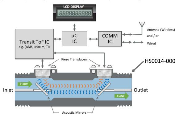
The following evaluation kits from ams, Maxim, and TI that are sold on Digikey can be used to directly connect to the HS0014-000 and begin evaluation of both the flow tube and the chosen transit ToF measurement IC:
