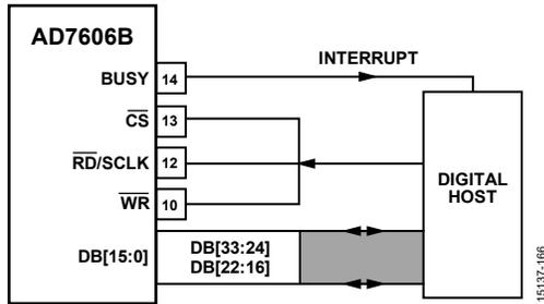
Figure 63. AD7606B Interface Diagram—One AD7606B Using the Parallel Bus, with CS and RD Shorted Together
