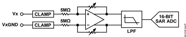
Figure 42. Analog Input Circuitry for Each Channel
