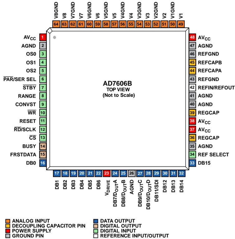
Figure 8. Pin Configuration
