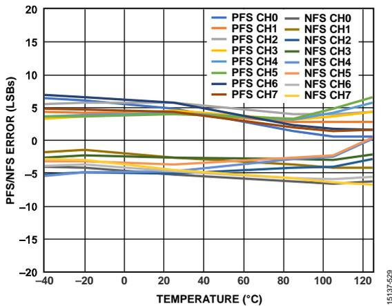
Figure 29. PFS/NFS Error vs. Temperature, ±2.5 V Range
