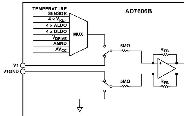
Figure 83. Diagnostic Multiplexer (Channel 1 Shown as an Example)
