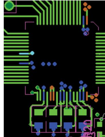
Figure 89. Top Layer Decoupling REF<sub>IN</sub>/REF<sub>OUT</sub>, REFCAPA, REFCAPB, and REGCAP Pins
