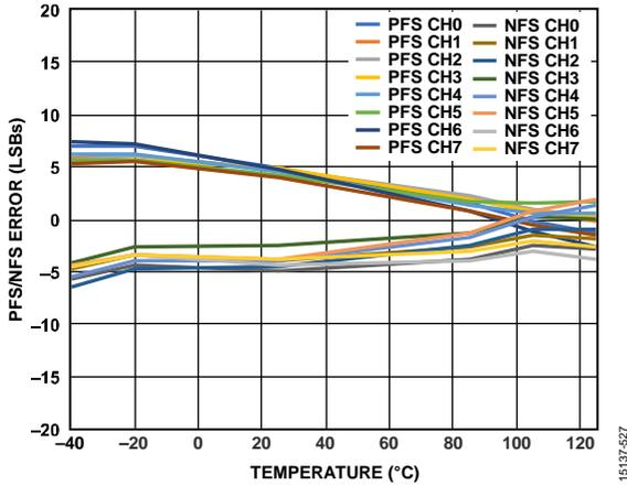
Figure 27. PFS/NFS Error vs. Temperature, ±10 V Range
