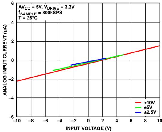
Figure 39. Analog Input Current vs. Input Voltage
