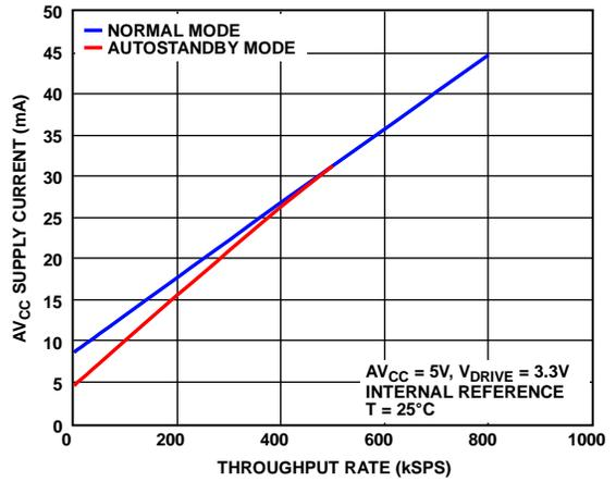
Figure 41. AVCC Supply Current vs. Throughput Rate
