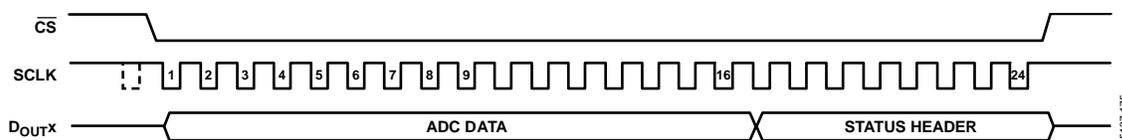
Figure 73. Serial Interface, ADC Read Mode, Status On
