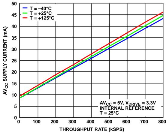
Figure 40. AVCC Supply Current vs. Throughput Rate
