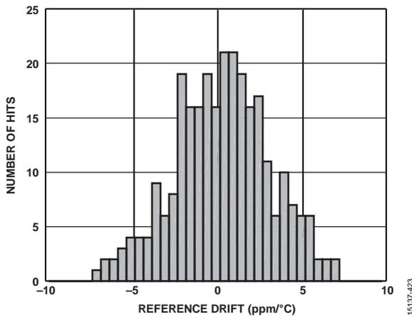
Figure 23. Reference Drift Histogram
