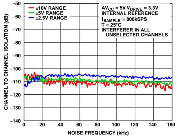
Figure 31. Channel to Channel Isolation vs. Noise Frequency
