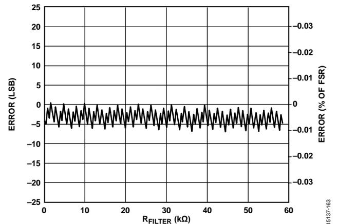
Figure 59. System Error with Gain Calibration Enabled
