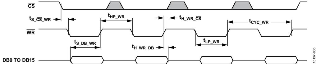
Figure 5. Parallel Mode Write Operation Timing Diagram
