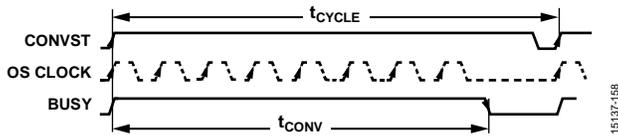
Figure 53. Oversampling by 8 Example, Oversampling Padding Enabled
