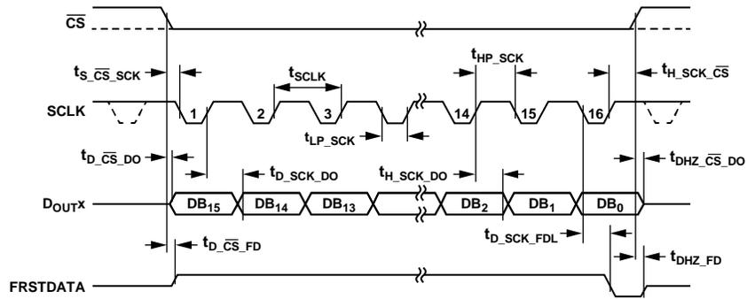
Figure 6. Serial Timing Diagram, ADC Read Mode (Channel 1)
