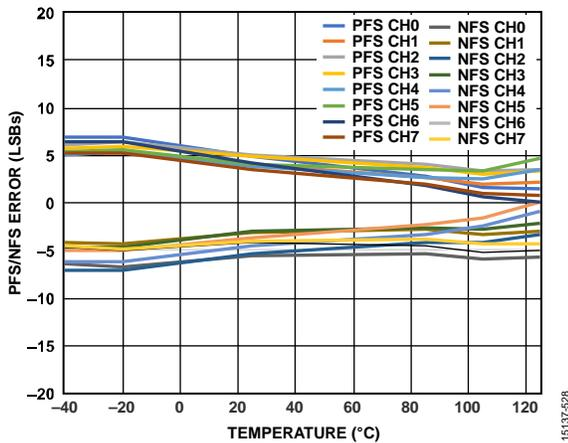
Figure 28. PFS/NFS Error vs. Temperature, ±5 V Range
