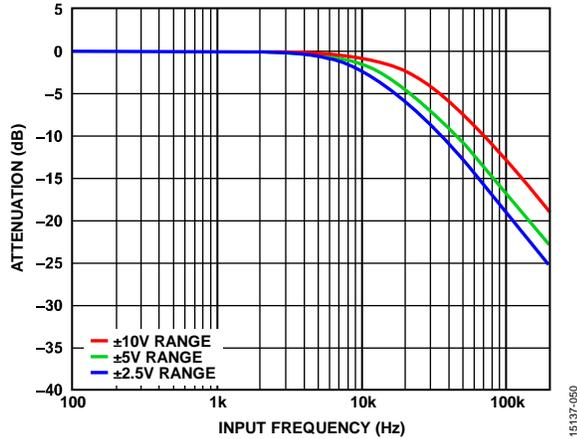
Figure 45. Analog Antialiasing Filter Frequency Response
