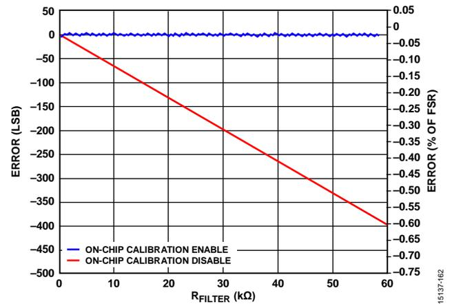
Figure 58. System Gain Calibration with and Without Calibration
