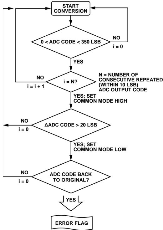
Figure 62. Automatic Analog Input Open Circuit Detect Flowchart
