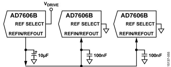
Figure 50. Internal Reference Driving Multiple AD7606B REFIN/REFOUT Pins
