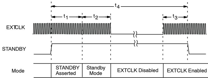
NOTE: In hard standby mode, EXTCLK is automatically gated off, and the two-wire serial interface is not active.
