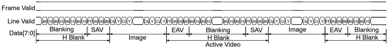
**Figure 20. BT656 Image Data with Odd SAV/EAV Codes**
