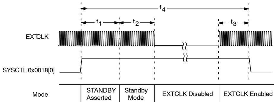
**Figure 4. Soft Standby Mode Operation**
