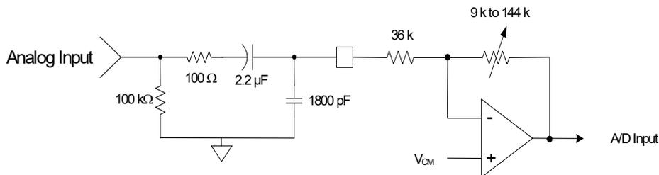
Figure 12. 1 V<sub>RMS</sub> Input Circuit with RF Filtering
