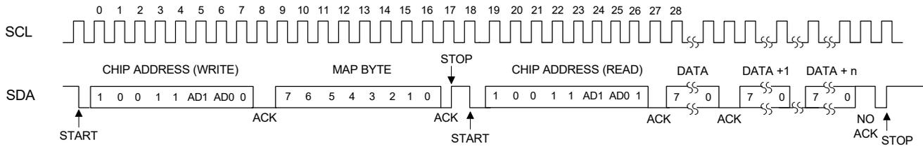
**Figure 16. Control Port Timing, I<sup>2</sup>C Read**
