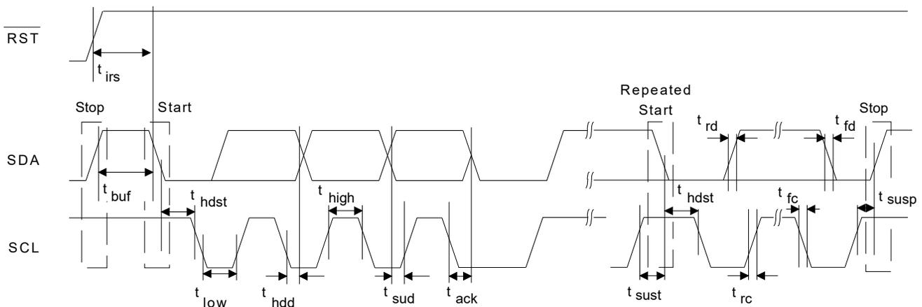
Figure 5. Control Port Timing - I<sup>2</sup>C Format
