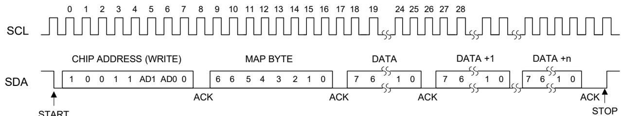
Figure 15. Control Port Timing, I<sup>2</sup>C Write
