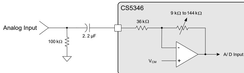
Figure 11. 1 V<sub>RMS</sub> Input Circuit
