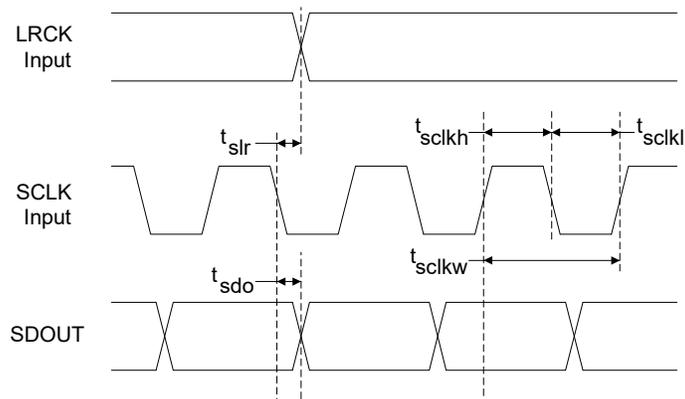
**Figure 1. Master Mode Serial Audio Port Timing**
