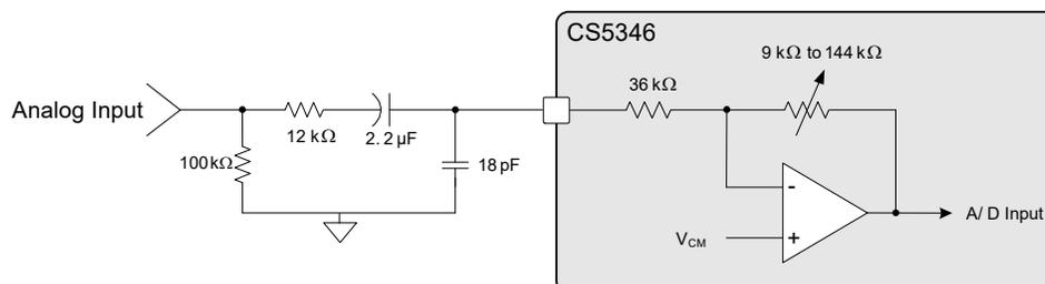
Figure 13. 2 V<sub>RMS</sub> Input Circuit
