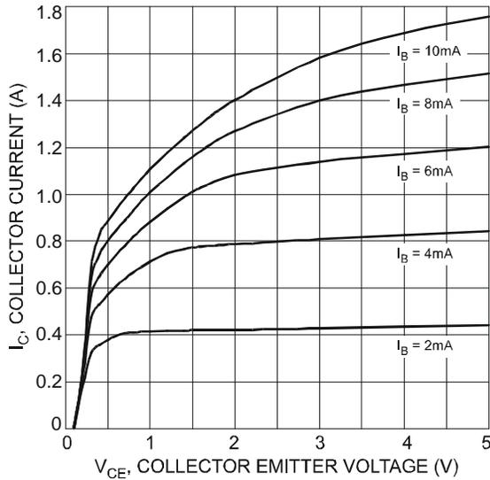
Figure 1. Typical Collector Current vs. Collector-Emitter Voltage
