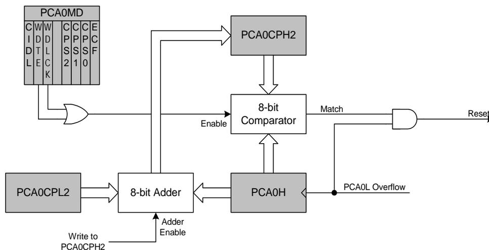
Figure 16.10. PCA Module 2 with Watchdog Timer Enabled
