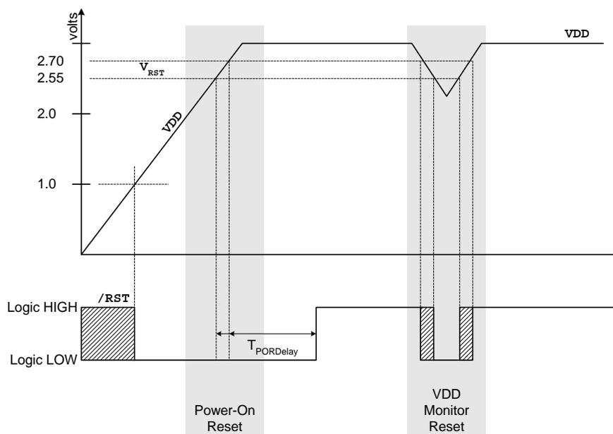
Figure 9.2. Power-On and  $V_{\text{DD}}$  Monitor Reset Timing
