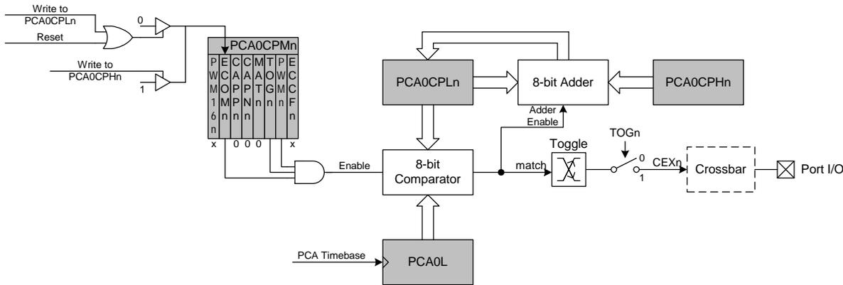
Figure 16.7. PCA Frequency Output Mode
