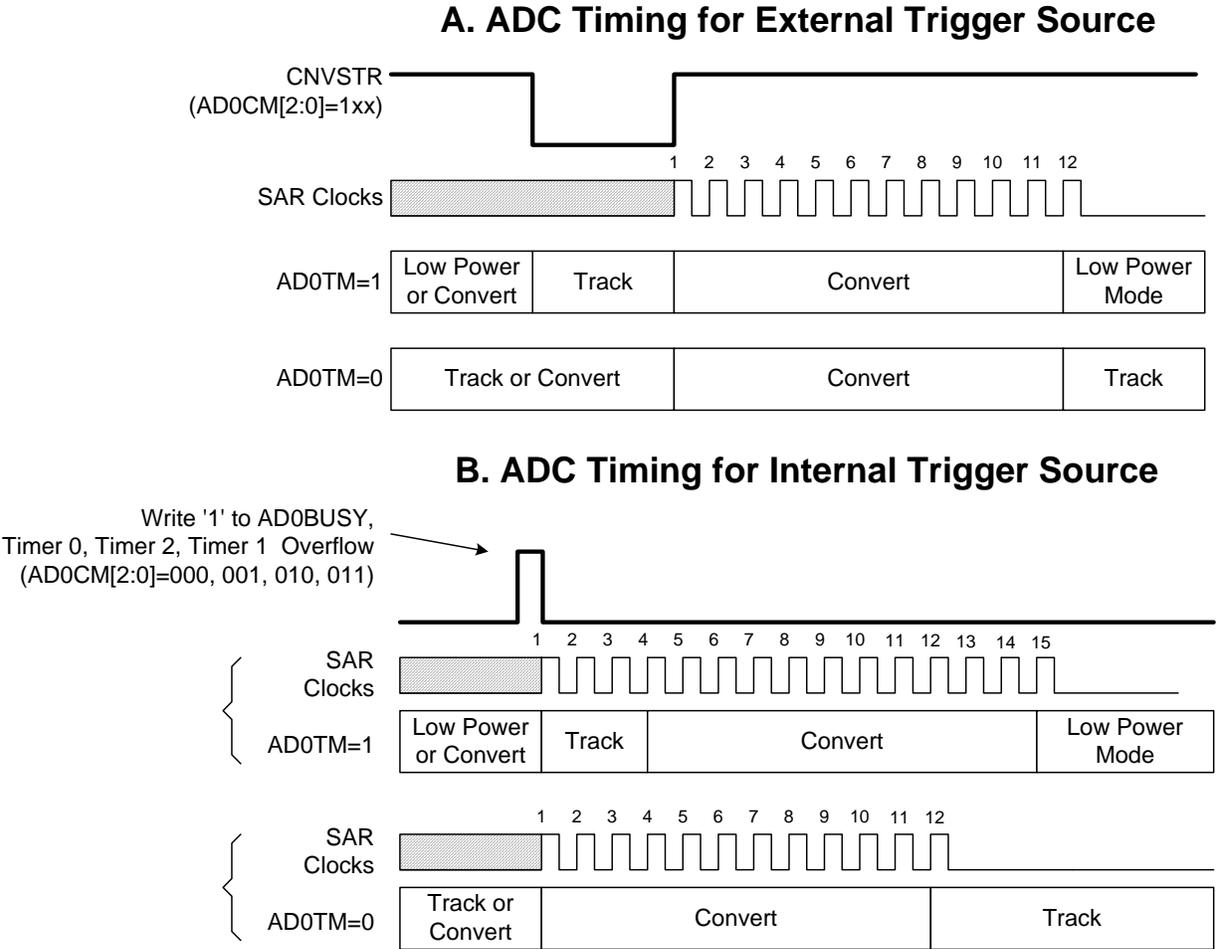
**Figure 5.4. 8-Bit ADC Track and Conversion Example Timing**
