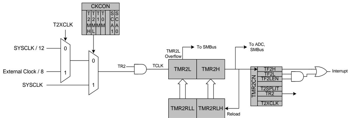
Figure 15.4. Timer 2 16-Bit Mode Block Diagram
