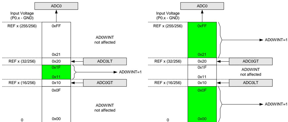
Figure 5.6. ADC Window Compare Examples, Single-Ended Mode
