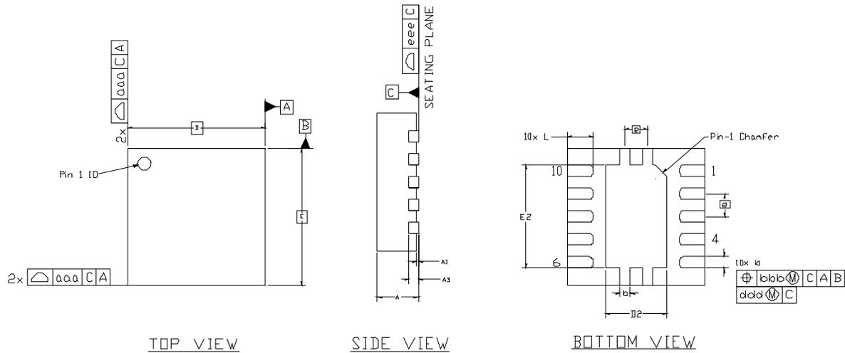
**Figure 4.2. QFN-11 Package Drawing**
