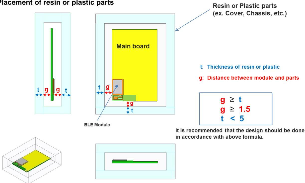
Please do not apply molding over the antenna area of BLE module.
