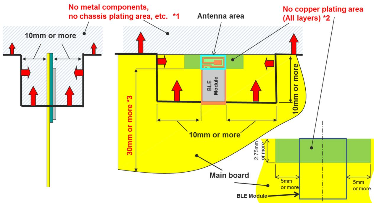
\*1 Please do not place any metal components in blue shaded space,(\*1) such as signal line and metal chassis as possible except for main board while mounting the components in \*1 space on the main board is allowed except for no copper plating area. (\*2).
