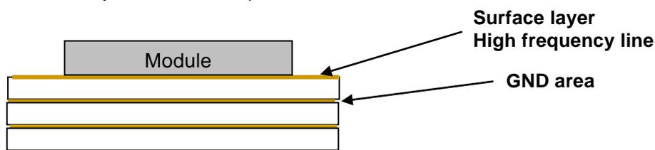
GND pattern of each layer should be connected to GND area with large number of vias.
