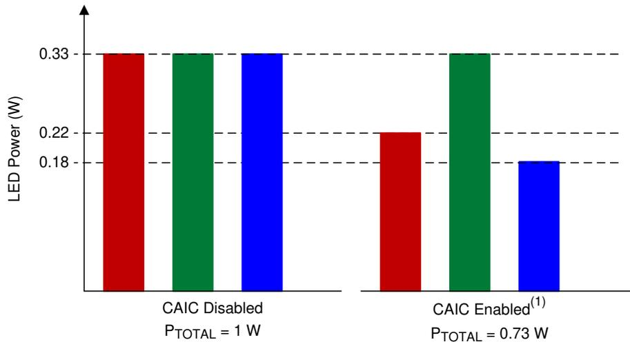
(1) With CAIC enabled, if red and blue LEDs require less than nominal power for a given input image, the red and blue LED power will reduce.
