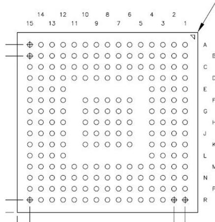
**Figure 5-2. ZEZ Package 201-Pin NFBGA Bottom View**
