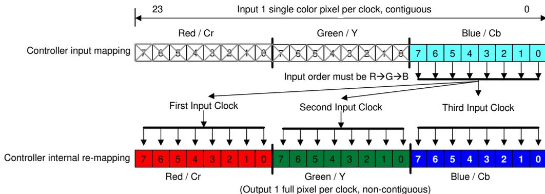
Figure 7-6. 8-Bit RGB-888 or YCbCr-888 I/O Mapping
