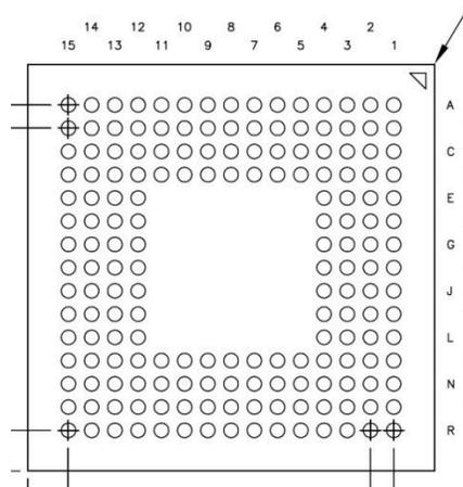
Figure 5-1. ZVB Package 176-Pin NFBGA Bottom View
