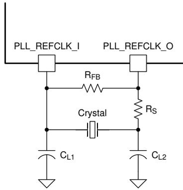
$C_L$  = Crystal load capacitance (farads)
