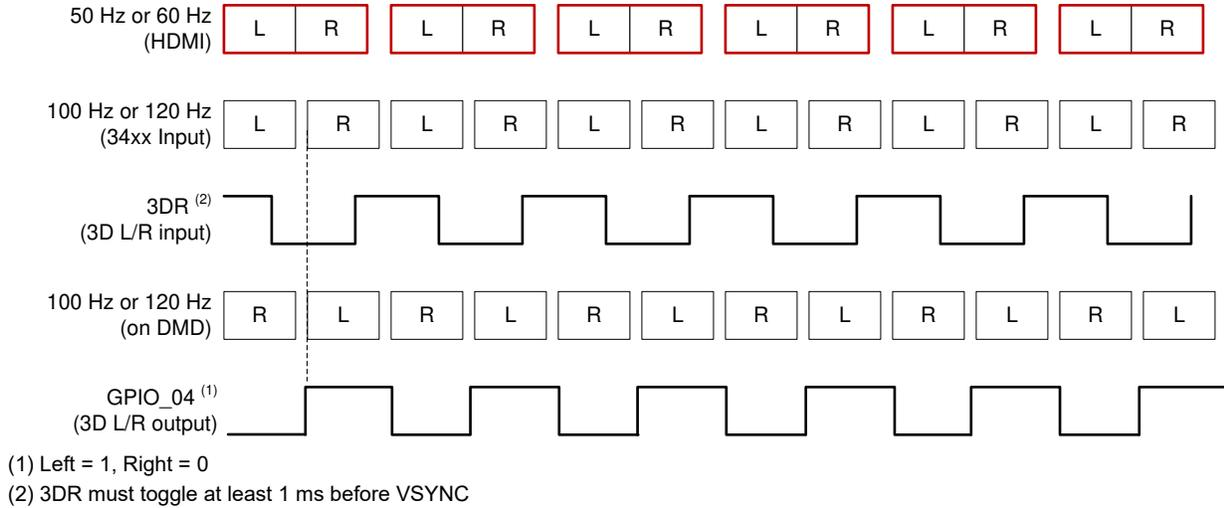
**Figure 7-1. 3D Display Left and Right Frame Timing**
