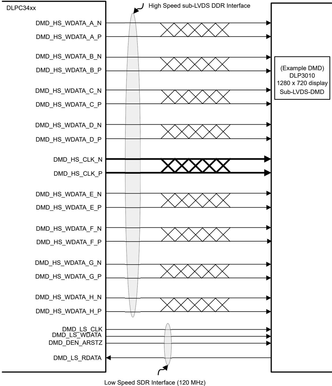
**Figure 7-16. DLP3010 (.3 720p) DMD Interface Example**
