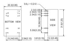
Pin Size is Tolerance 0.5 $\pm$ 0.05mm, Tolerance .X or .XX=  $\pm$ 0.5mm
