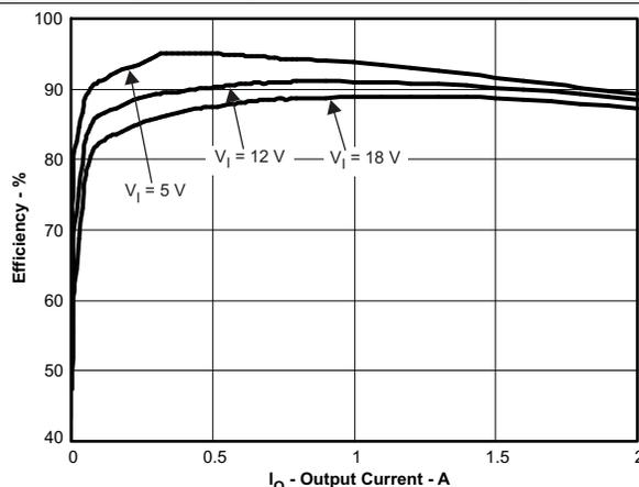
$V_{OUT1} = 3.3\text{ V}$
