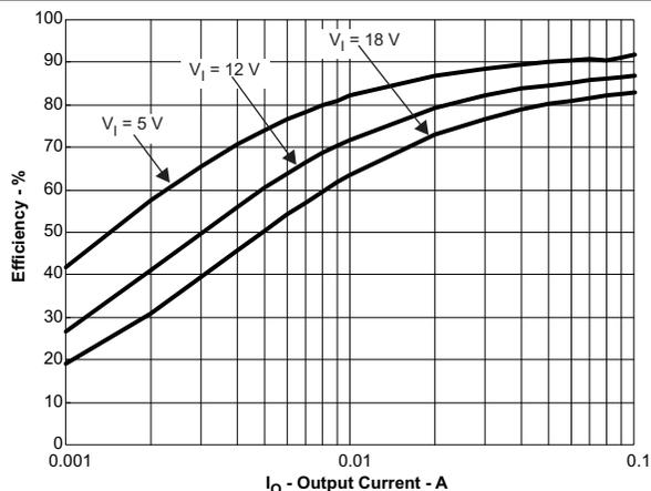
$V_{OUT1} = 3.3\text{ V}$
