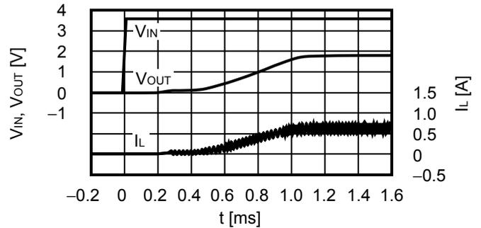
**3.2 Shutdown pin response ( $V_{OUT} = 1.8\text{ V}$ ,  $V_{IN} = 3.6\text{ V}$ ,  $V_{ON/OFF} = 0\text{ V} \rightarrow 3.6\text{ V}$ ,  $T_a = +25^\circ\text{C}$ )**
