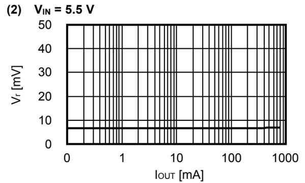
**3.4  $V_{OUT} = 4.0\text{ V}$  ( $R_{FB1} = 51\text{ k}\Omega$ ,  $R_{FB2} = 9\text{ k}\Omega$ )**
