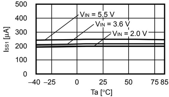
**2. 2 Current consumption during shutdown ( $I_{SSS}$ ) vs. Temperature ( $T_a$ )**
