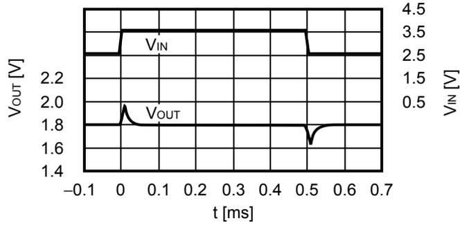
**3.4 Load fluctuations ( $V_{OUT} = 1.8\text{ V}$ ,  $V_{IN} = 3.6\text{ V}$ ,  $T_a = +25^\circ\text{C}$ )**
