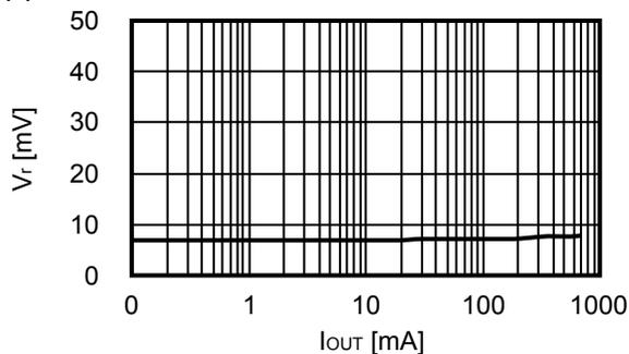
**3.2  $V_{OUT} = 1.8\text{ V}$  ( $R_{FB1} = 36\text{ k}\Omega$ ,  $R_{FB2} = 18\text{ k}\Omega$ )**
