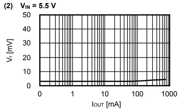
**3.3  $V_{OUT} = 3.3\text{ V}$  ( $R_{FB1} = 36\text{ k}\Omega$ ,  $R_{FB2} = 8\text{ k}\Omega$ )**
