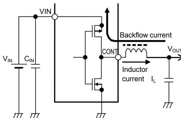
**Figure 12 Backflow Current**
