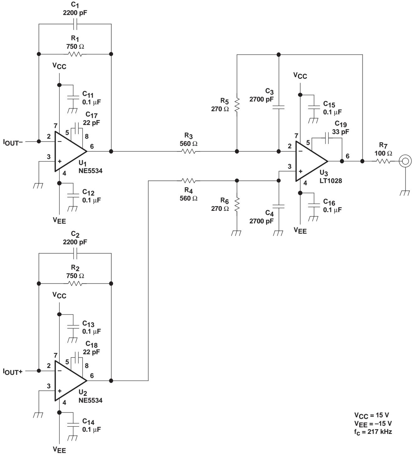
Figure 36. Measurement Circuit for PCM, V<sub>OUT</sub> = 2 V rms
