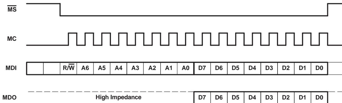
NOTE: Bit 15 is used for selection of write or read. Setting  $\overline{R/W} = 0$  indicates a write, while  $\overline{R/W} = 1$  indicates a read. Bits 14–8 are used for the register address. Bits 7–0 are used for register data.
