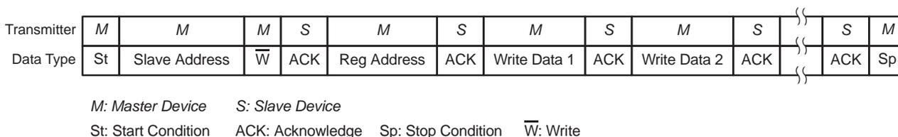
Figure 33. Write Operation
