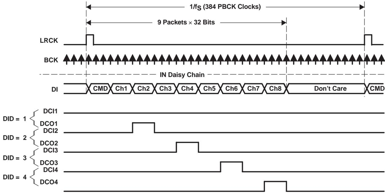
Figure 61. DCO Output Timing of TDMCA Mode Operation
