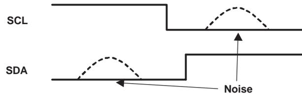
When these conditions occur at the same time, the PCM1792A erroneously detects a start or stop condition.
