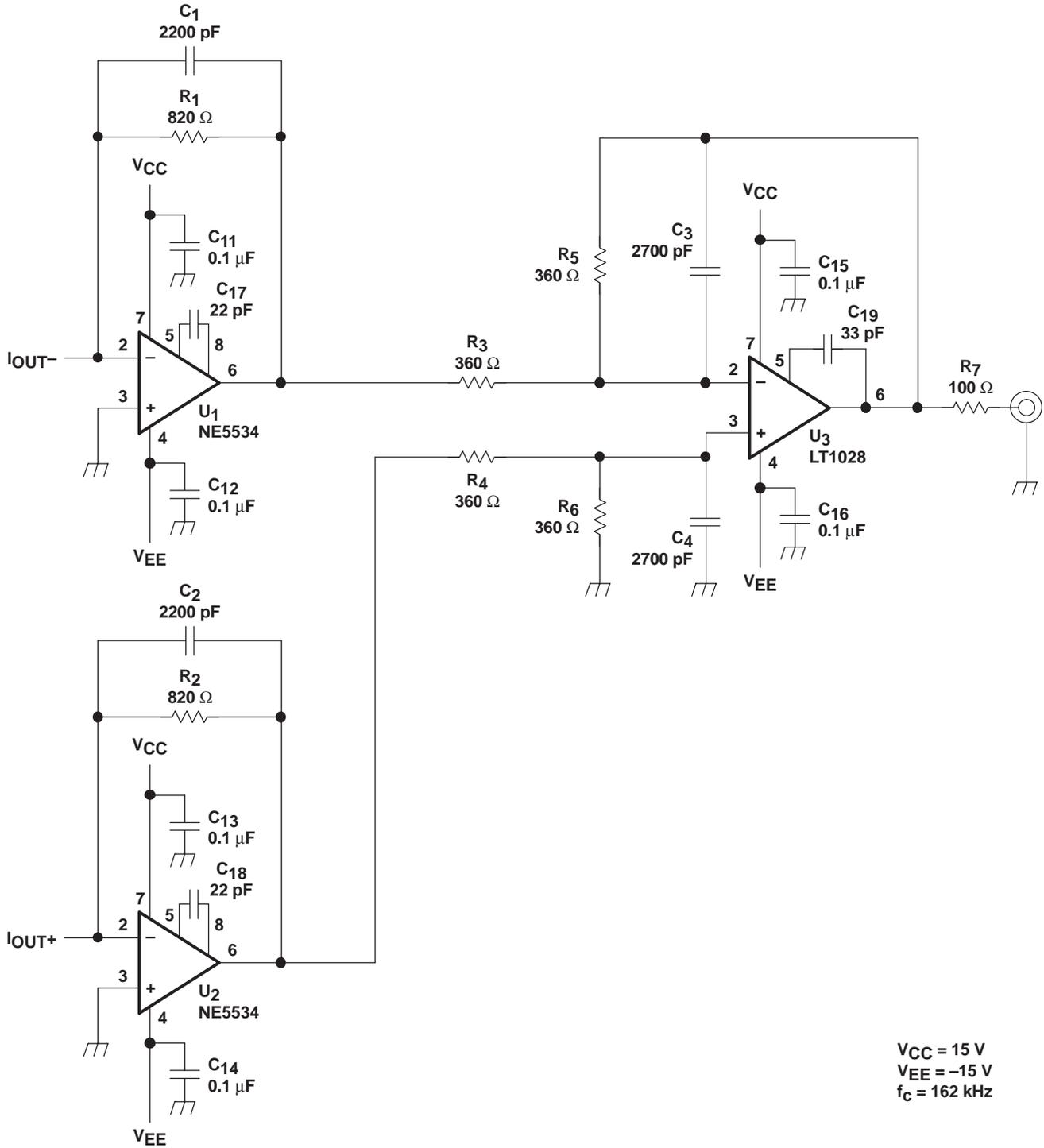
Figure 37. Measurement Circuit for PCM, V<sub>OUT</sub> = 4.5 V rms
