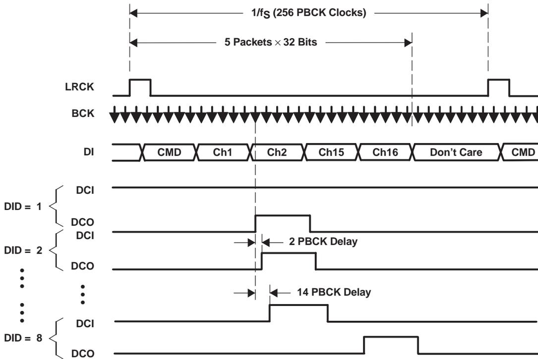
Figure 62. DCO Output Timing With Skip Operation
