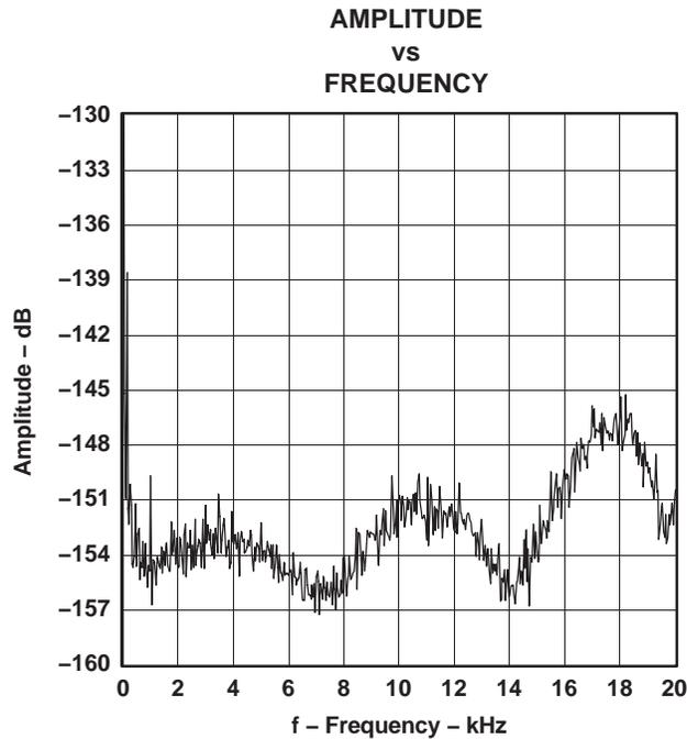
Figure 23. -150-dB Output Spectrum, DSD Mono Mode
