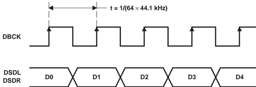
**Figure 44. Normal Data Output Form From DSD Decoder**
