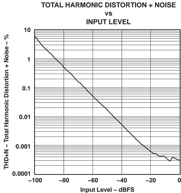
**Figure 21. THD+N vs Input Level, PCM Mode**
