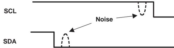
When these conditions occur at the same time, the PCM1792A fails to detect a start condition.
