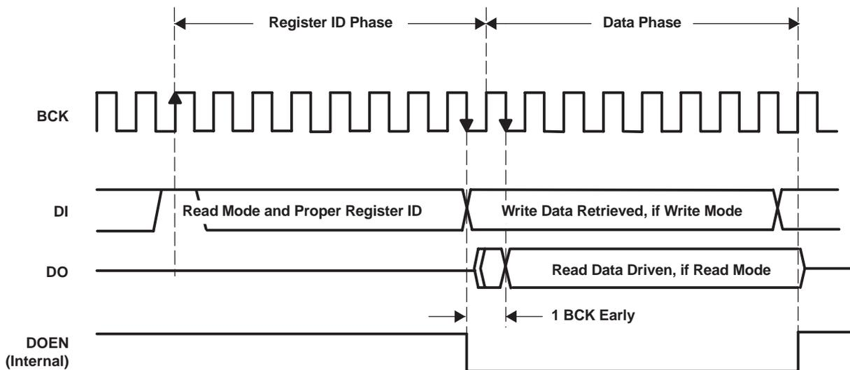
Figure 60. TDMCA Write and Read Operation Timing
