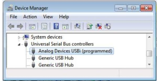
Figure 9. Confirming Driver Installation Using the Device Manager
