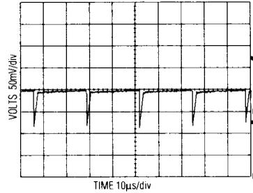
REGULATOR 7 V<sub>OUT</sub> = -30V WITH 150kΩ LOAD
