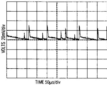
REGULATOR 8 V<sub>OUT</sub> = +15V WITH 1.5kΩ LOAD
