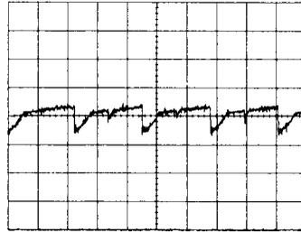
REGULATOR 6 V<sub>OUT</sub> = -5V WITH 250kΩ LOAD
