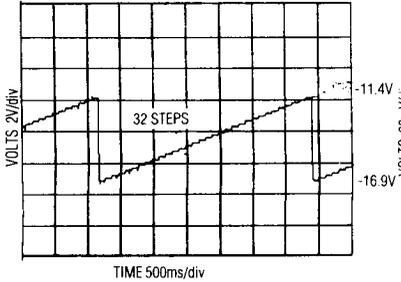
REGULATOR 7 V<sub>OUT</sub> = -11.4 TO -16.9 V WITH 10kΩ LOAD
