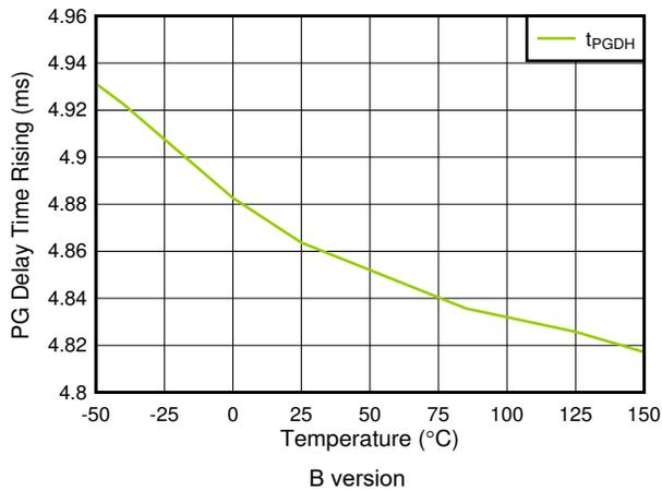
Figure 6-25.  $t_{PGDH}$  vs Temperature (For TPS746B Only)
