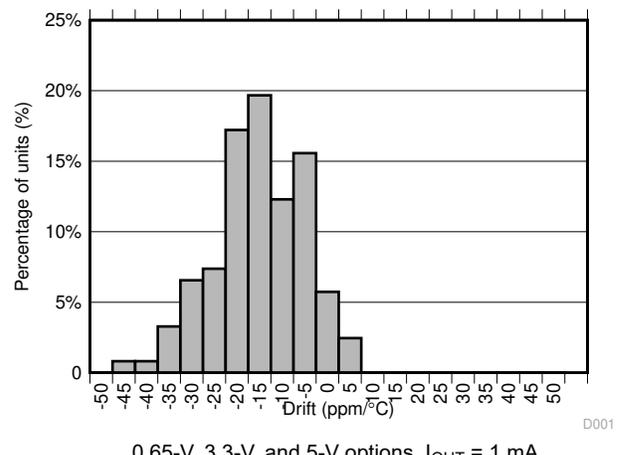
Figure 6-4. Temperature Drift Histogram ( $-40^\circ\text{C}$  to  $+25^\circ\text{C}$ )
