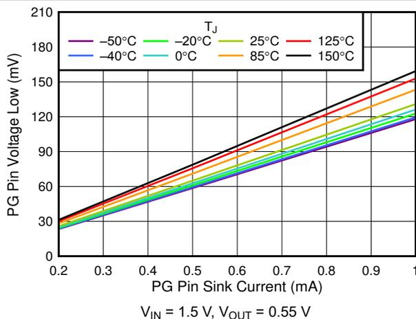
Figure 6-23.  $V_{OL(PG)}$  vs PG Pin Sink Current
