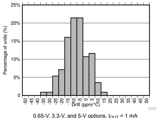
Figure 6-5. Temperature Drift Histogram ( $25^\circ\text{C}$  to  $150^\circ\text{C}$ )
