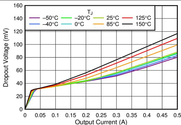
Figure 6-11. 5.5-V Dropout Voltage vs  $I_{OUT}$
