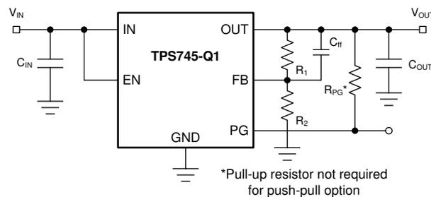
**Figure 8-1. Adjustable Operation**
