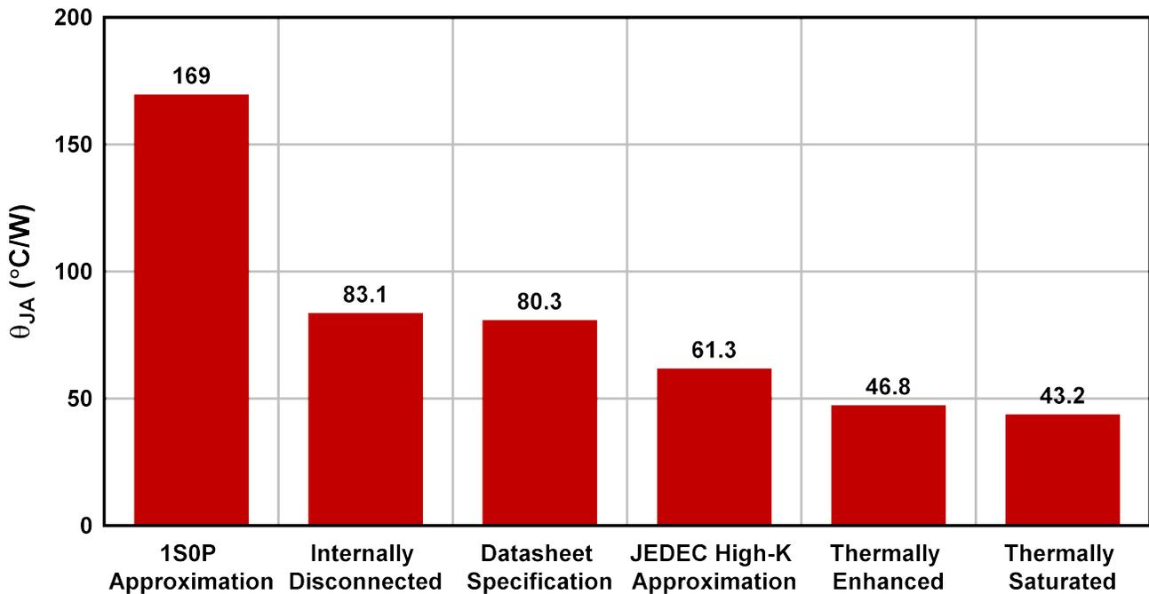
**Figure 8-8. TPS745-Q1 (WSN)  $R_{\theta JA}$  versus Board Layout**
