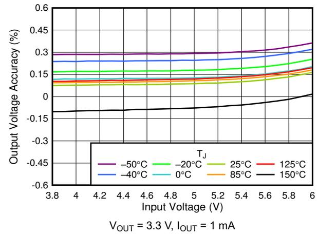
Figure 6-6. 3.3-V Line Regulation vs  $V_{IN}$
