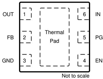
**Figure 5-1. DRV Package, 6-Pin Adjustable WSON (Top View)**
