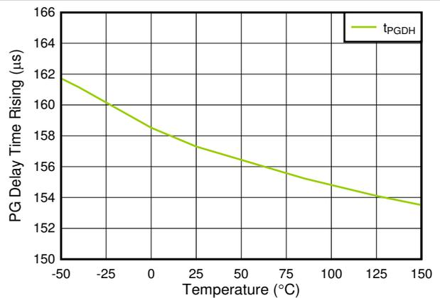
Figure 6-24.  $t_{PGDH}$  vs Temperature
