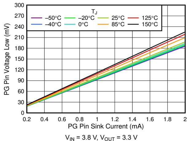
Figure 6-22.  $V_{OL(PG)}$  vs PG Pin Sink Current
