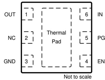
**Figure 5-2. DRV Package, 6-Pin Fixed WSON (Top View)**
