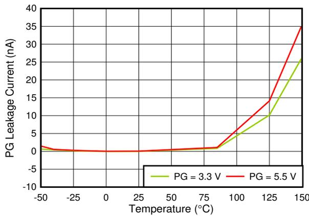
Figure 6-21.  $I_{kg(PG)}$  vs Temperature and PG Pin Voltage
