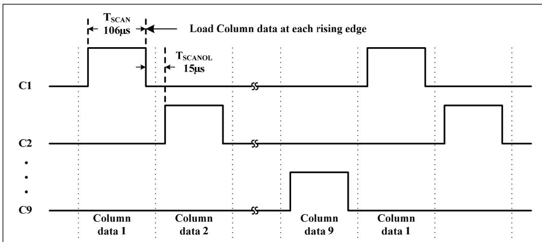
Figure 2 Scanning timing
