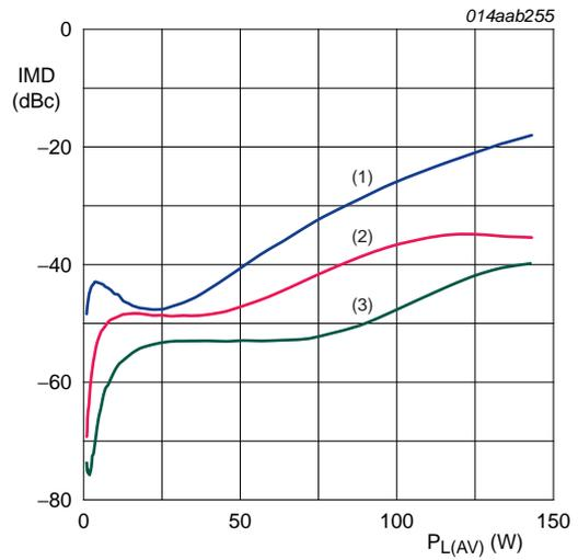
$V_{DS} = 28$  V;  $I_{Dq} = 1600$  mA;  $f = 1511$  MHz;
