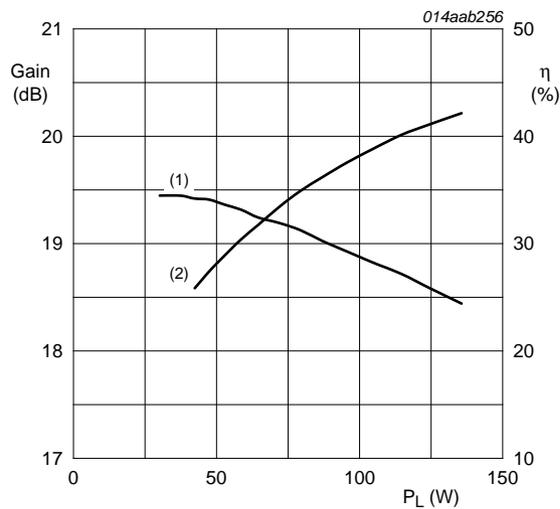
$V_{DS} = 28$  V;  $I_{Dq} = 1600$  mA;  $f = 1511$  MHz;
