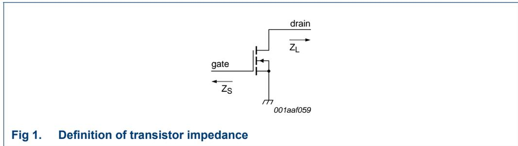
Fig 1. Definition of transistor impedance
