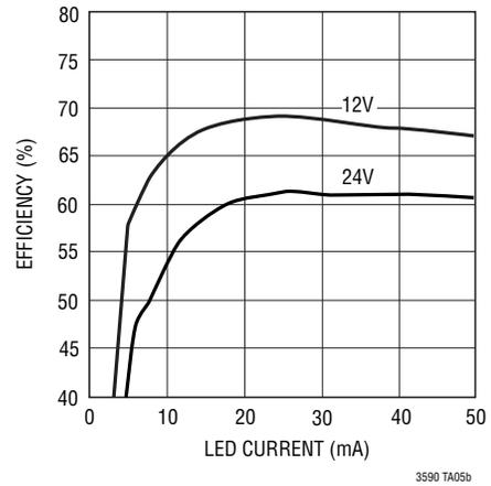
48V Supply for Two Strings of 10 LEDs, 25mA Current
