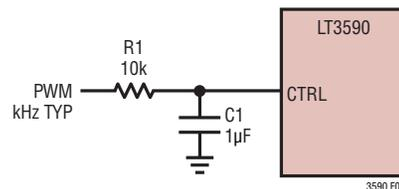
**Figure 5. Dimming Control Using a Filtered PWM Signal**
