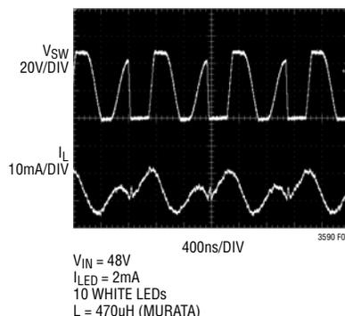
Figure 2. Switching Waveforms
