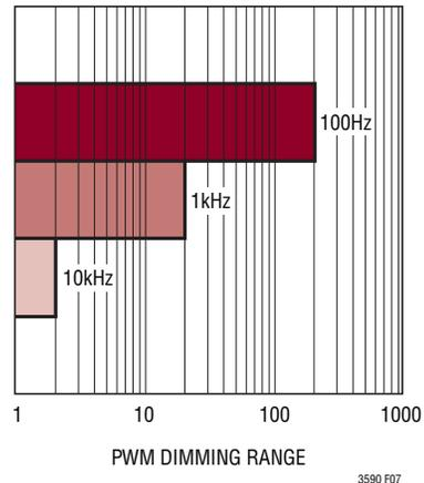
Figure 7. Dimming Range Comparison of Three PWM Frequencies
