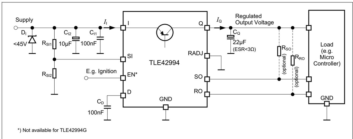
**Figure 10 Application diagram with selecting default reset thresholds**
