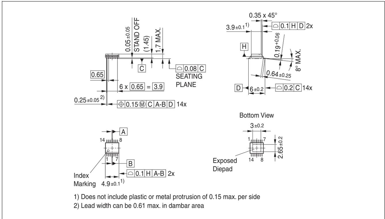
**Figure 14 PG-SSOP-14 exposed pad<sup>1)</sup>**
