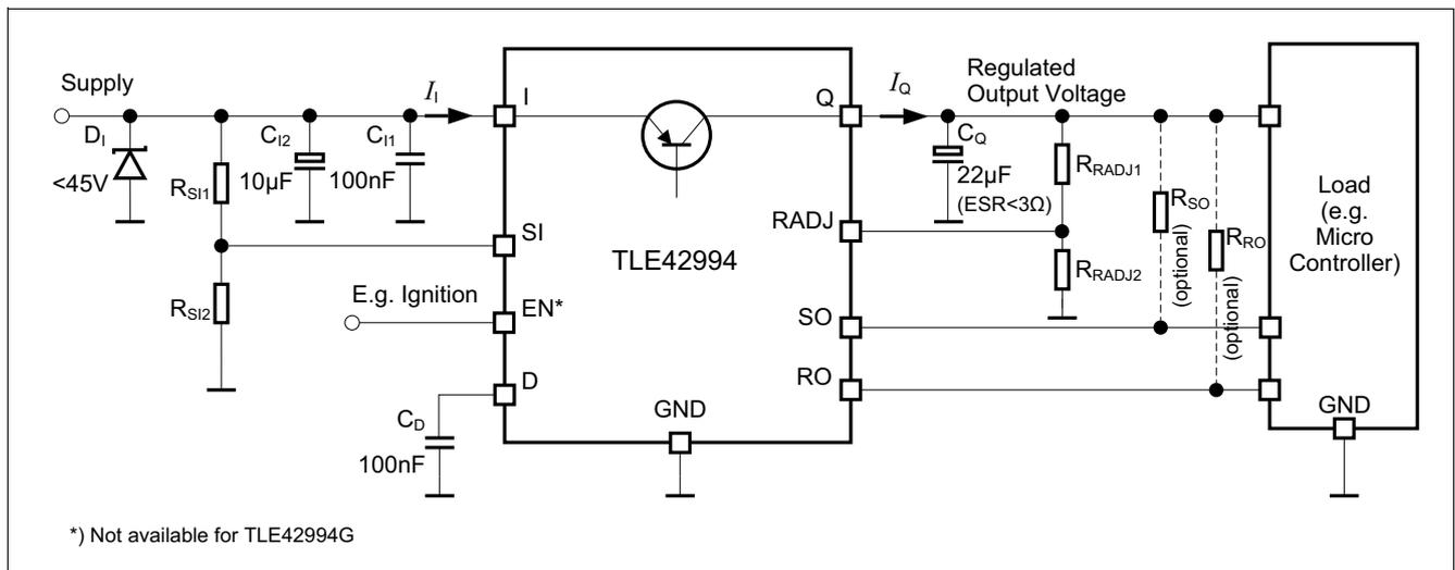
**Figure 11 Application diagram with reset thresholds adjustment**
