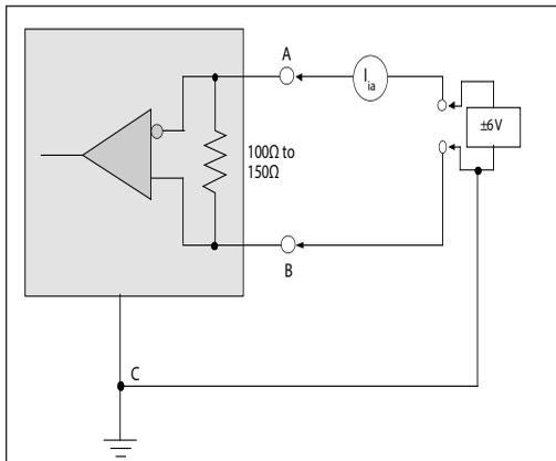
Figure 23. V.11 Receiver Input Current w/ Termination
