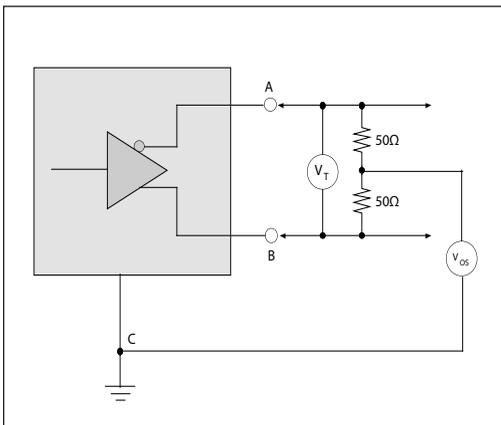
Figure 17. V.11 Driver Output Test Terminated Voltage
