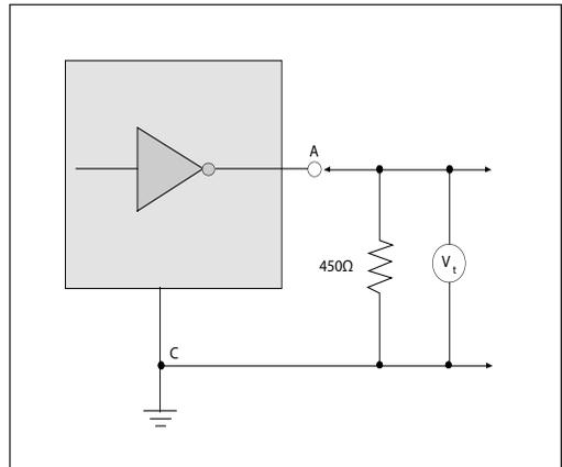
Figure 10. V.10 Driver Output Test Terminated Voltage
