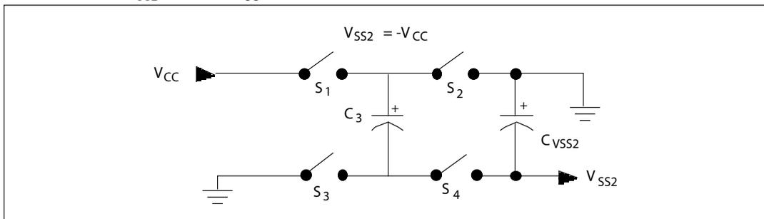
Figure 49. Circuit for an Ideal Voltage Inverter.
