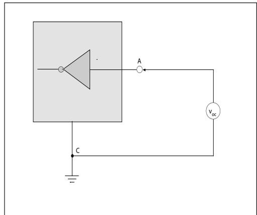
Figure 8. V.28 Receiver Input Open Circuit Bias
