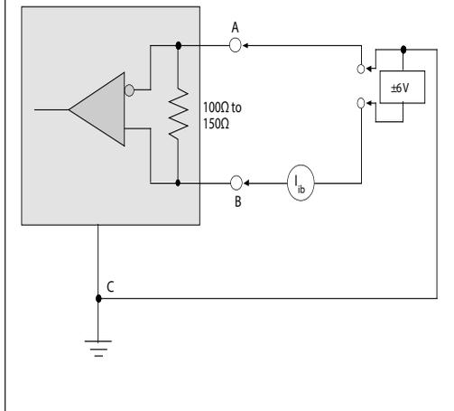
Figure 25. V.11 Receiver Input Current w/ Termination
