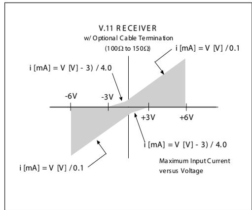
Figure 24. V.11 Receiver Input Graph with Termination
