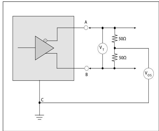
Figure 26. V.35 Driver Output Test Terminated Voltage
