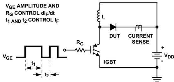
**Figure 9.  $t_{rr}$  Waveforms and Definitions**
