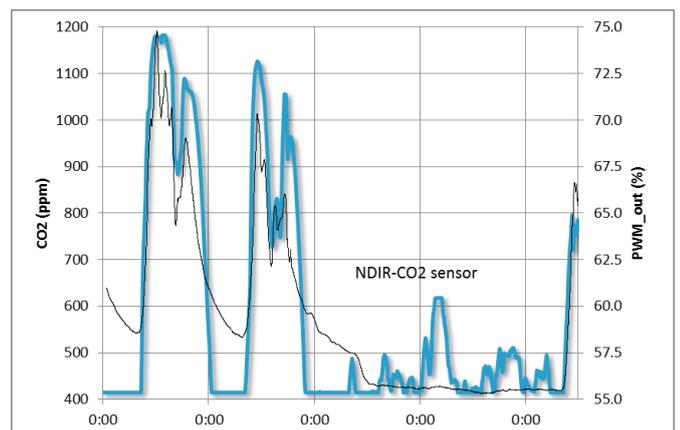
Comparison between MICS-VZ-89TE output signal and NDIR CO<sub>2</sub> sensor signal over a duration of 4 consecutive days (Thu – Sun)
