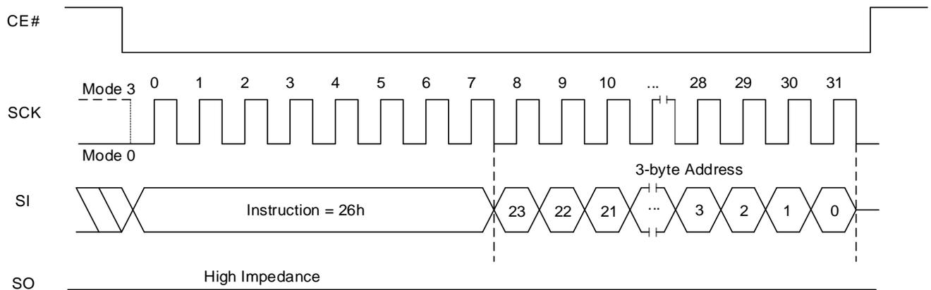
**Figure 8.71 Sector Unlock Sequence In QPI Mode**
