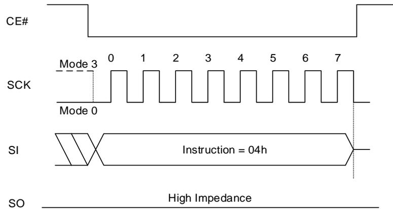
**Figure 8.25 Write Disable Sequence In QPI Mode**
