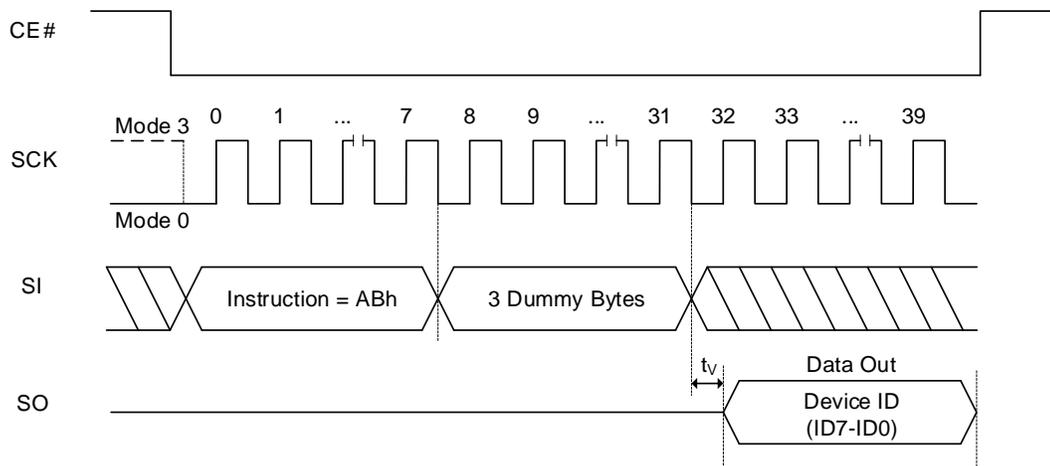
**Figure 8.51 Read Product Identification Sequence In QPI Mode**
