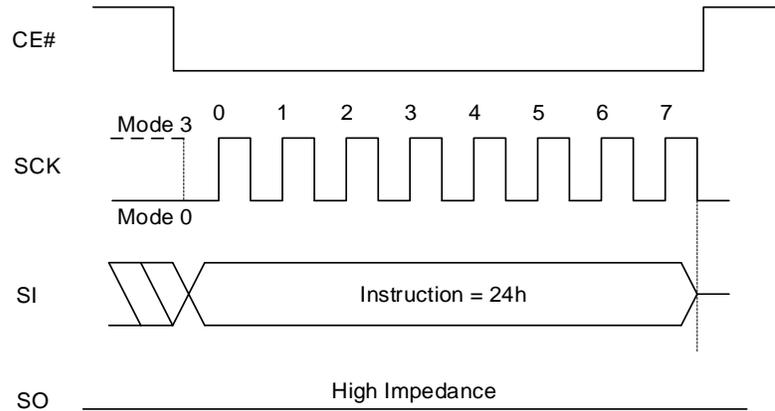
**Figure 8.73 Sector Lock Sequence In QPI Mode**
