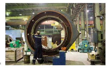
What are the standard signals, where are they sent, and how are they converted? RTD sensors will output a resistance. As the motor/generator is operating, the resistance will rise with the temperature of the motor. If a hot spot occurs or other failure takes place within the stator that causes the temperature to spike, the resistance of the sensor will also spike. This will be transmitted to the instrumentation used to monitor the motor or generator and will then trigger an alarm.
