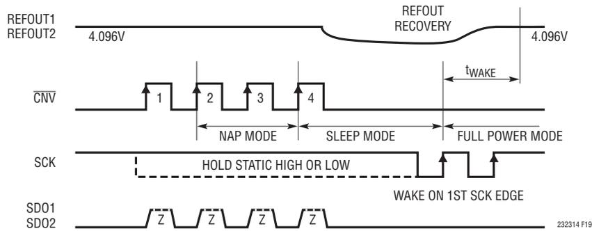
Figure 19. CMOS Mode SLEEP and WAKE Using SCK
