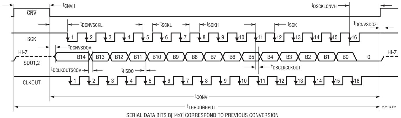
Figure 21. LTC2323-14 Timing Diagram
