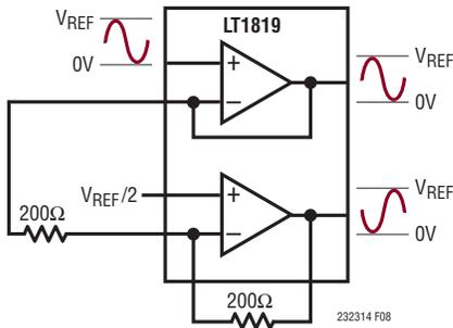
Figure 8. Single-Ended to Differential Driver
