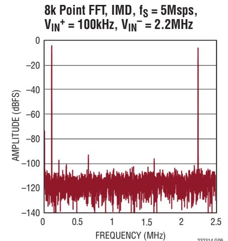
**TYPICAL PERFORMANCE CHARACTERISTICS**  $T_A = 25^\circ\text{C}$ ,  $V_{DD} = 5\text{V}$ ,  $OV_{DD} = 2.5\text{V}$ ,
