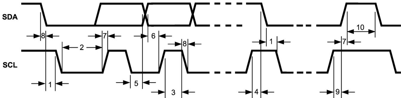
Figure 1. I<sup>2</sup>C Timing Parameters
