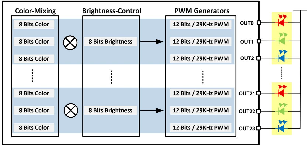
Figure 9. PWM Control Scheme for Each Channel
