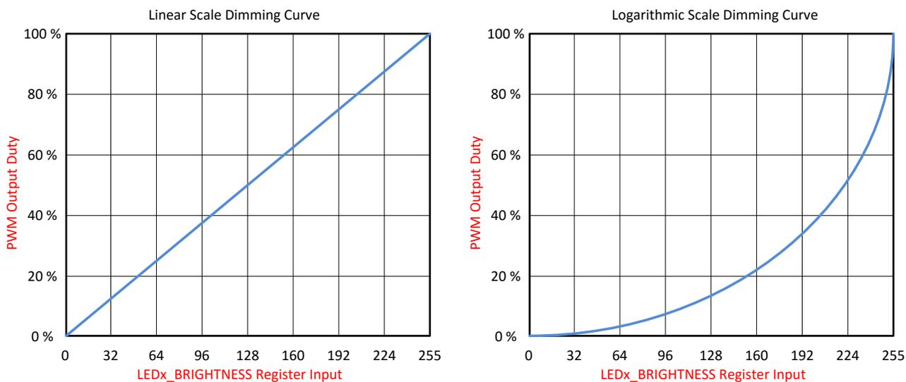
Figure 11. Logarithmic vs Linear Dimming Curve
