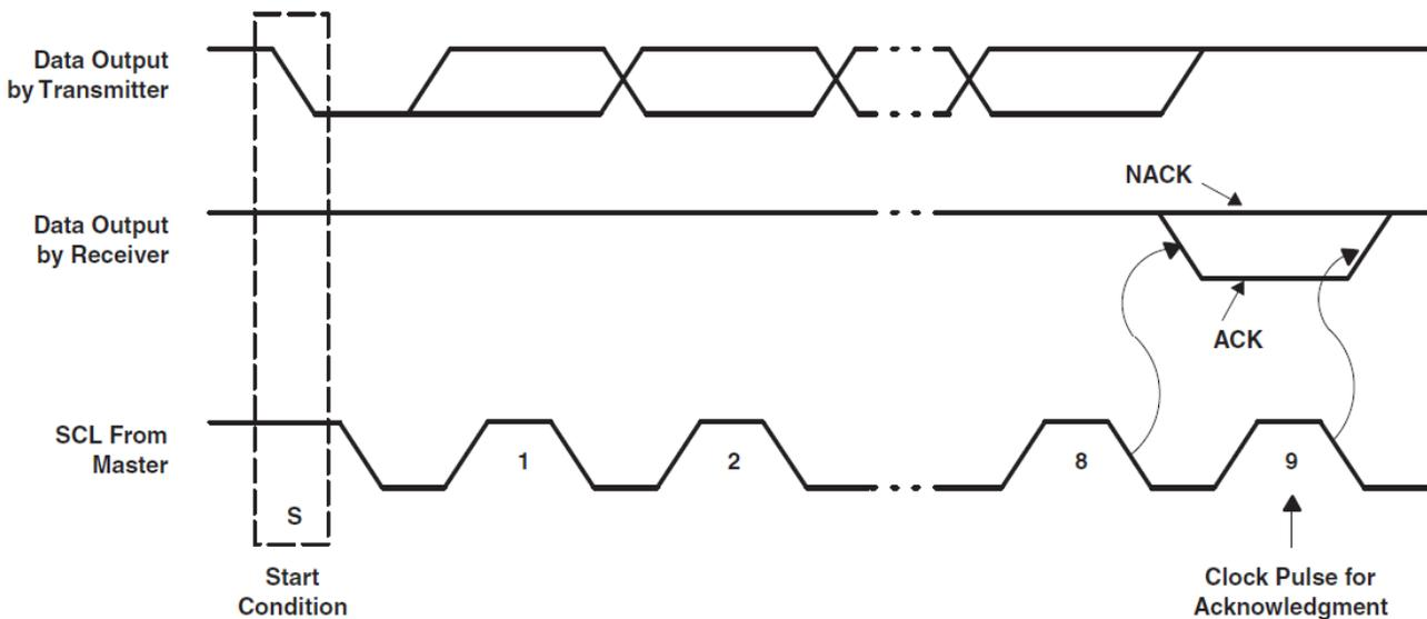
Figure 18. Acknowledge and Not Acknowledge on I<sup>2</sup>C Bus
