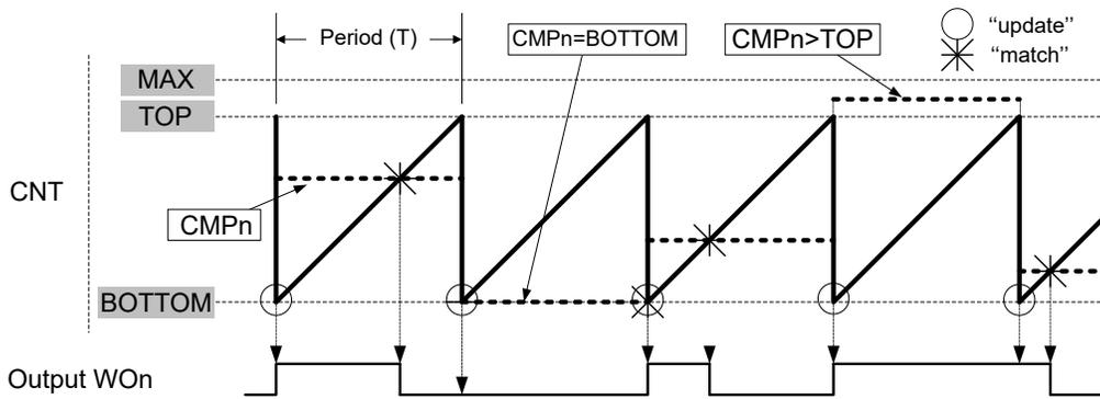
**Note:** The representation in the figure above is valid for when CMP $n$  is updated using CMPnBUF.
