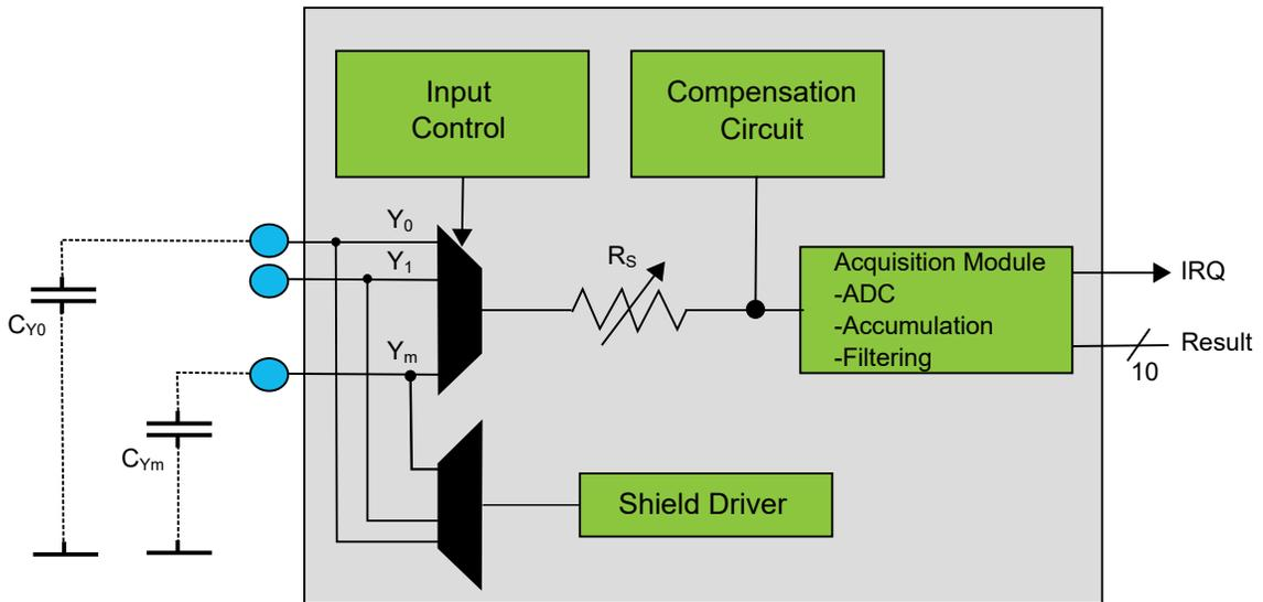
**Note:** The internal series resistor,  $R_S$ , has limited effect in Self-Capacitance mode. It is always recommended to add an external series resistor.
