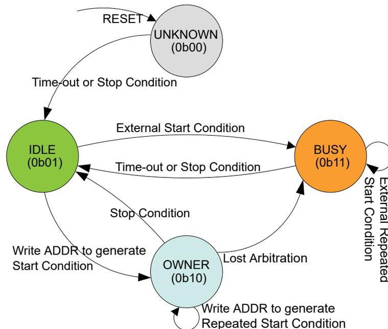
1. **Unknown:** The bus state machine is active when the TWI master is enabled. After the TWI master has been enabled, the bus state is Unknown. The bus state will also be set to Unknown after a System Reset is performed or after the TWI master is disabled.
