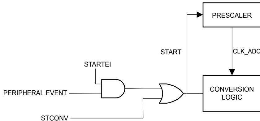
In Free-Running mode, the first conversion is started by writing a '1' to the STCONV bit in the ADCn.COMMAND register. A new conversion cycle is started immediately after the previous conversion cycle has completed. A completed conversion will set the RESRDY flag in the ADCn.INTFLAGS register.
