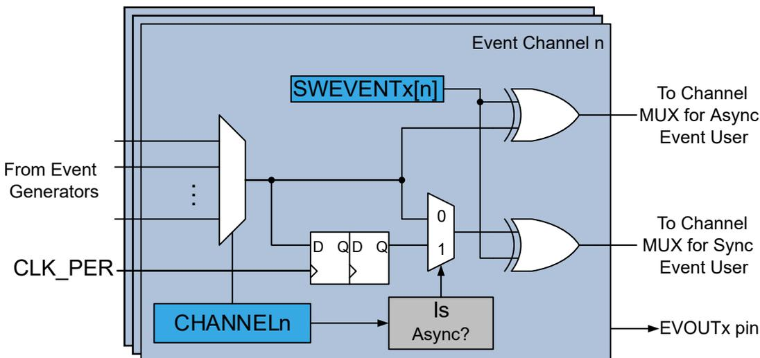
The block diagram shows the operation of an event channel. A multiplexer controlled by Channel n Generator Selection (EVSYS.CHANNELn) register at the input selects which of the event sources to route onto the event channel. Each event channel has two subchannels: one asynchronous and one synchronous. A synchronous user will listen to the synchronous subchannel, and an asynchronous user will listen to the asynchronous subchannel.
