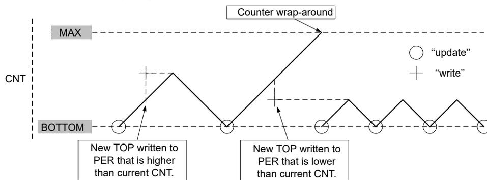
**With Buffering:** When double-buffering is used, the buffer can be written at any time and still maintain correct operation. The TCA<sub>n</sub>.PER is always updated on the UPDATE condition, as shown for dual-slope operation in the figure below. This prevents wrap-around and the generation of odd waveforms.
