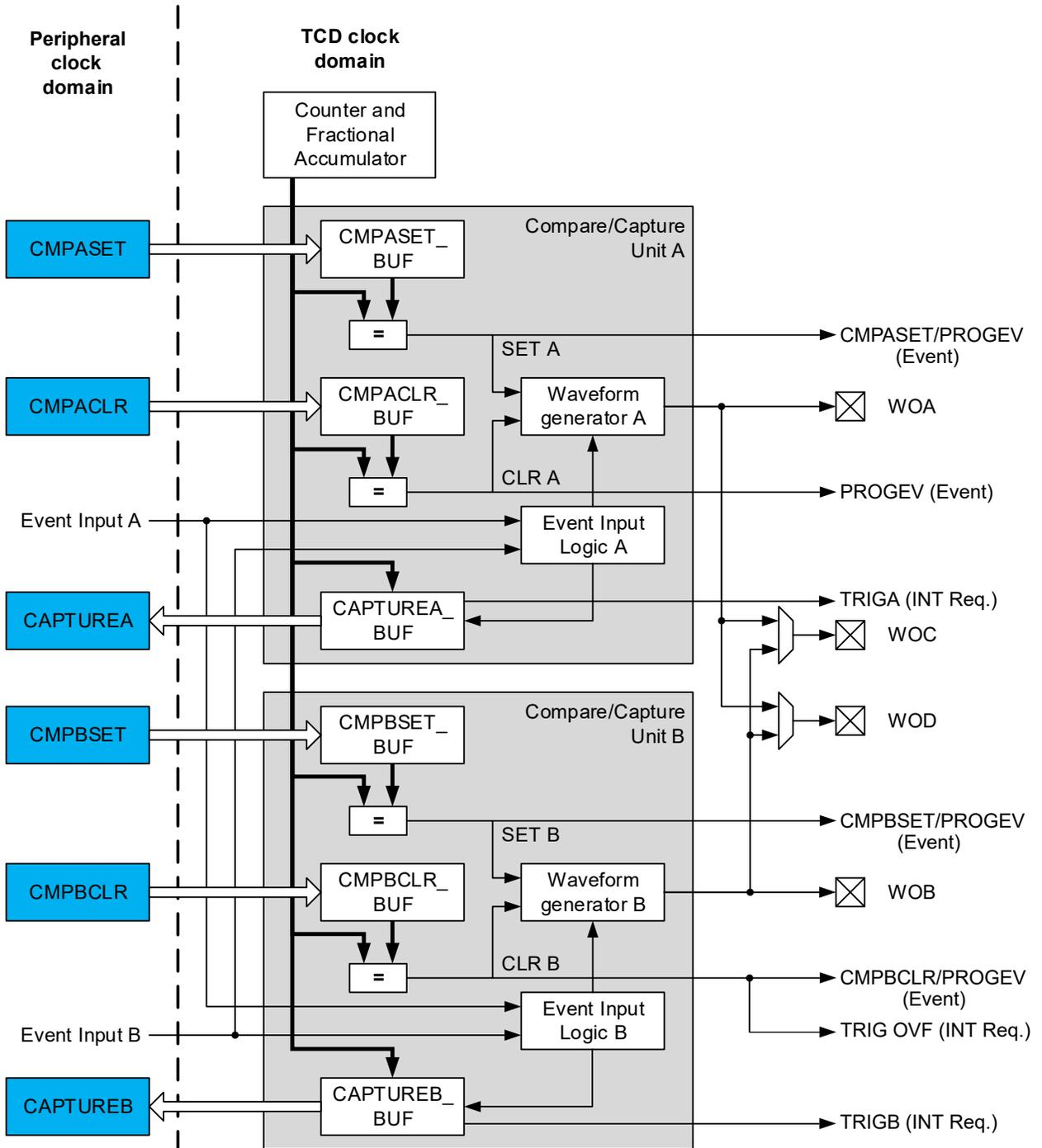
The TCD core is asynchronous to the peripheral clock. The timer/counter consists of two compare/capture units, each with a separate waveform output. There are also two extra waveform outputs which can be equal to the output from one of the units. For each compare/capture unit, there is a pair of compare registers which are stored in the respective peripheral registers (TCDn.CMPASET, TCDn.CMPACLR, TCDn.CMPBSET, TCDn.CMPBCLR).
