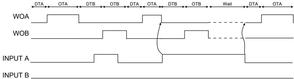
If Input mode 2 is used on input B, an event will only have an effect if the TCD is in dead time B or on time B, and it will only affect the WOB output.
