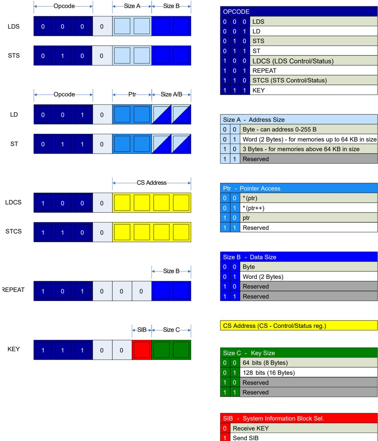
35.3.3.1 LDS - Load Data from Data Space Using Direct Addressing
