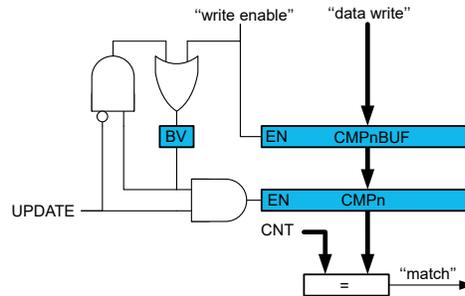
Both the TCA<sub>n</sub>.CMP<sub>n</sub> and TCA<sub>n</sub>.CMP<sub>n</sub>BUF registers are available as I/O registers. This allows initialization and bypassing of the buffer register and the double-buffering function.
