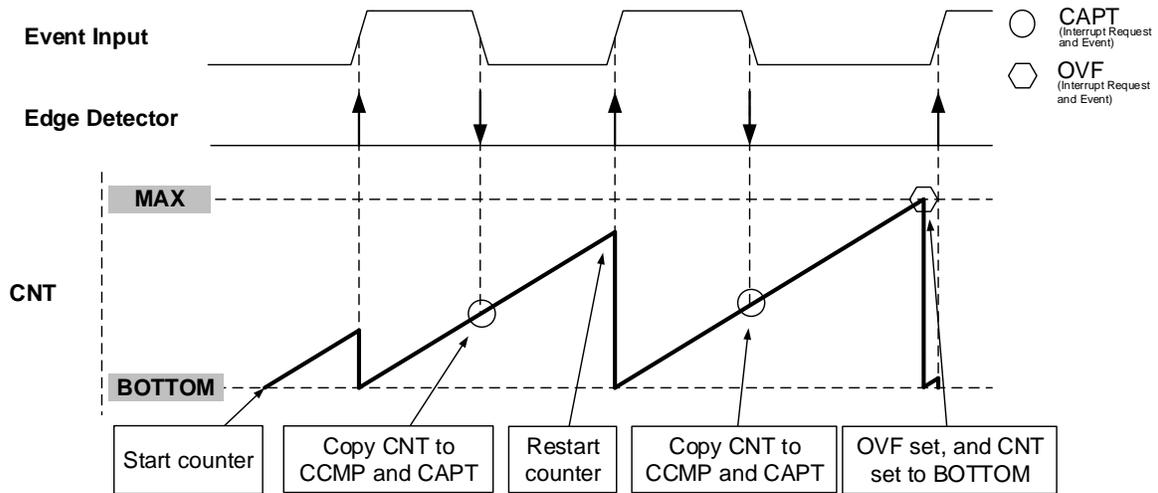
22.3.3.1.6 Input Capture Frequency and Pulse-Width Measurement Mode
