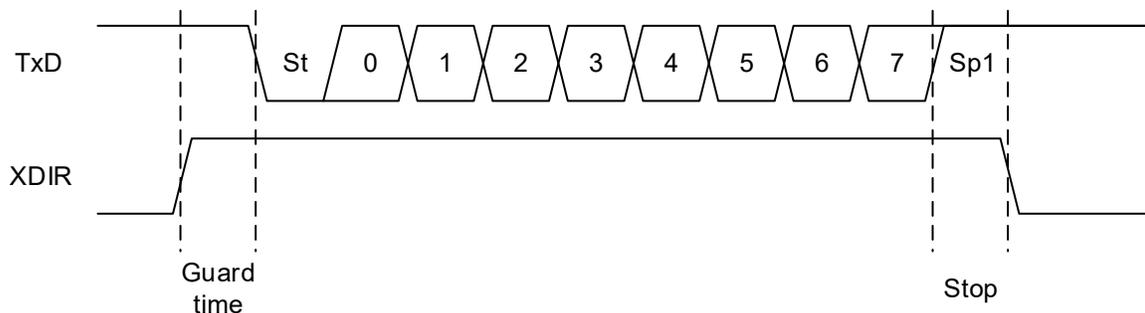
RS-485 mode is compatible with One-Wire mode. One-Wire mode enables an internal connection between the TXD pin and the USART receiver, making the TXD pin a combined TxD/RxD line. The RXD pin will be disconnected from the USART receiver and may be controlled by a different peripheral. An example of such a circuit is shown in the figure below.
