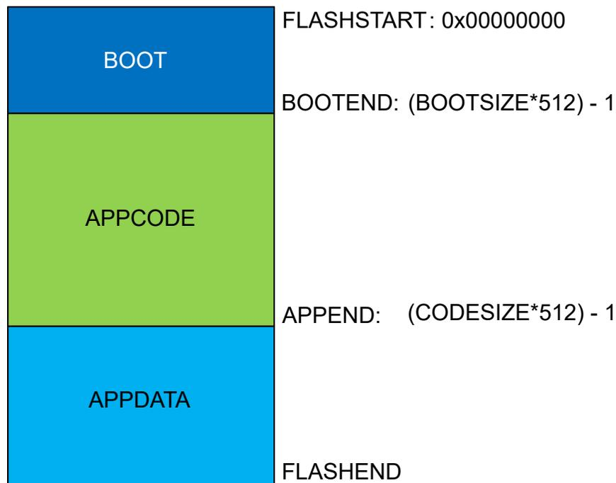
If FUSE.BOOTSIZE is written to '0', the entire Flash is regarded as the BOOT section. If FUSE.CODESIZE is written to '0' and FUSE.BOOTSIZE > 0, the APPCODE section runs from BOOTEND to the end of Flash (no APPDATA section).
