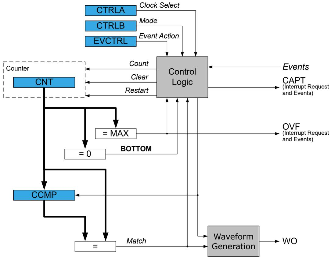
The timer/counter can be clocked from the Peripheral Clock (CLK\_PER), from a 16-bit Timer/Counter type A (CLK\_TCA<sub>n</sub>) or the Event System (EVSYS).
