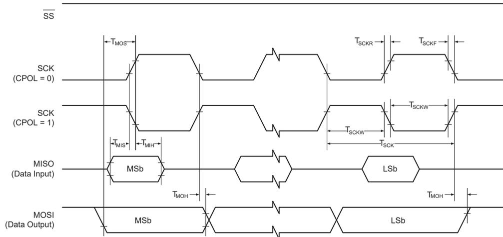
**Table 37-19. SPI - Timing Characteristics in Master Mode**
