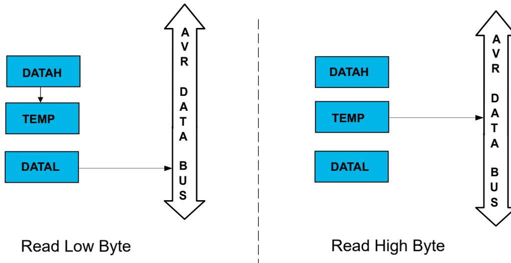
For a 16-bit read operation, the low byte register (e.g., DATAL) of the 16-bit register must be read before the high byte register (e.g., DATAH). When the low byte register is read, the high byte register of the 16-bit register is copied into the temporary (TEMP) register in the same clock cycle, as shown on the left side of [Figure 7-3](#). Reading the high byte register will result in a read from TEMP instead of the high byte register, as shown on the right side of [Figure 7-3](#).
