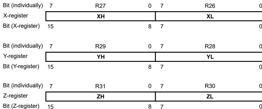
The lowest register address holds the Least Significant Byte (LSB), and the highest register address holds the Most Significant Byte (MSB). These address registers can function as fixed displacement, automatic increment, and automatic decrement, with different *LD\*/ST\** instructions. See the *Instruction Set Summary* section for details.
