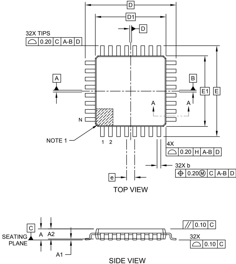
**32-Lead Plastic Thin Quad Flatpack (PT) - 7x7x1.0 mm Body [TQFP]
