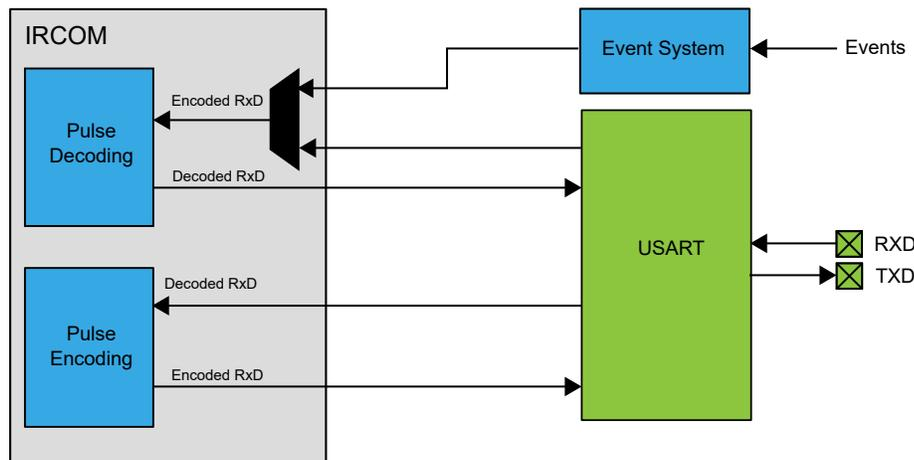
The USART is set in IRCOM mode by writing 0x02 to the CMODE bits in the USARTn.CTRLA register. The data on the TXD/RXD pins are the inverted values of the transmitted/received infrared pulse. It is also possible to select an event channel from the Event System as an input for the IRCOM receiver. This enables the IRCOM to receive input from the I/O pins or sources other than the corresponding RXD pin. This will disable the RxD input from the USART pin.
