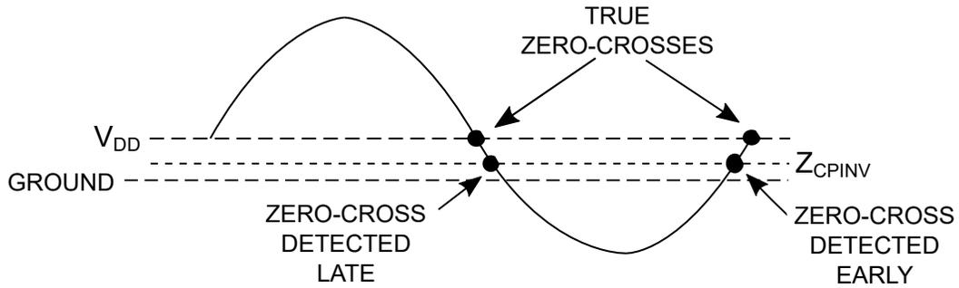
The actual offset time can be determined for sinusoidal waveforms of a known frequency  $f$  using the equations shown below.
