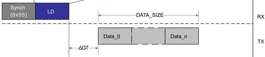
The figure above shows an example of a typical LD sequence, where the data are received after the Guard Time (GT) period. Loading data from the UPDI Pointer register follows the same transmission protocol.
