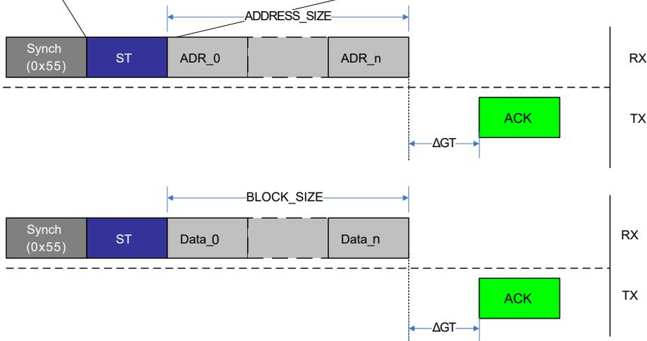
The figure above gives an example of an ST instruction to the UPDI Pointer register and the storage of regular data. A SYNCH character is sent before each instruction. In both cases, an Acknowledge (ACK) is sent back by the UPDI if the ST instruction was successful.
