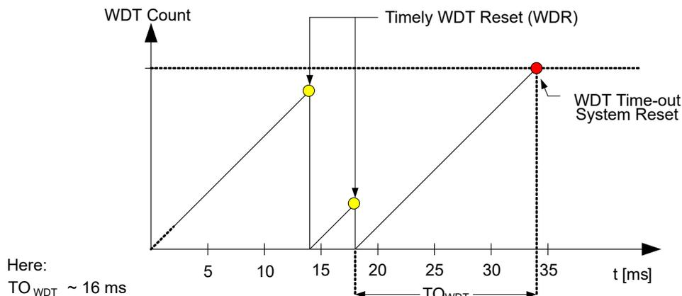
The Normal mode is enabled as long as the Window (WINDOW) bit field in the WDT.CTRLA register is '0x0'.
