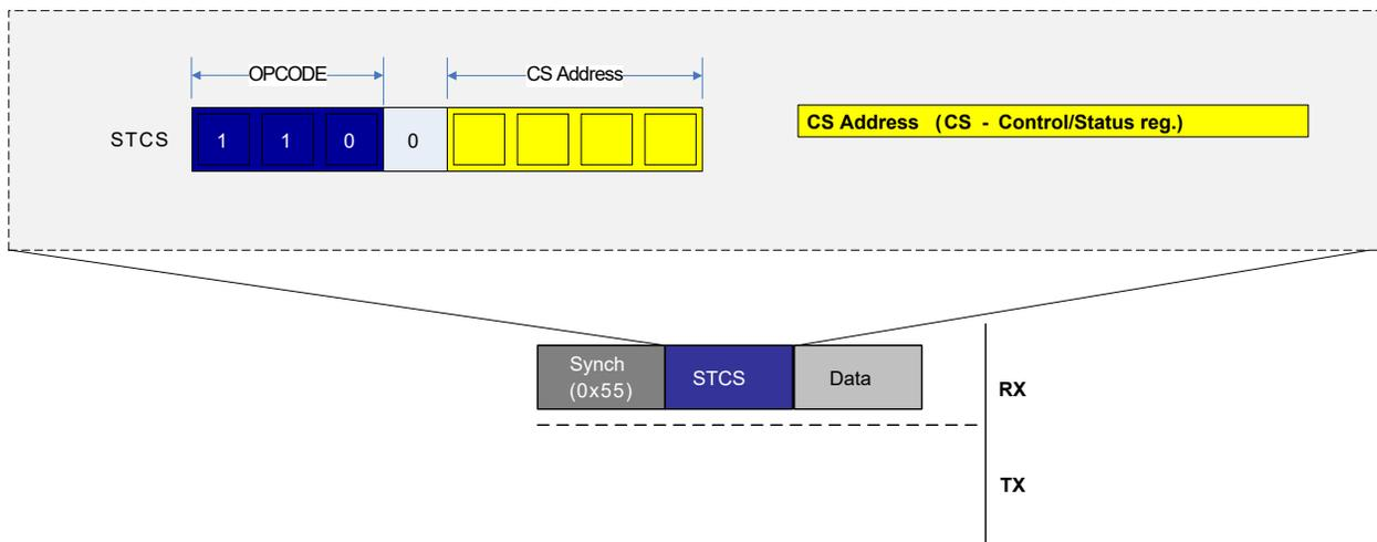
The figure above shows the data frame transmitted after the SYNCH character and the instruction frames. The STCS instruction byte can be immediately followed by the data byte. There is no response generated from the STCS instruction, as is the case for the ST and STS instructions.
