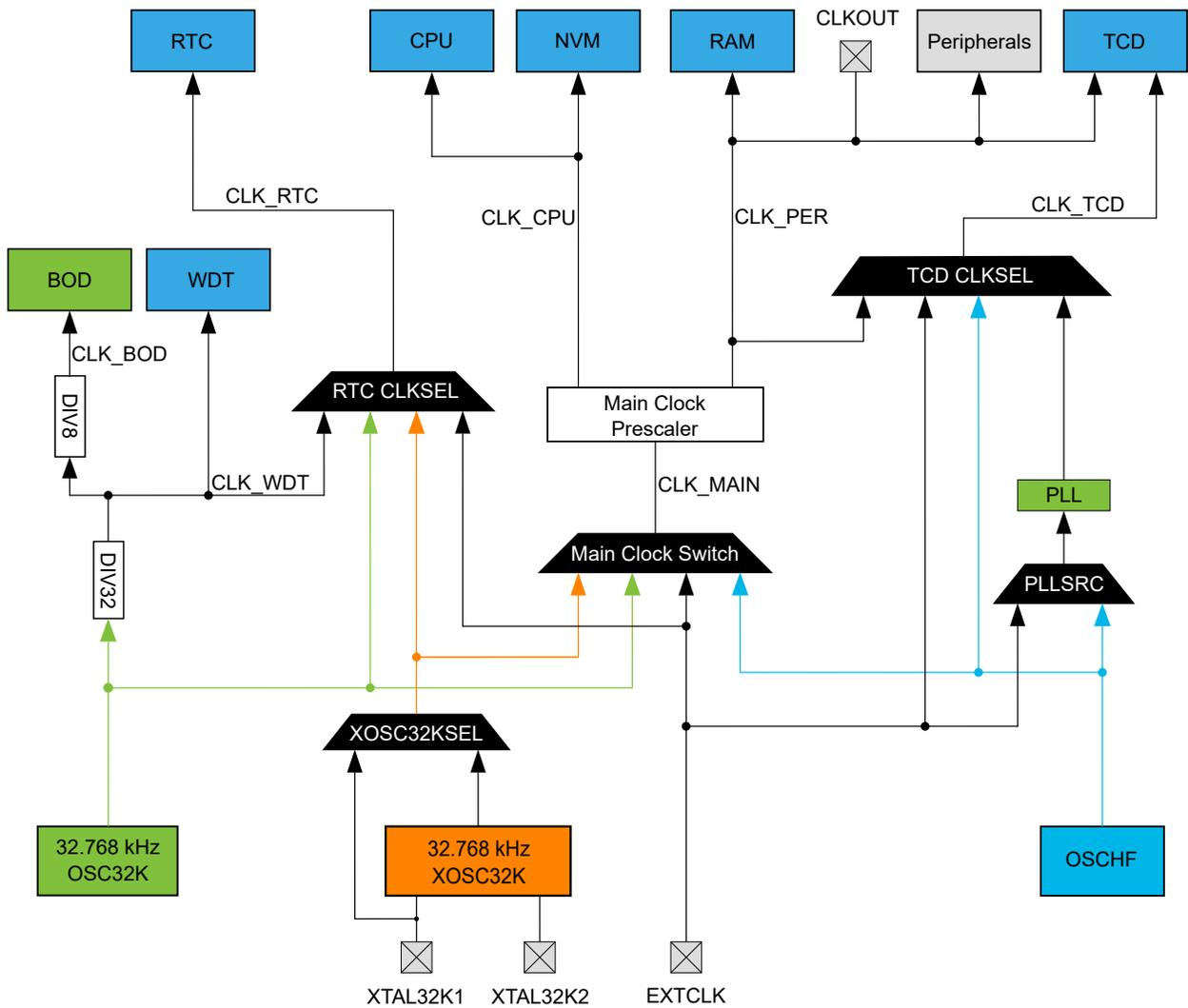
The clock system consists of the main clock and clocks derived from the main clock, as well as several asynchronous clocks:
