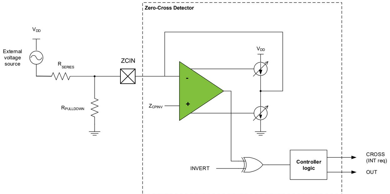
The resistor adds a bias to the ZCD input pin so that the external voltage source must go to zero to pull the pin voltage to the  $Z_{CPINV}$  switching voltage. The pull-up or pull-down value can be determined with the equations shown below.
