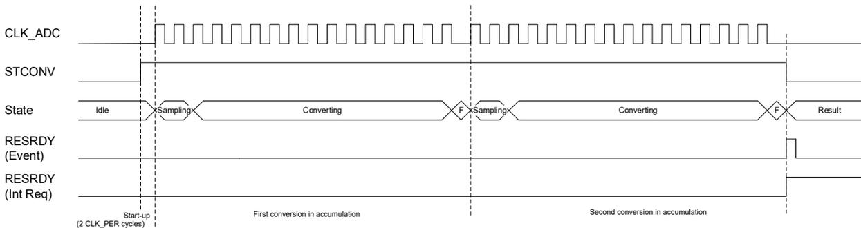
The number of samples to accumulate is configured with the Sample Number (SAMPNUM) bit field in the Control B (ADCn.CTRLB) register. The STCONV bit is set for the entire conversion. The total conversion time for n samples is given by:
