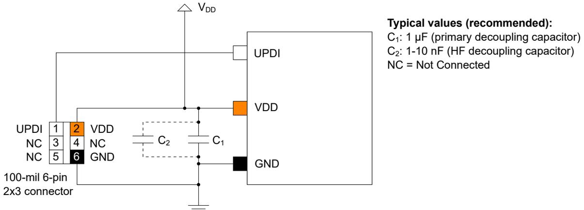
The decoupling capacitor between  $V_{DD}$  and GND should be placed as close to the pin pair as possible and should be included even if the UPDI connector is not included in the circuit.
