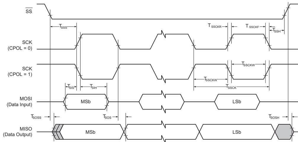
**Table 37-20. SPI - Timing Characteristics in Slave Mode**
