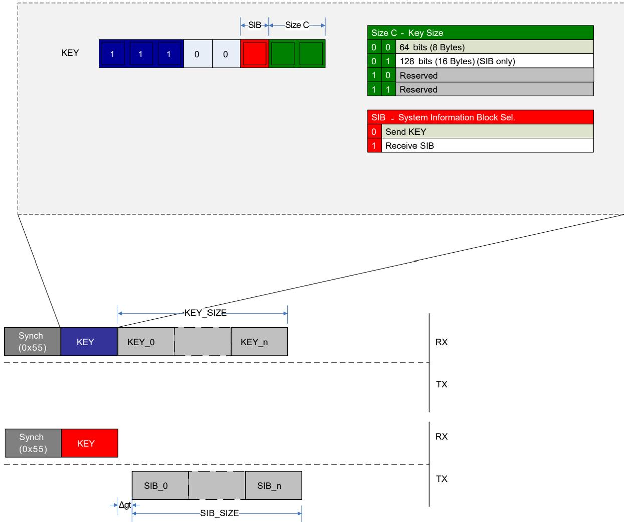
The figure above shows the transmission of a key and the reception of a SIB. In both cases, the Size C (*SIZE\_C*) field in the operand determines the number of frames being sent or received. There is no response after sending a *KEY* to the UPDI. When requesting the SIB, data will be transmitted from the UPDI according to the current guard time setting.
