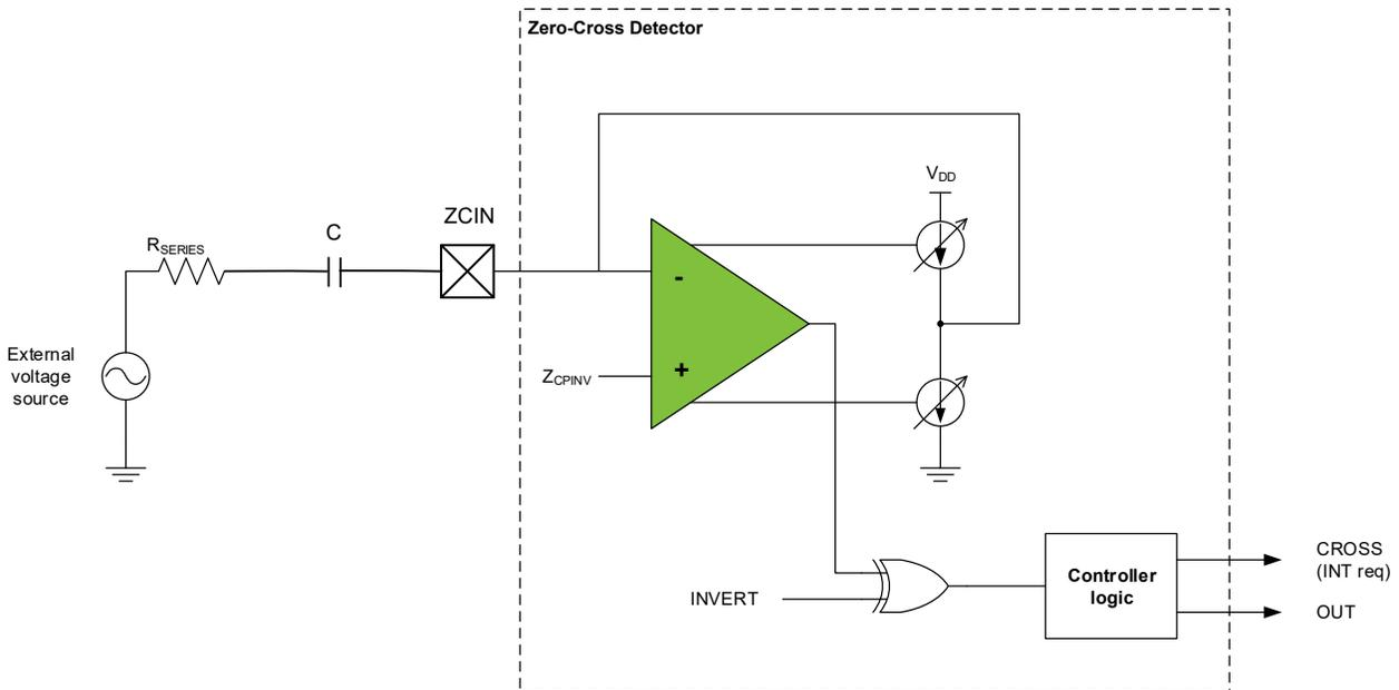
The phase shift resulting from the capacitor will cause the ZCD output to switch in advance of the actual zero-crossing event. The phase shift will be the same for both rising and falling zero-crossings, which can be compensated for by either delaying the CPU response to the ZCD switch by a timer or other means, or selecting a capacitor value large enough that the phase shift is negligible.
