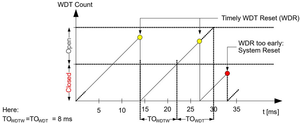
The Window mode is enabled by writing a non-zero value to the Window (WINDOW) bit field in the Control A (WDT.CTRLA) register. The Window mode is disabled by writing the WINDOW bit field to '0x0'.
