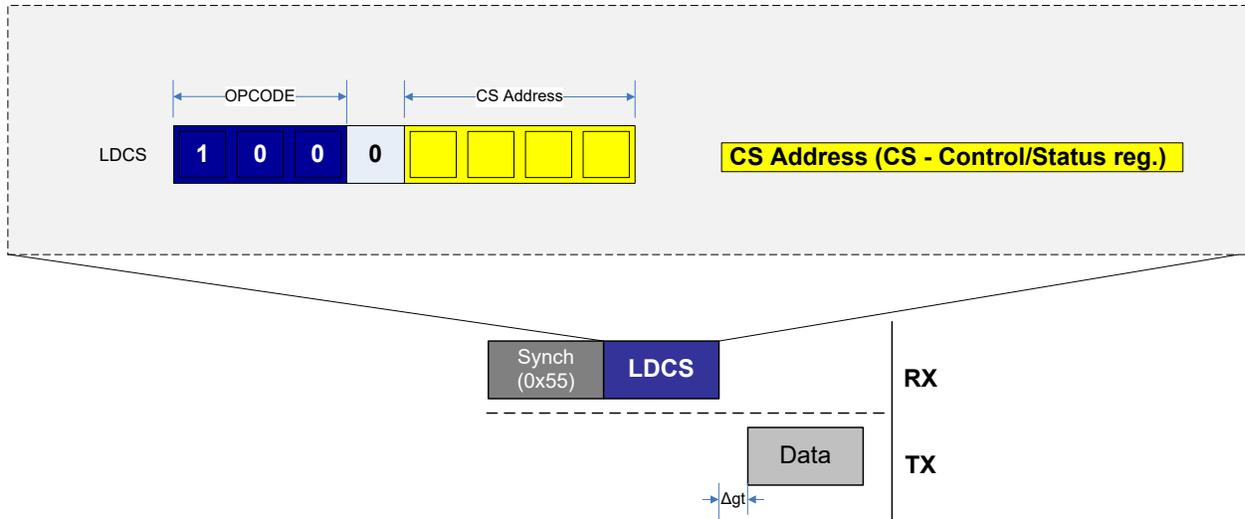
The figure above shows a typical example of `LDCS` data transmission. A data byte from the `LDCS` is transmitted from the UPDI after the guard time is completed.
