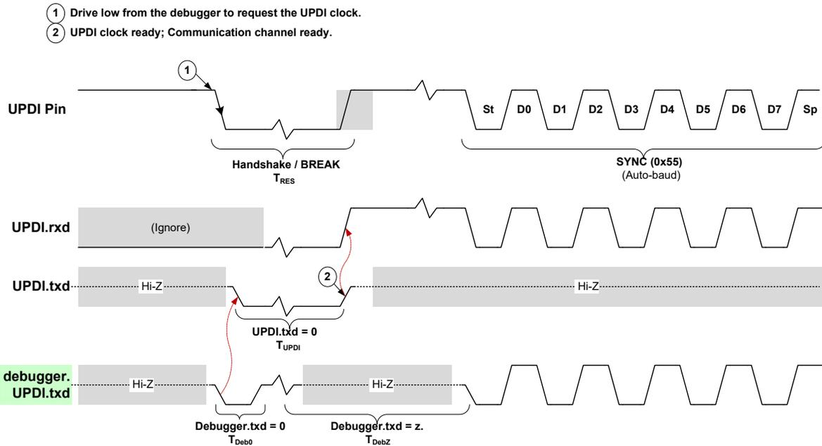
To avoid the UPDI from staying enabled if an accidental trigger of the edge detector happens, the UPDI will automatically disable itself and lower its clock request. See the *Disable During Start-up* section for more details.
