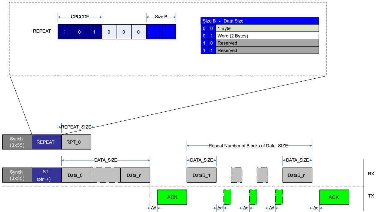
The figure above gives an example of repeat operation with an ST instruction using pointer post-increment operation. After the REPEAT instruction is sent with  $RPT\_0 = n$ , the first ST instruction is issued with SYNCH and instruction frame, while the next n ST instructions are executed by only sending data bytes according to the ST operand DATA\_SIZE, and maintaining the Acknowledge (ACK) handshake protocol.
