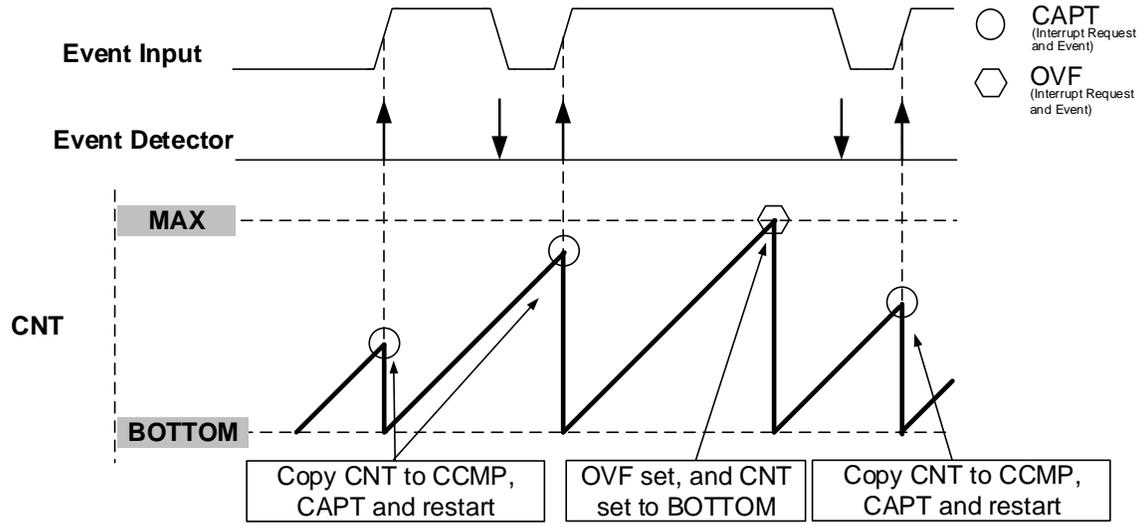
22.3.3.1.5 Input Capture Pulse-Width Measurement Mode
