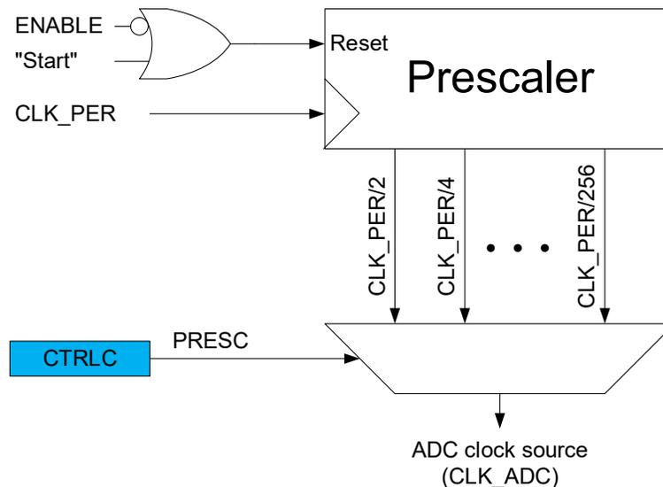
When initiating a conversion by writing a '1' to the Start Conversion (STCONV) bit in the ADCn.COMMAND register or from event, the conversion starts after one CLK\_PER cycle. The prescaler is kept in Reset, as long as there is no ongoing conversion. This assures a fixed delay from the trigger to the actual start of a conversion of maximum 2 CLK\_PER cycles.
