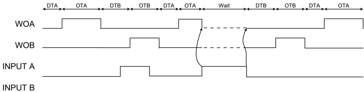
If Input mode 1 is used on input B, an event will only have an effect if the TCD is in dead time B or on time B, and it will only affect the WOB output. When the event is done, the TCD counter starts at dead time A.
