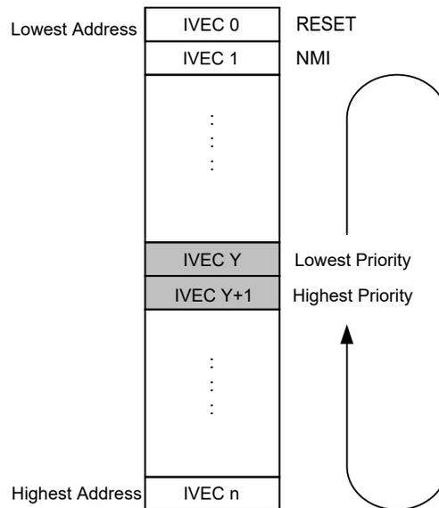
Here, value Y has been written to CPUINT.LVL0PRI, so that interrupt vector Y+1 has the highest priority. Note that, in this case, the priorities will wrap so that the lowest address no longer has the highest priority. This does not include RESET and NMI, which will always have the highest priority.
