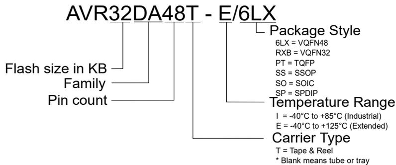
**Note:** The Tape and Reel identifier only appears in the catalog part number description. This identifier is used for ordering purposes and is not printed on the device package. Check with your [Microchip Sales Office](#) for package availability with the Tape and Reel option.
