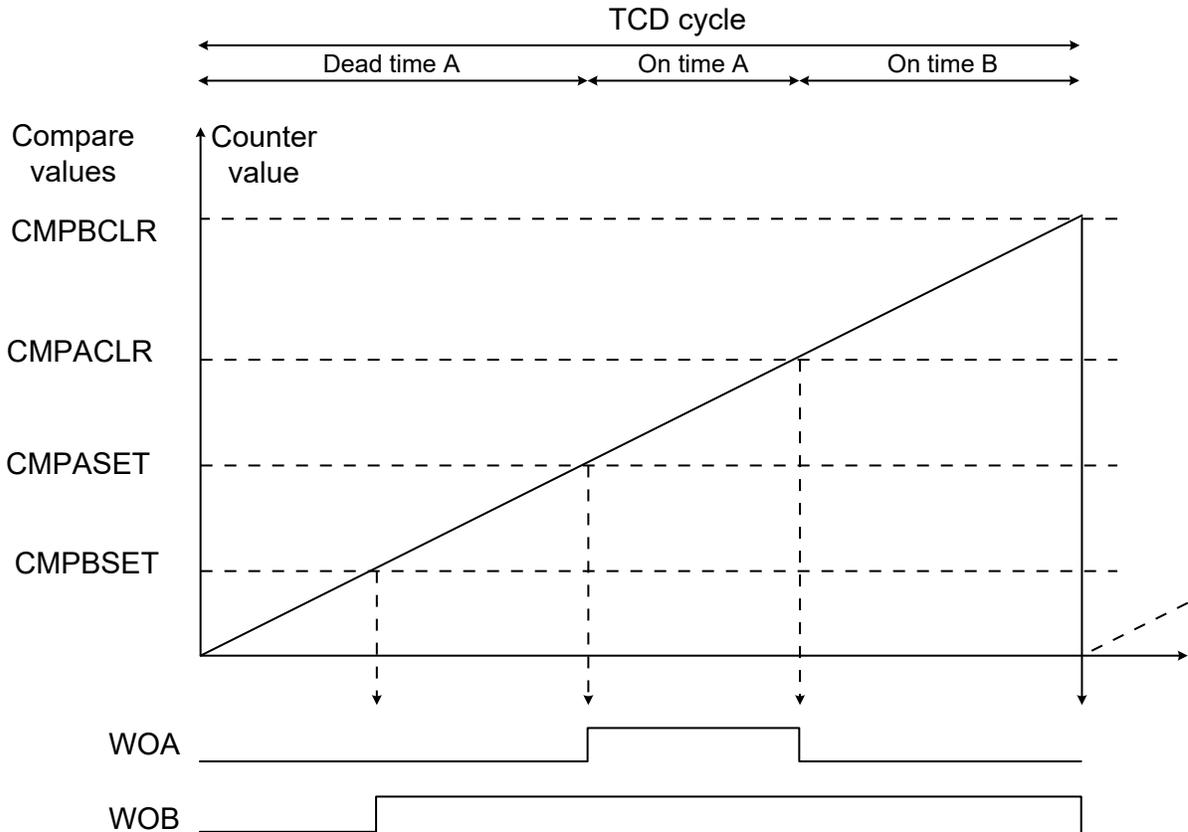
A match with CMPBCLR will always result in all outputs being cleared. If any of the other compare values are bigger than CMPBCLR, their associated effect will never occur. If the CMPACL is smaller than the CMPASET value, the clear value will not have any effect.
