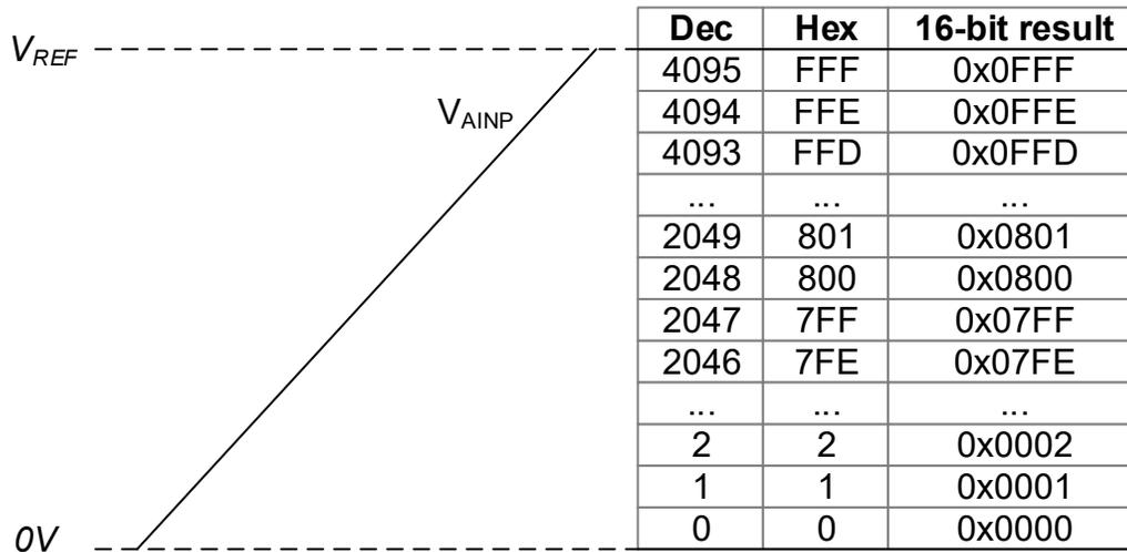
Where  $V_{AINP}$  is the single-ended or internal input.
