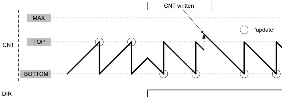
It is possible to change the counter value in the Counter (TCAn.CNT) register when the counter is running. The write access to TCAn.CNT has higher priority than count, clear or reload, and will be immediate. The direction of the counter can also be changed during normal operation by writing to DIR in TCAn.CTRLE.
