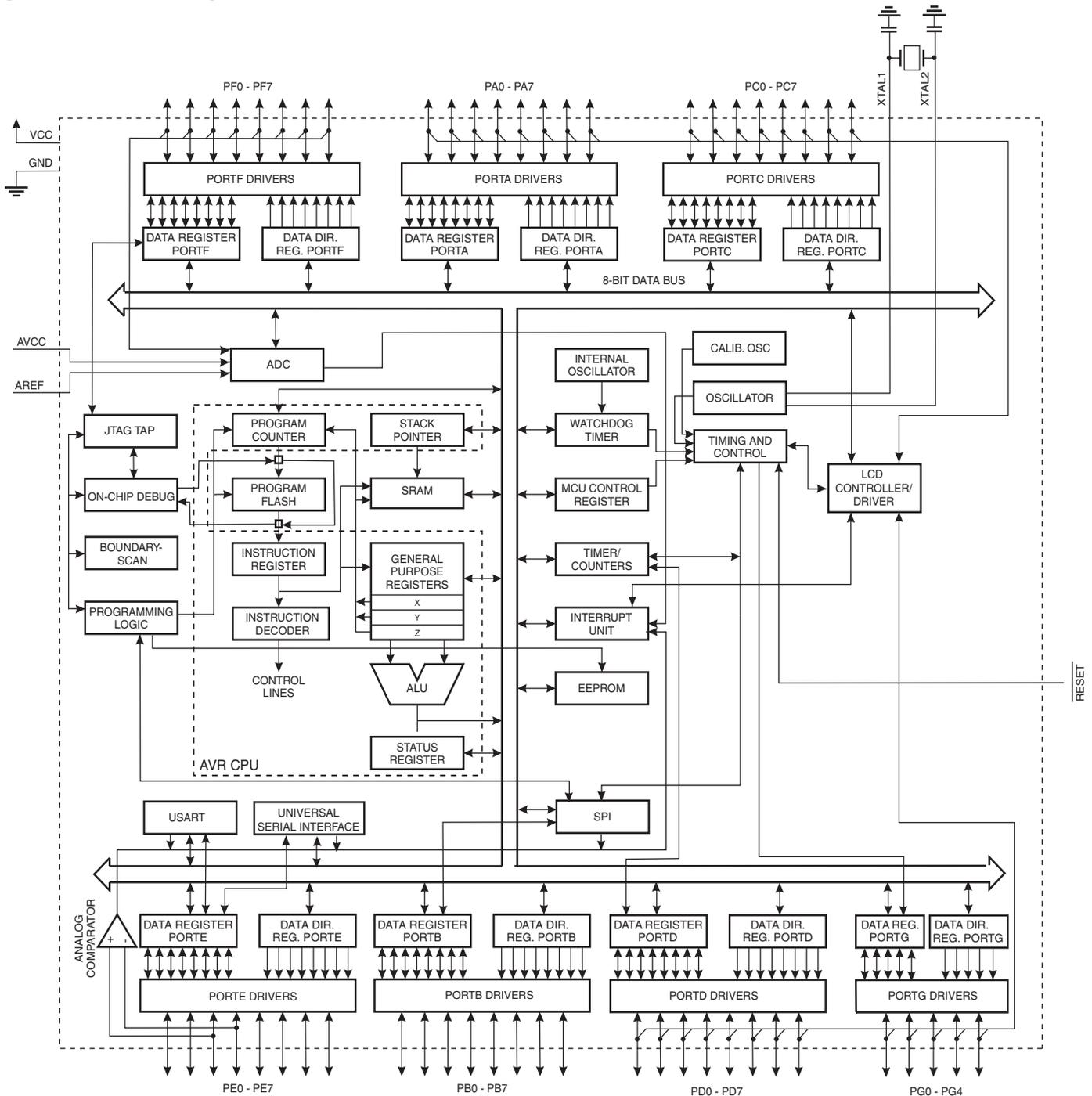
The AVR core combines a rich instruction set with 32 general purpose working registers. All the 32 registers are directly connected to the Arithmetic Logic Unit (ALU), allowing two independent registers to be accessed in one single instruction executed in one clock cycle. The resulting architecture is more code efficient while achieving throughputs up to ten times faster than conventional CISC microcontrollers.
