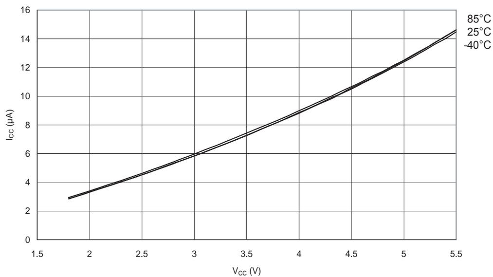
**Figure 29-62.** Analog Comparator Current vs.  $V_{CC}$
