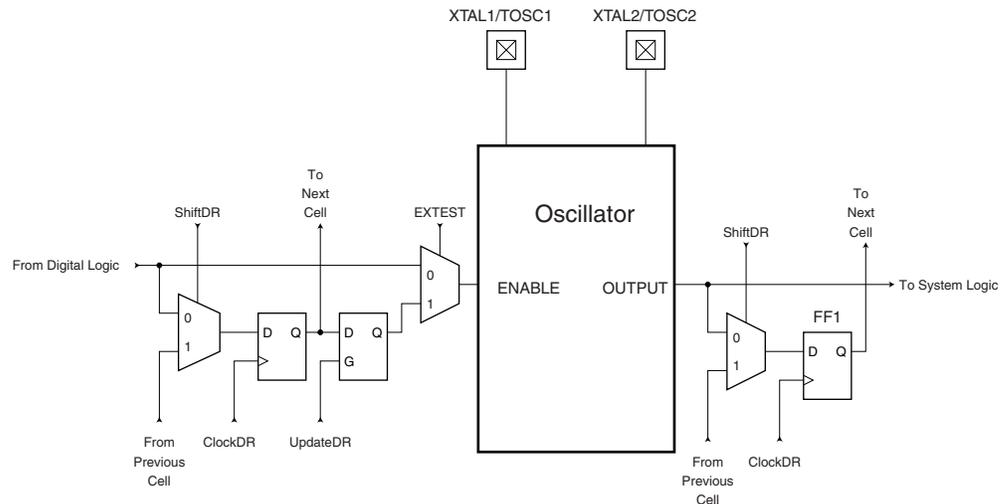
Table 25-1 summarizes the scan registers for the external clock pin XTAL1, oscillators with XTAL1/XTAL2 connections as well as 32 kHz Timer Oscillator.
