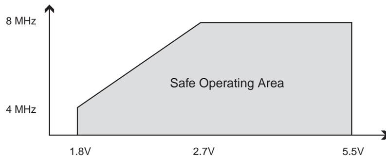
**Figure 28-2.** Maximum Frequency vs.  $V_{CC}$ , ATmega169P
