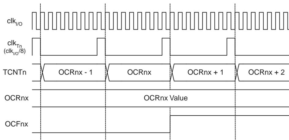
Figure 17-11 shows the setting of OCF2A and the clearing of TCNT2 in CTC mode.
