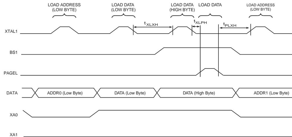
Note: 1. The timing requirements shown in [Figure 27-7 on page 308](#) (that is,  $t_{DVXH}$ ,  $t_{XHXL}$ , and  $t_{XLDX}$ ) also apply to loading operation.
