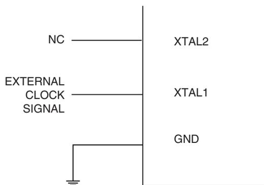
When this clock source is selected, start-up times are determined by the SUT Fuses as shown in [Table 8-12](#).
