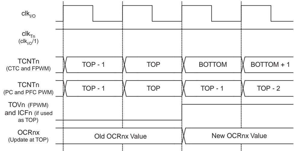
Figure 15-13 shows the same timing data, but with the prescaler enabled.
