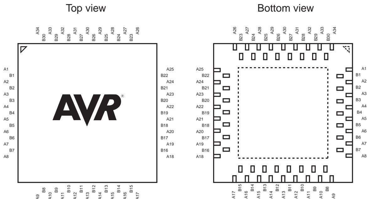
Table 1-1. DRQFN-64 Pinout ATmega169P.
