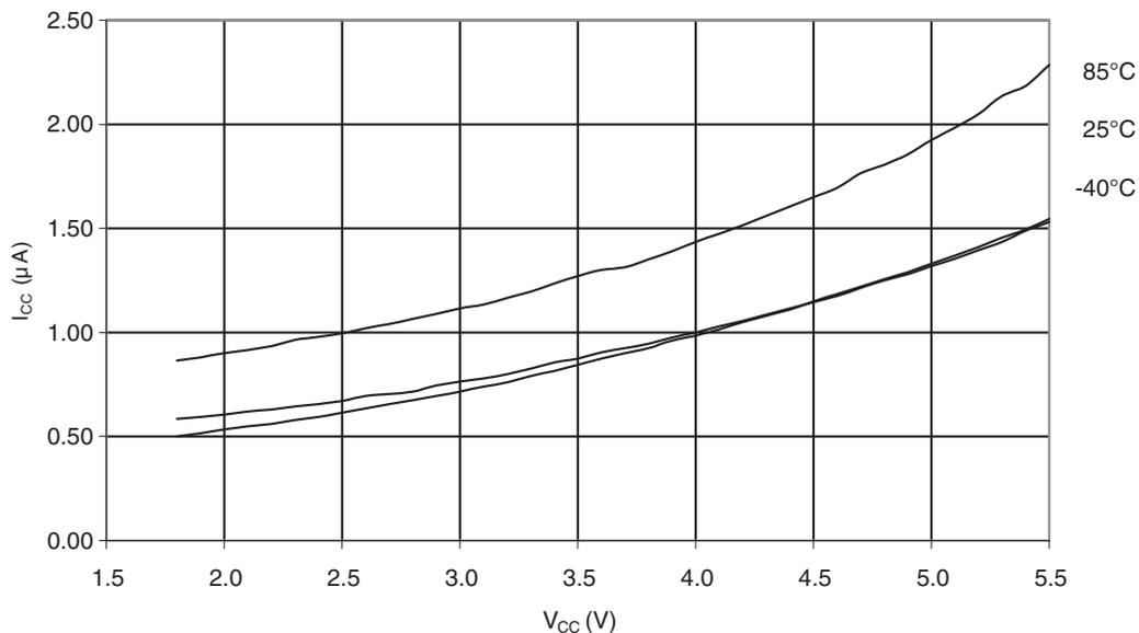
Figure 29-15. Standby Supply Current vs.  $V_{CC}$  (455 kHz Resonator, Watchdog Timer Disabled)
