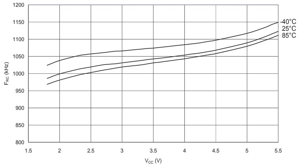
**Figure 29-55.** Calibrated 8 MHz RC Oscillator Frequency vs. Temperature
