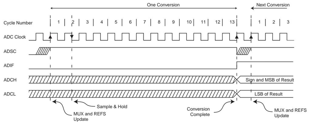
**Figure 22-6.** ADC Timing Diagram, Auto Triggered Conversion
