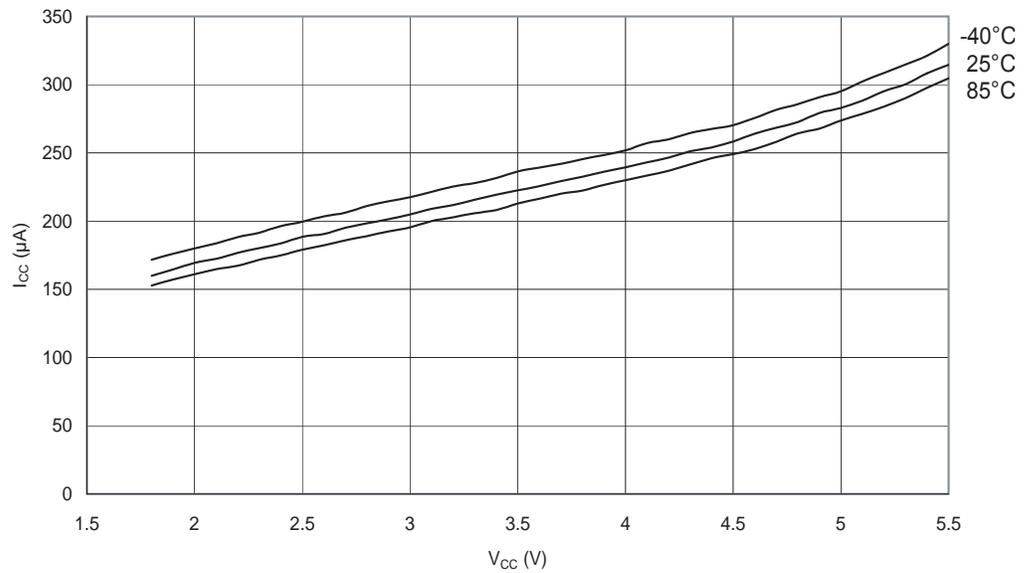
**Figure 29-60.** AREF External Reference Current vs.  $V_{CC}$
