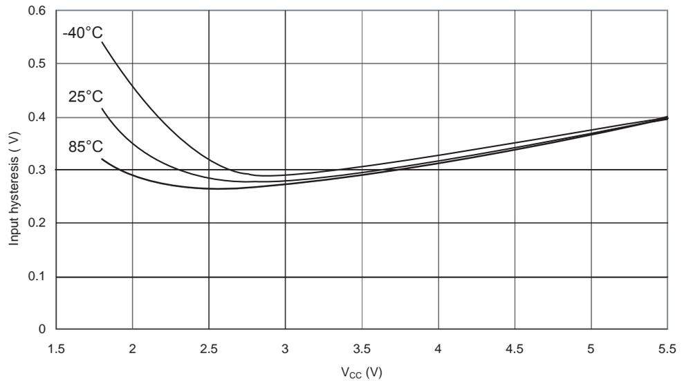
**Figure 29-44.** Reset Input Threshold Voltage vs.  $V_{CC}$  ( $V_{IH}$ , Reset Pin Read as "1")
