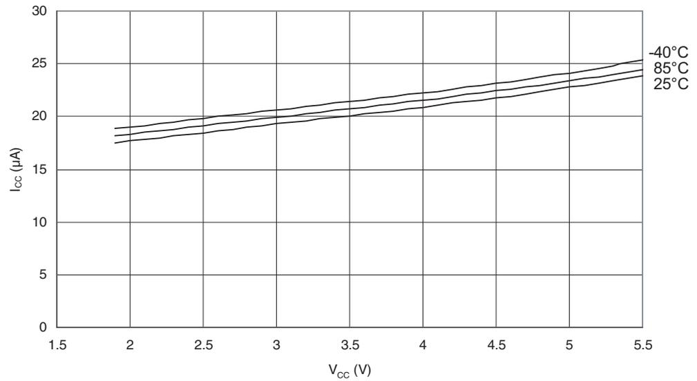
Figure 29-59. ADC Current vs.  $V_{CC}$  (AREF = AVCC)
