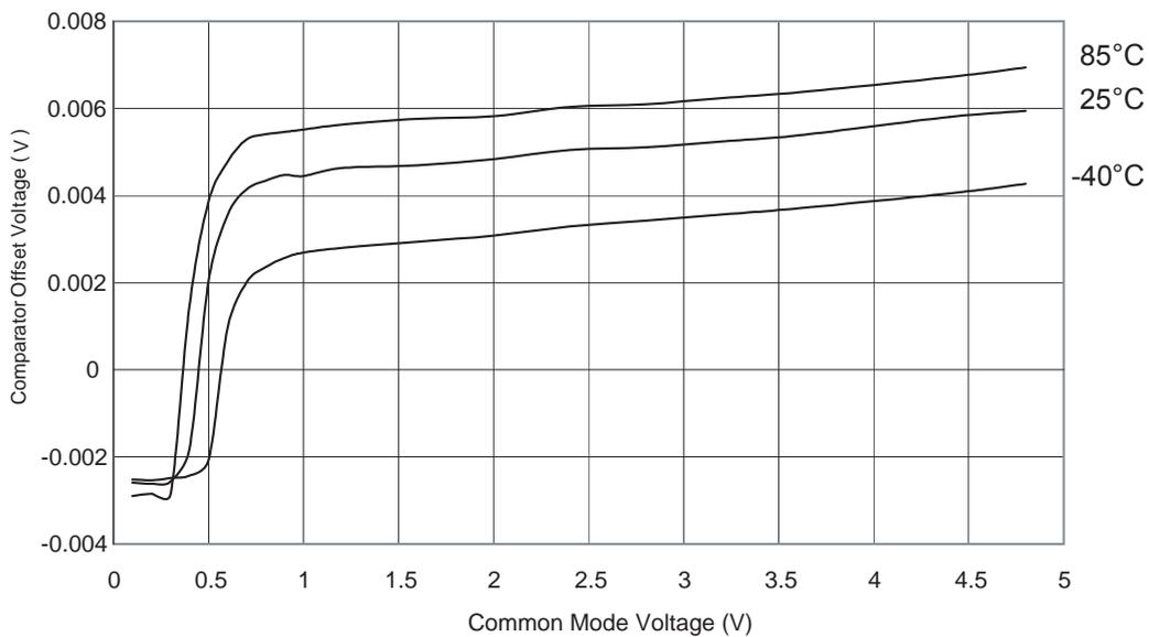
**Figure 29-52.** Analog Comparator Offset Voltage vs. Common Mode Voltage ( $V_{CC} = 2.7V$ )
