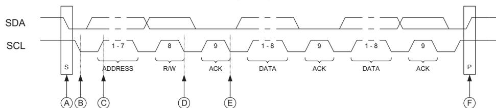
Referring to the timing diagram (Figure 20-5), a bus transfer involves the following steps:
