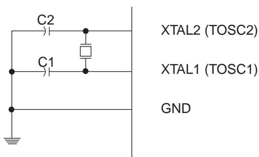
The Oscillator can operate in three different modes, each optimized for a specific frequency range. The operating mode is selected by the fuses CKSEL3:1 as shown in Table 8-5.
