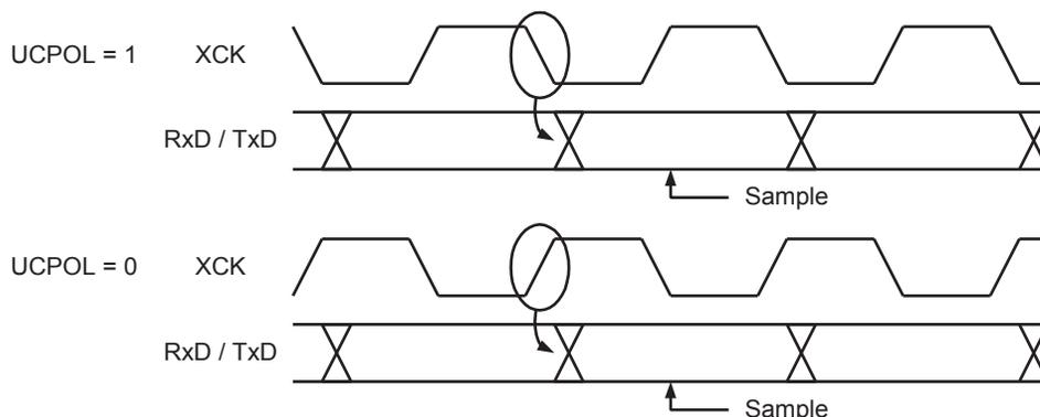
The  $UCPOLn$  bit  $UCRSC$  selects which XCK clock edge is used for data sampling and which is used for data change. As [Figure 19-3](#) shows, when  $UCPOLn$  is zero the data will be changed at rising XCK edge and sampled at falling XCK edge. If  $UCPOLn$  is set, the data will be changed at falling XCK edge and sampled at rising XCK edge.
