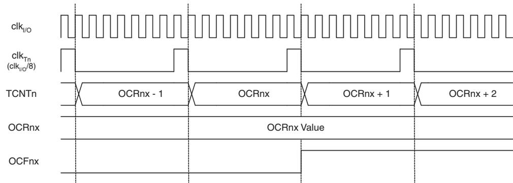
Figure 14-11 shows the setting of OCF0A and the clearing of TCNT0 in CTC mode.
