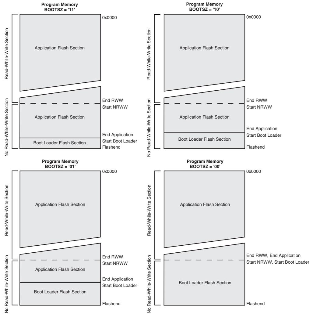
Note: 1. The parameters in the figure above are given in [Table 26-6 on page 292](#).
