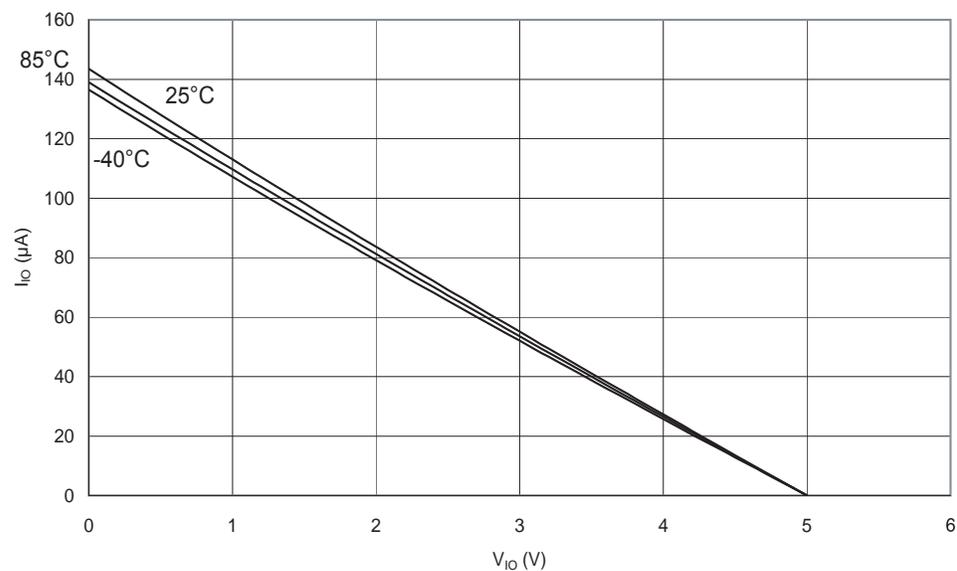
**Figure 29-24.** I/O Pin Pull-up Resistor Current vs. Input Voltage ( $V_{CC} = 2.7V$ )
