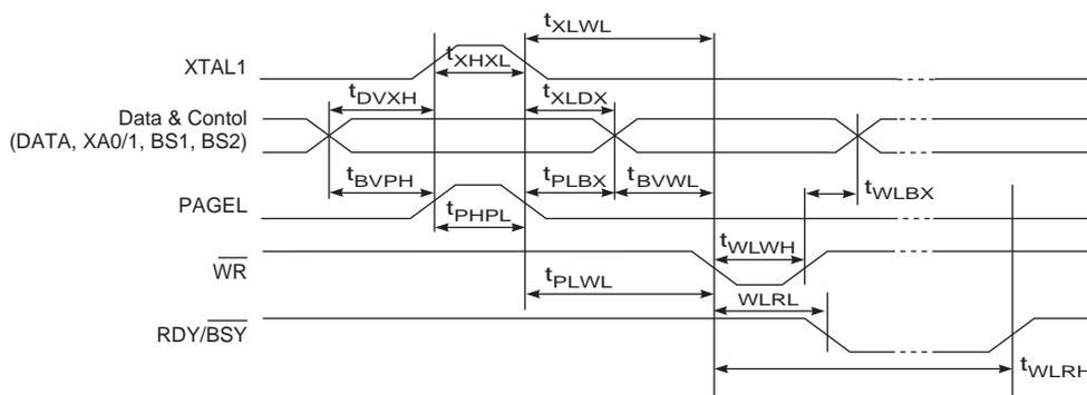
**Figure 27-8.** Parallel Programming Timing, Loading Sequence with Timing Requirements<sup>(1)</sup>
