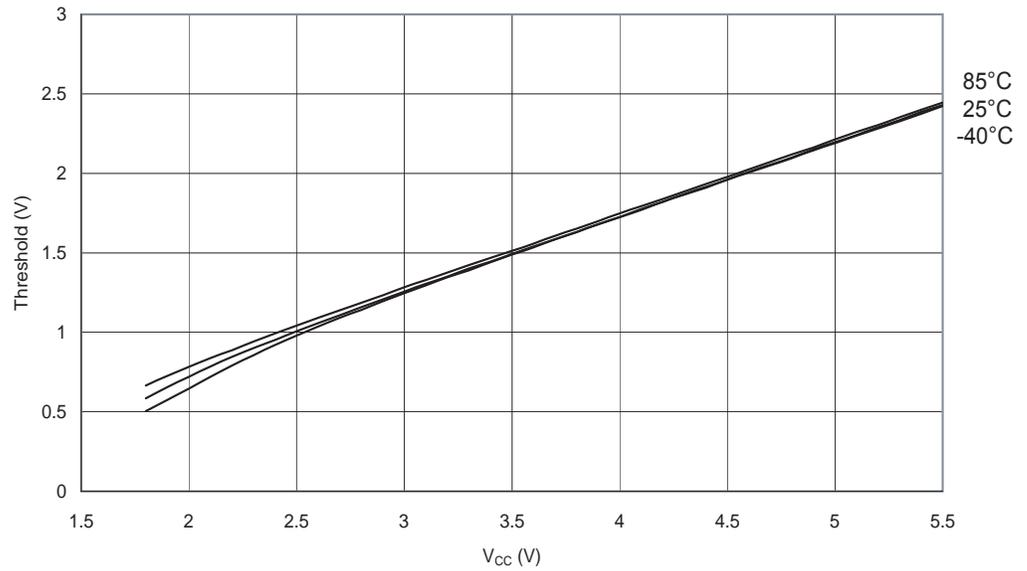
**Figure 29-43.** I/O Pin Input Hysteresis vs.  $V_{CC}$
