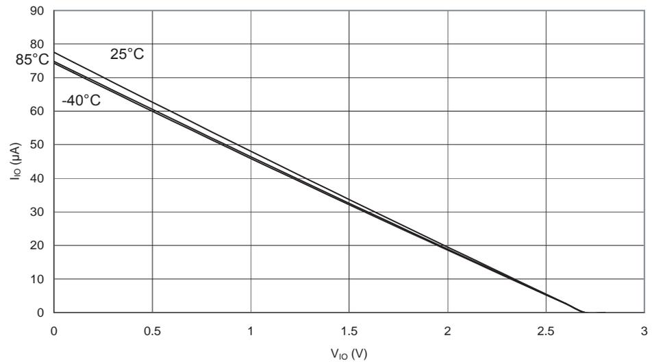
**Figure 29-25.** I/O Pin Pull-up Resistor Current vs. Input Voltage ( $V_{CC} = 1.8V$ )
