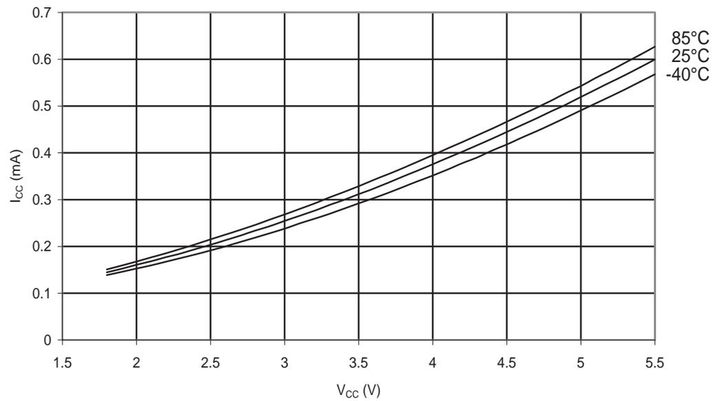
**Figure 29-10.** Idle Supply Current vs.  $V_{CC}$  (32 kHz Watch Crystal)
