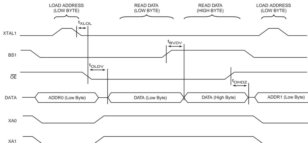
Note: 1. The timing requirements shown in [Figure 27-7 on page 308](#) (that is,  $t_{DVXH}$ ,  $t_{XHXL}$ , and  $t_{XLDX}$ ) also apply to reading operation.
