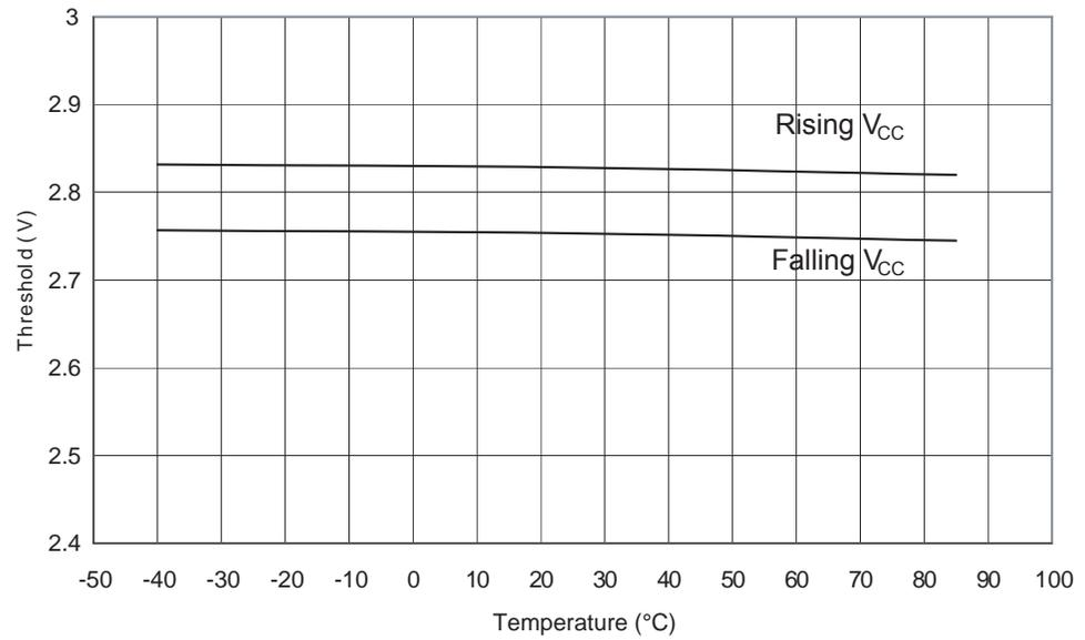
**Figure 29-49.** BOD Thresholds vs. Temperature (BOD Level is 1.8V)
