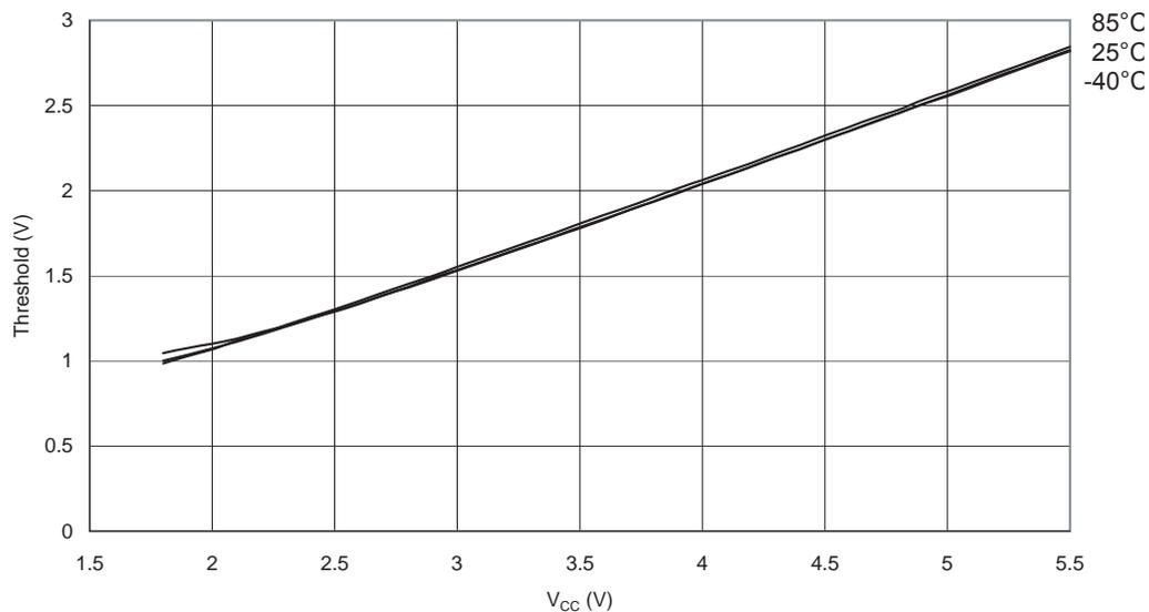
**Figure 29-42.** I/O Pin Input Threshold Voltage vs.  $V_{CC}$  ( $V_{IL}$ , I/O Pin Read as "0")
