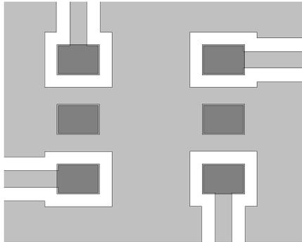
7. Recommended PCB layout shown above uses 1.6 mm FR4, rounded coplanar wave guide, transmission line width 0.70 mm and gap 0.57 mm.
