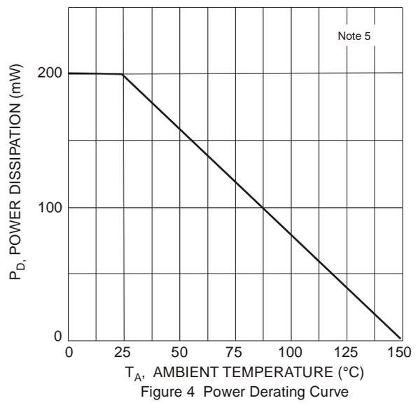
Note: 5. Part mounted on FR-4 board with recommended pad layout, which can be found on our website at <http://www.diodes.com/package-outlines.html>.
