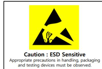
Proper ESD procedures should be followed when handling the device.
