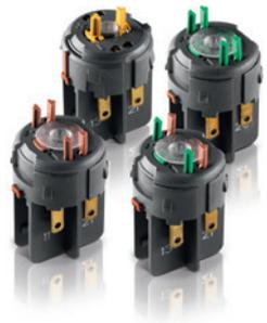
QC contact blocks can be easily snapped into the actuators without tools. Male quick-connect terminals are used directly for wiring in a conventional manner. This is a fast and efficient variant for applications where a printed circuit board is not cost-effective.
