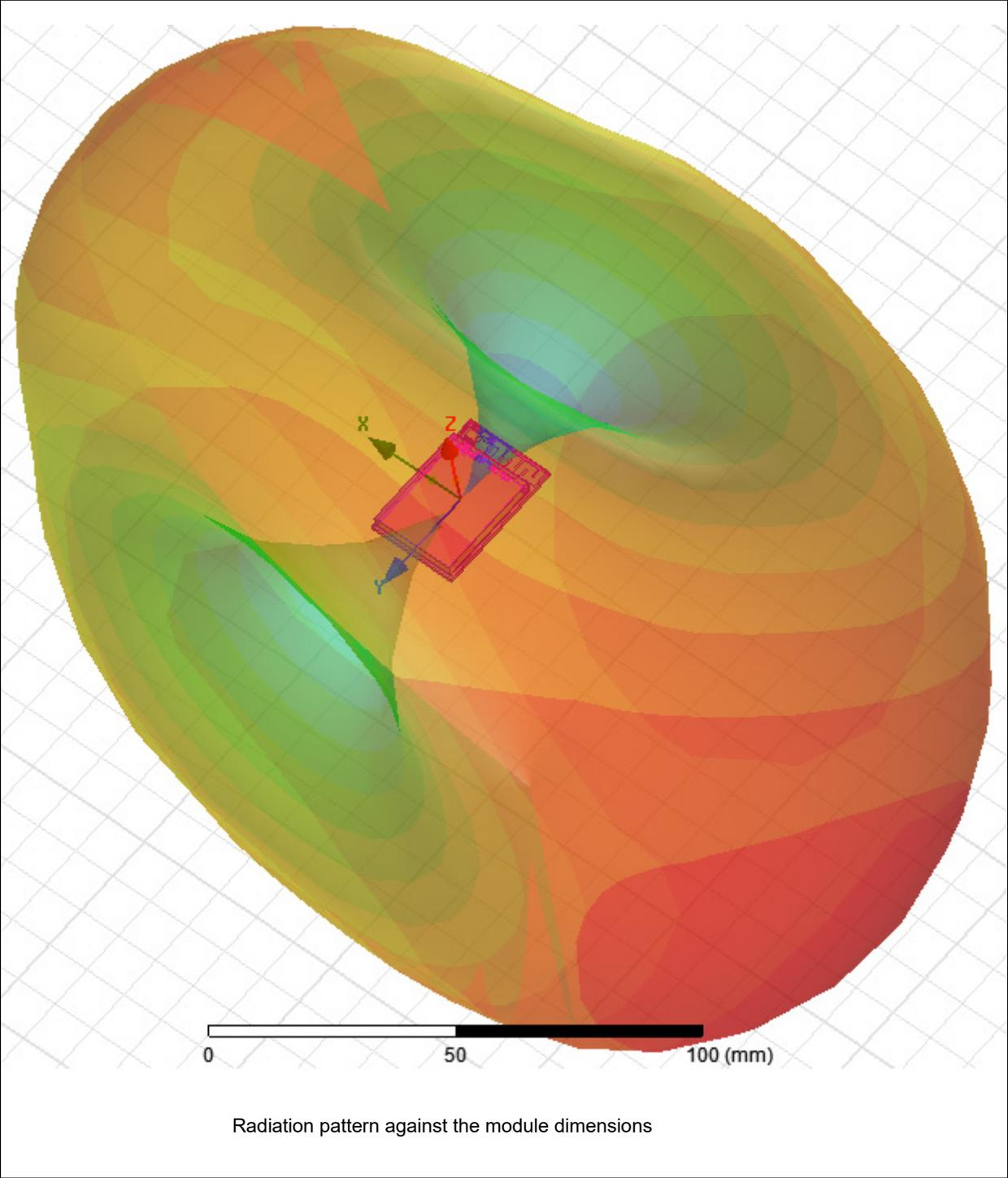
FIGURE 2-7: SIMULATED THREE-DIMENSIONAL RADIATION PATTERN
