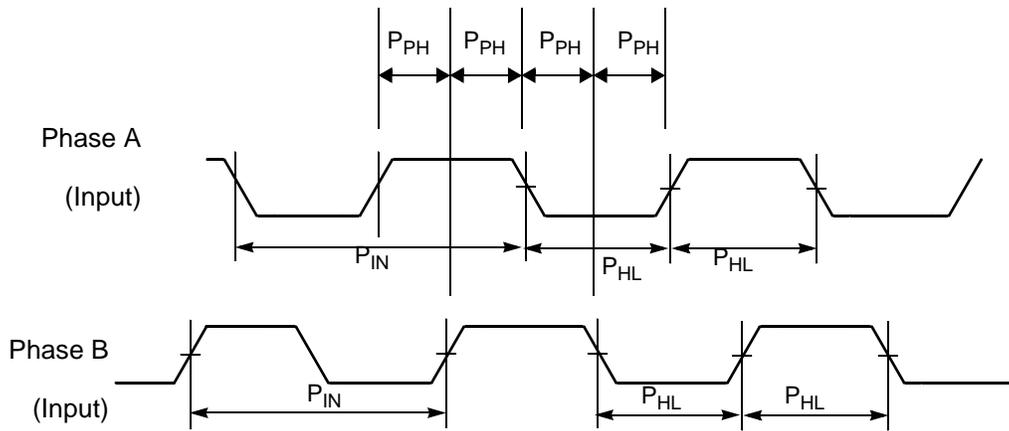
**Figure 3-24 Quadrature Decoder Timing**
