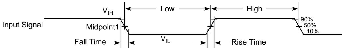
Note: The midpoint is  $V_{IL} + (V_{IH} - V_{IL})/2$ .
