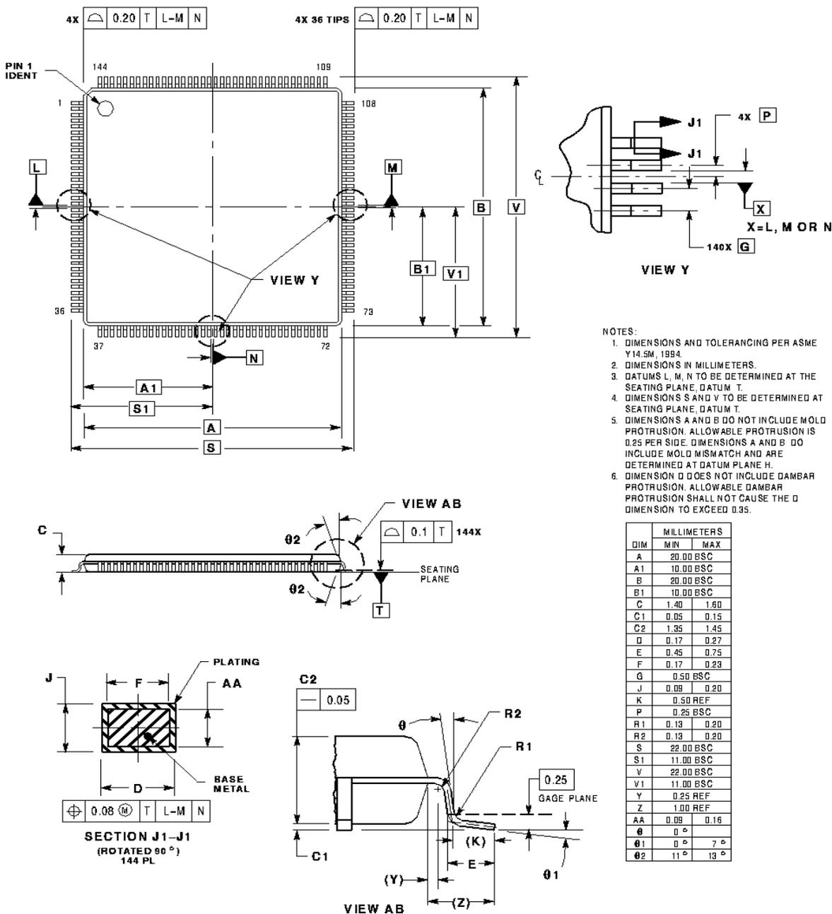
Figure 4-2 144-pin LQFP Mechanical Information
