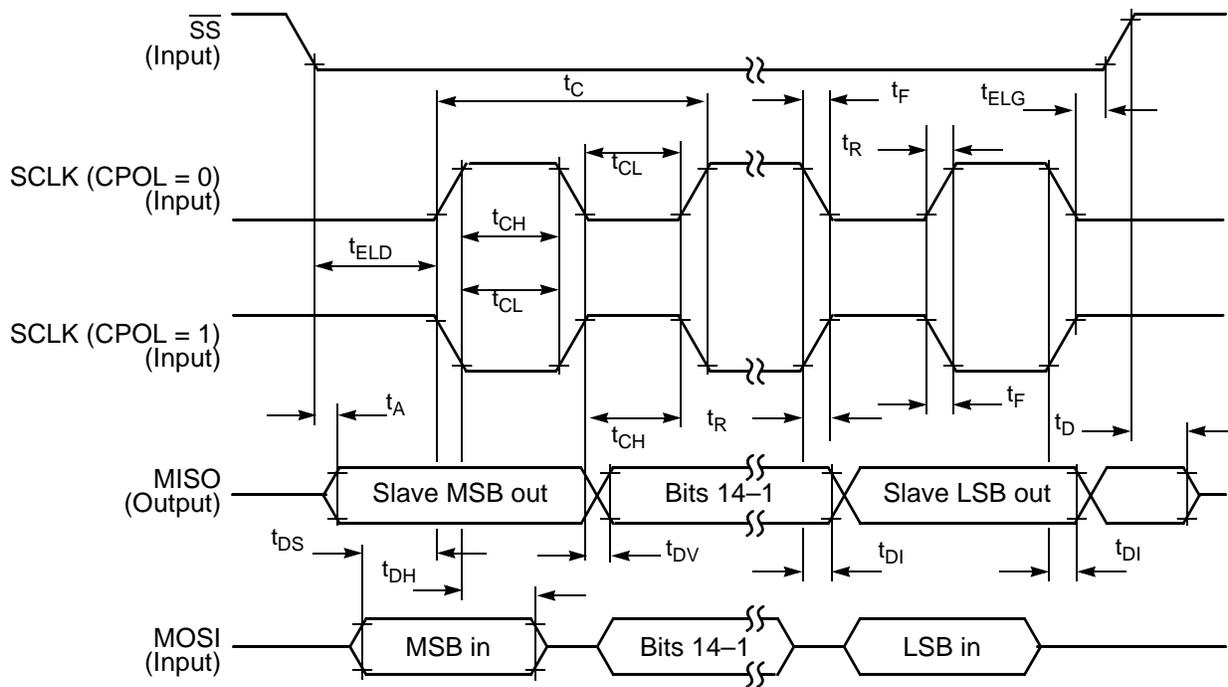
**Figure 3-21 SPI Slave Timing (CPHA = 0)**
