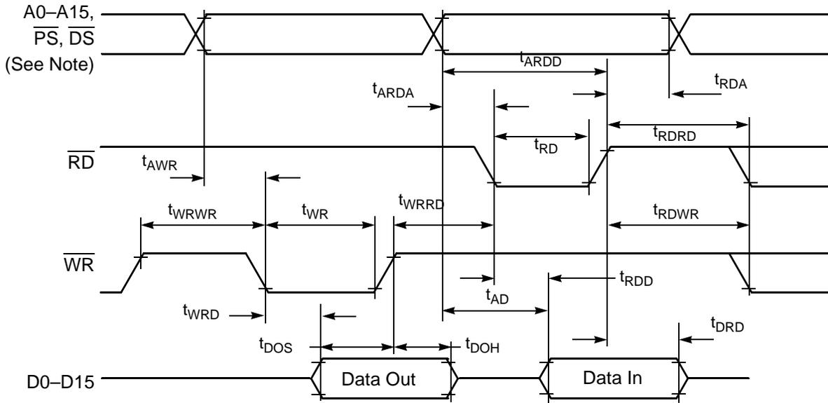
Note: During read-modify-write instructions and internal instructions, the address lines do not change state.
