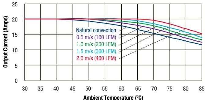
(Resistive loads 50% with +25% step Vin=48V)
