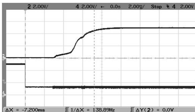
Enable Start-up (VIN=48V, Iout=12A, Cload=1000uF, Ta=+25°C)
