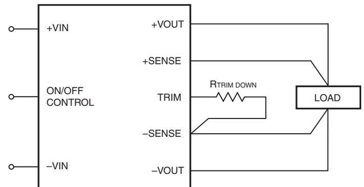
Figure 8. Trim Connections To Decrease Output Voltages
