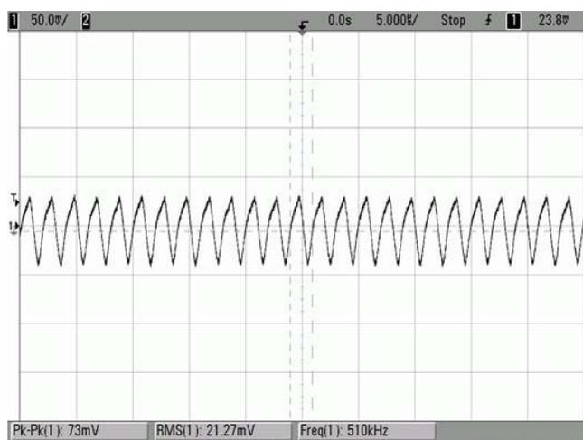
Output and Ripple Noise (Vin=48V, Iout=5A, 1uF Ceramic and 10uF tantalum capacitors)
