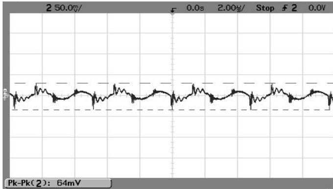
Output and Ripple Noise (Vin=48V, Iout=0A, 1uF Ceramic and 10uF tantalum capacitors)
