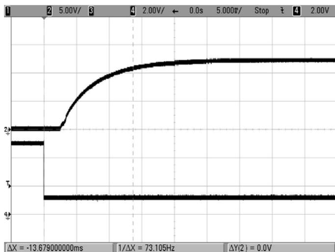
Enable Start-up (Vin=48V, Iout=0A, Ta=+25°C) Trace 2=Output, Trace 4= Enable.
