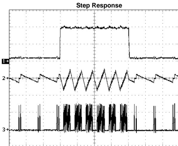
$V_{OUT} = 20V$ ,  $V_{IN} = 2.5V$
