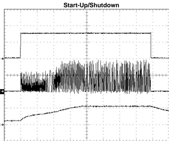
$V_{OUT} = 20V$ ,  $V_{IN} = 2.5V$
