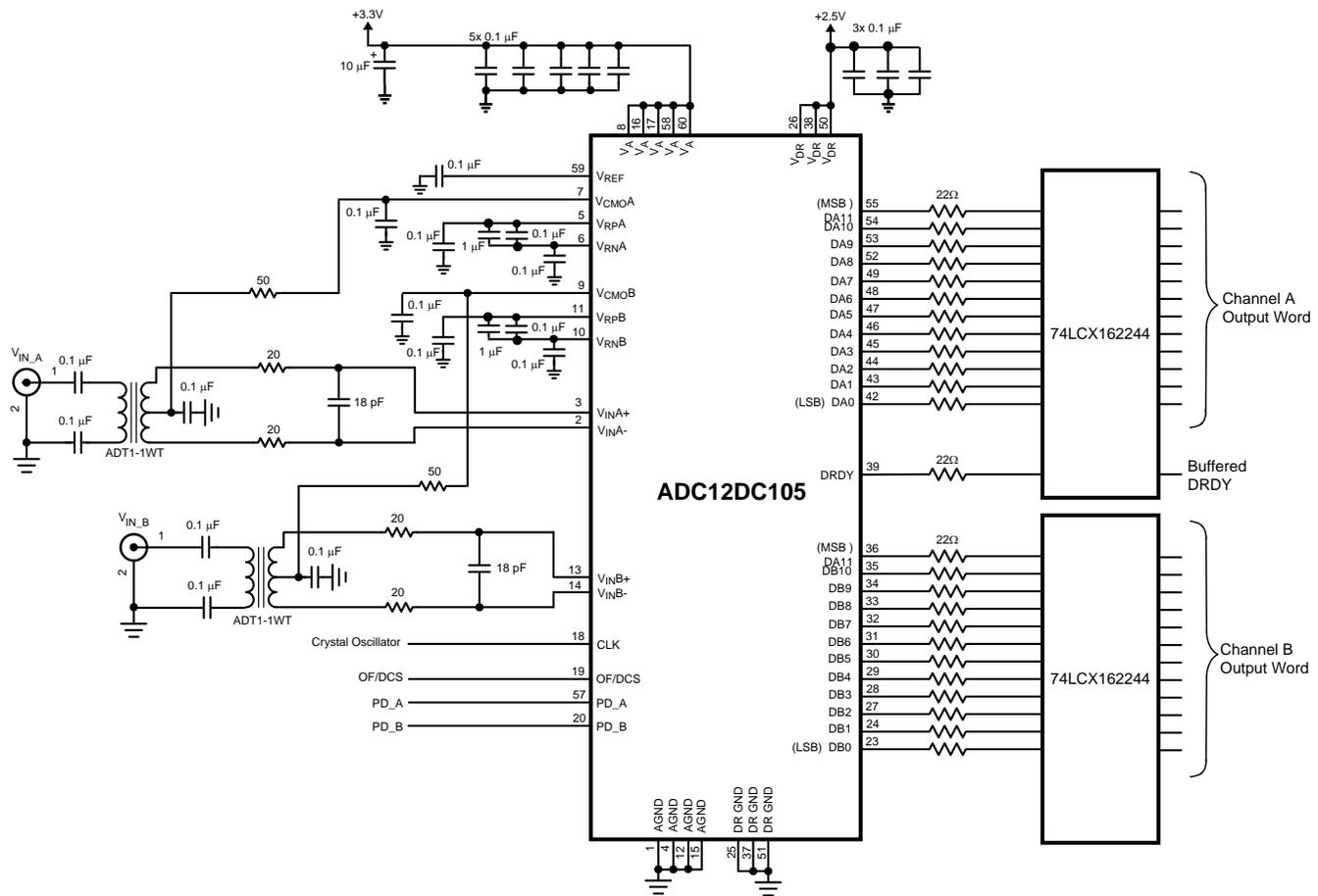
Figure 22. Application Circuit
