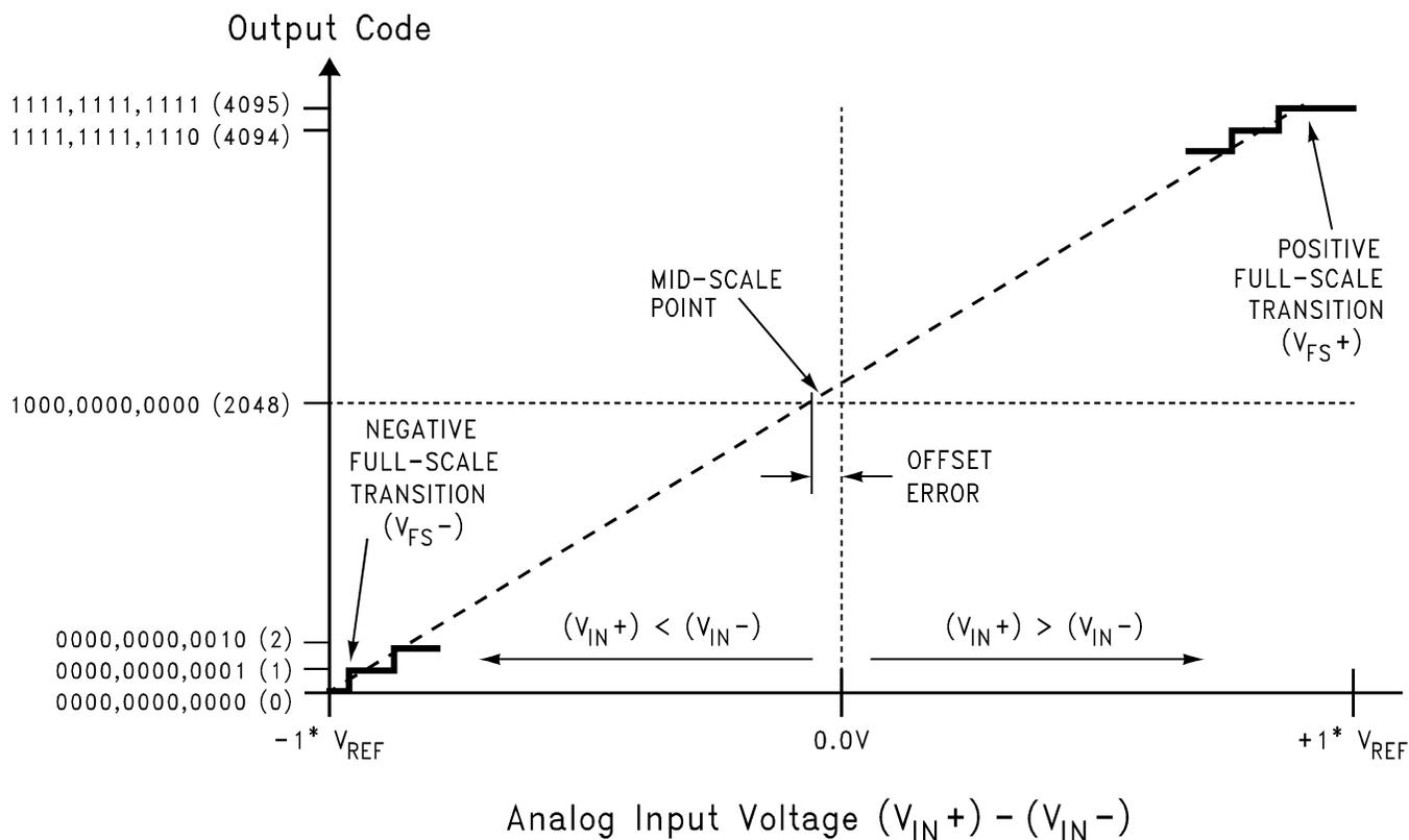
Figure 3. Transfer Characteristic
