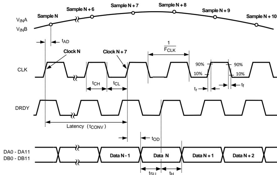
**Figure 2. Output Timing**
