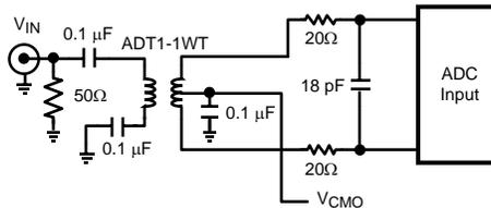
Figure 20. Low Input Frequency Transformer Drive Circuit
