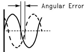
**Figure 19. Angular Errors Between the Two Input Signals Will Reduce the Output Level or Cause Distortion**
