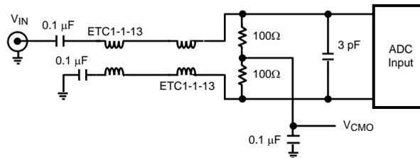
Figure 21. High Input Frequency Transformer Drive Circuit
